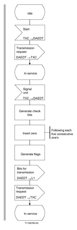
Figure 12/Q.703 – Delimitation, alignment and error detection (transmitting)
