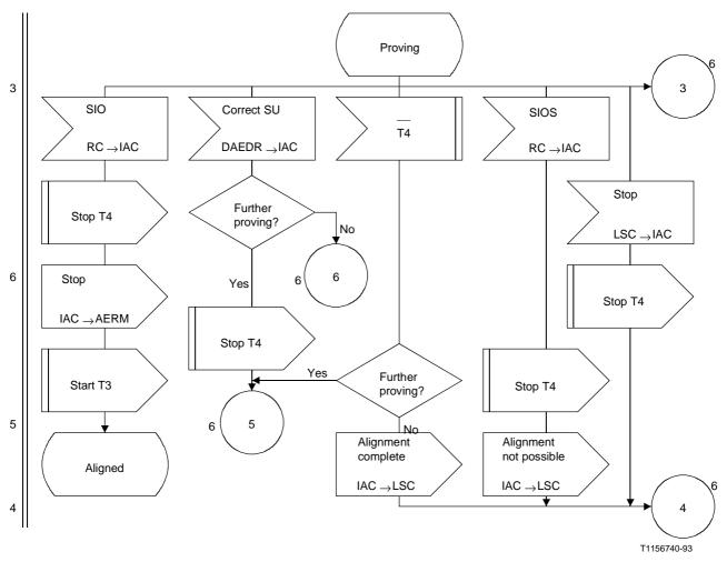
Figure 9/Q.703 (sheet 5 of 6) – Initial alignment control
