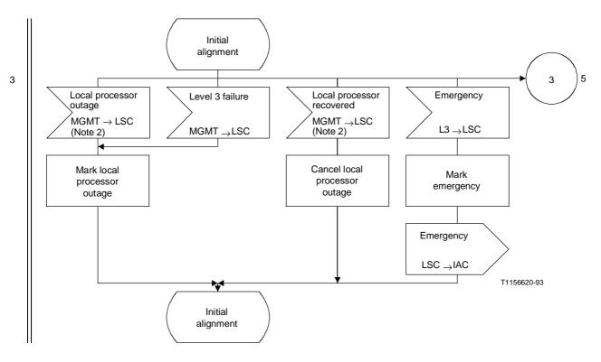
Figure 8/Q.703 (sheet 4 of 14) – Link state control
