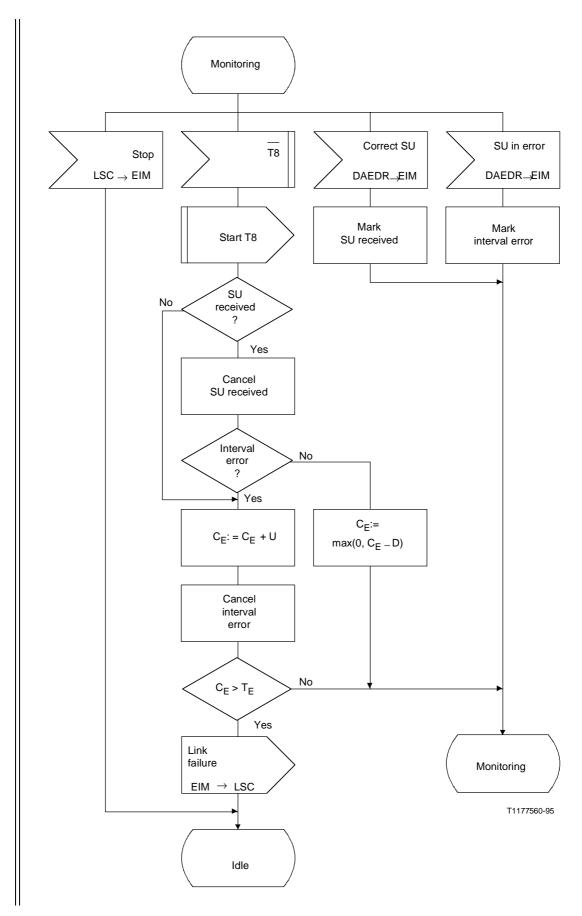
Figure A.2/Q.703 (sheet 2 of 2) – Errored interval monitor for 1.5 and 2.0 Mbit/s links
