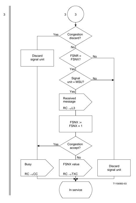
Figure 16/Q.703 (sheet 4 of 6) – Preventive cyclic retransmission – Reception control
