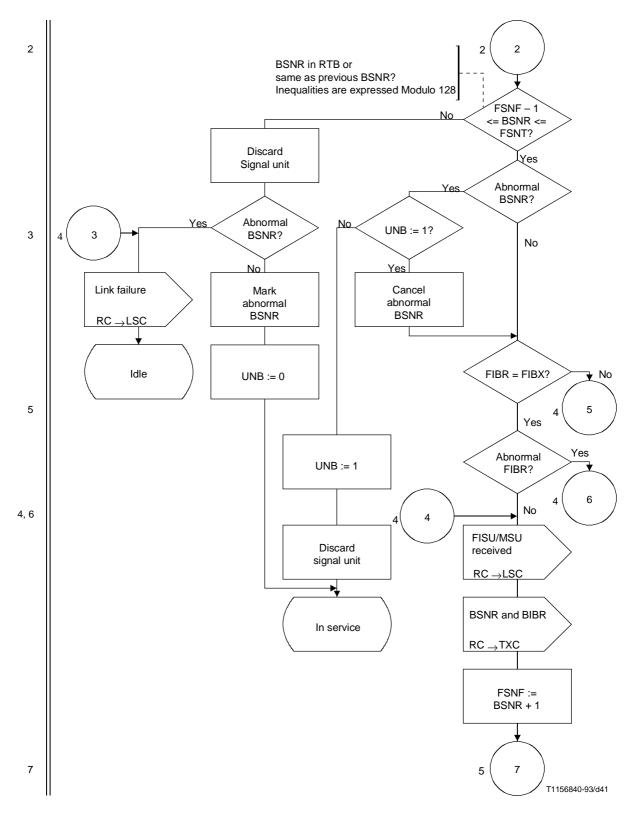
Figure 14/Q.703 (sheet 3 of 7) – Basic reception control
