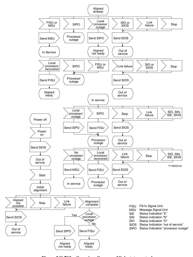
Figure 2/Q.703 – Overview diagram of link state control
