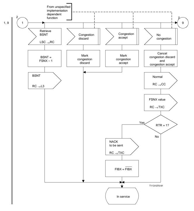
Figure 14/Q.703 (sheet 6 of 7) – Basic reception control
