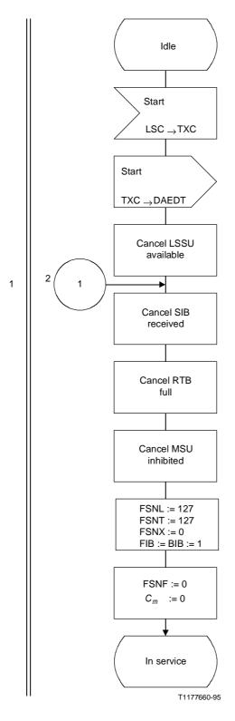
Figure 13/Q.703 (sheet 1 of 7) – Basic transmission control
