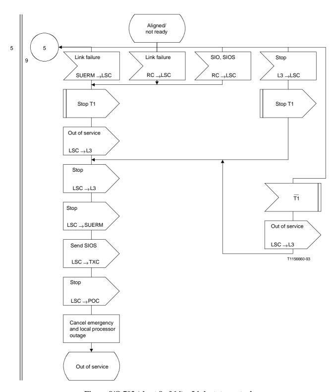
Figure 8/Q.703 (sheet 8 of 14) – Link state control
