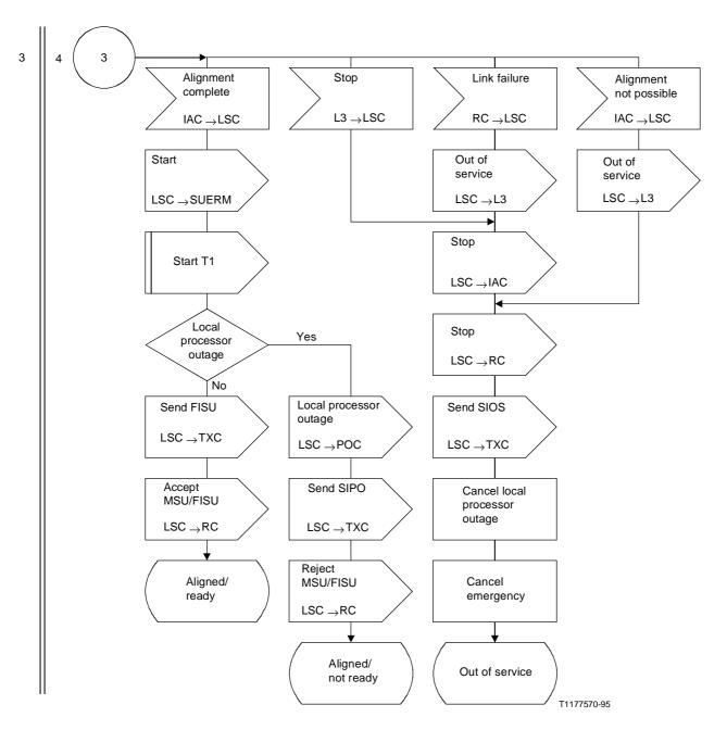
Figure 8/Q.703 (sheet 5 of 14) – Link state control
