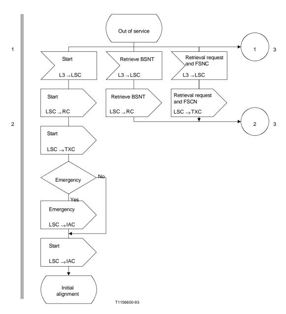
Figure 8/Q.703 (sheet 2 of 14) – Link state control
