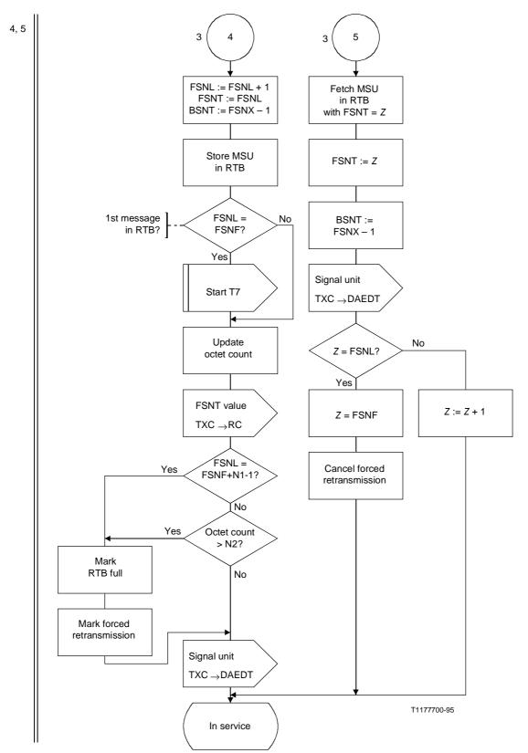
Figure 15/Q.703 (sheet 4 of 7) – Preventive cyclic retransmission – Transmission control
