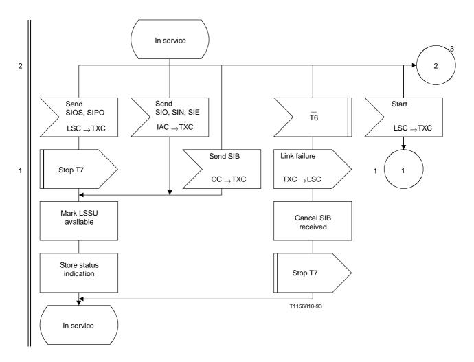
Figure 13/Q.703 (sheet 2 of 7) – Basic transmission control
