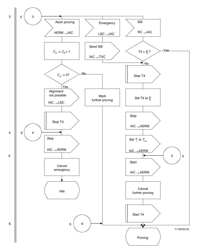
Figure 9/Q.703 (sheet 6 of 6) – Initial alignment control
