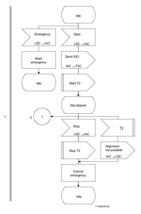
Figure 9/Q.703 (sheet 1 of 6) – Initial alignment control
