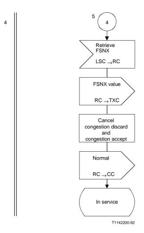
Figure 16/Q.703 (sheet 6 of 6) – Preventive cyclic retransmission – Reception control
