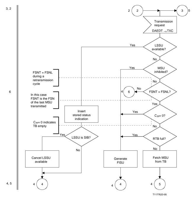
Figure 13/Q.703 (sheet 3 of 7) – Basic transmission control
