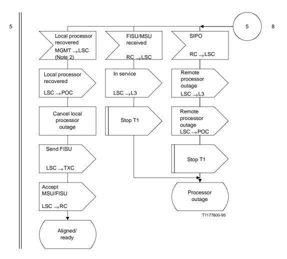
Figure 8/Q.703 (sheet 9 of 14) – Link state control
