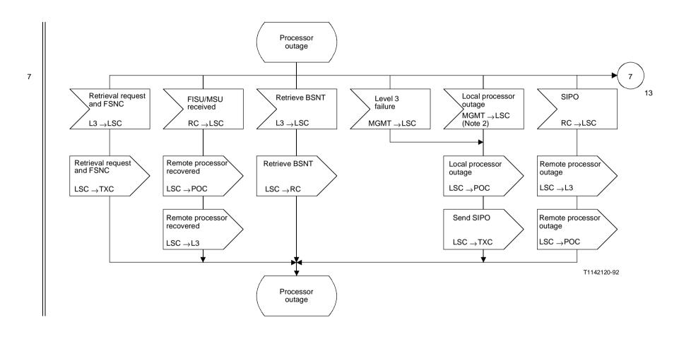
Figure 8/Q.702 (sheet 12 of 14) – Link state control
