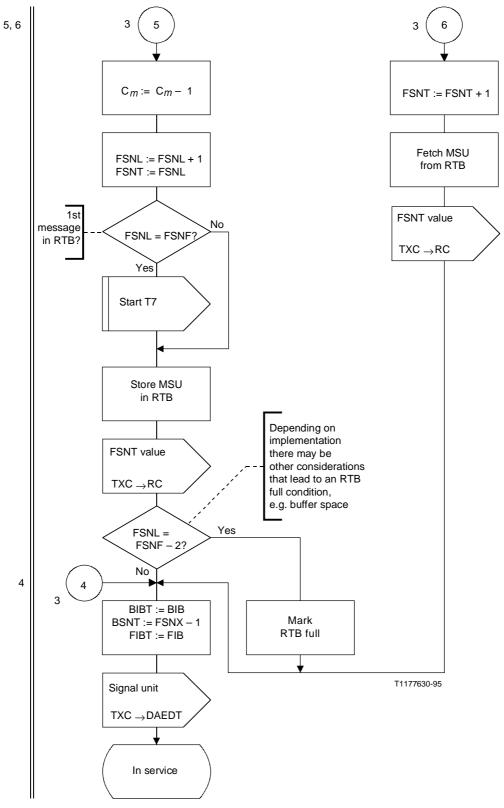
Figure 13/Q.703 (sheet 4 of 7) – Basic transmission control
