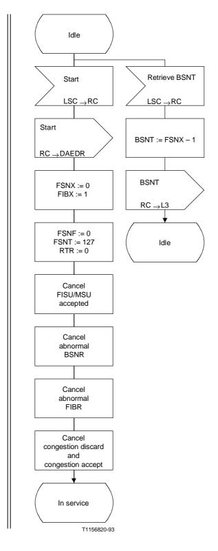
Figure 14/Q.703 (sheet 1 of 7) – Basic reception control
