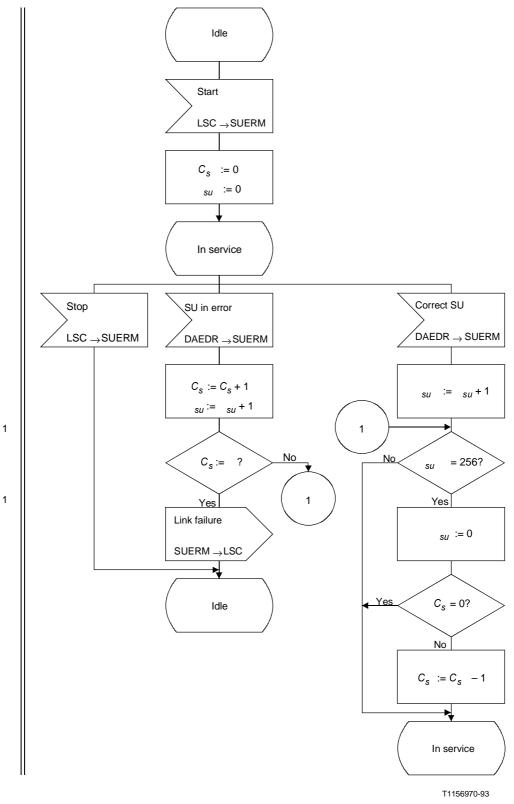
Figure 18/Q.703 – Signal unit error rate monitor
