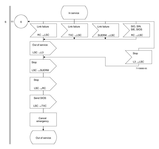
Figure 8/Q.703 (sheet 10 of 14) – Link state control
