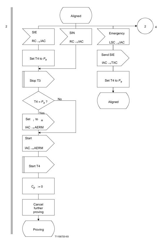
Figure 9/Q.703 (sheet 3 of 6) – Initial alignment control
