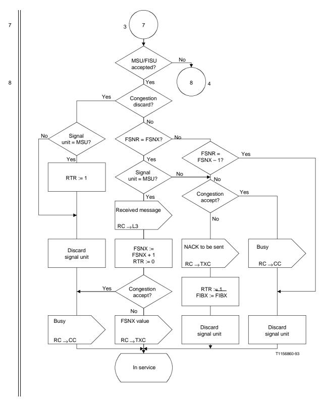
Figure 14/Q.703 (sheet 5 of 7) – Basic reception control
