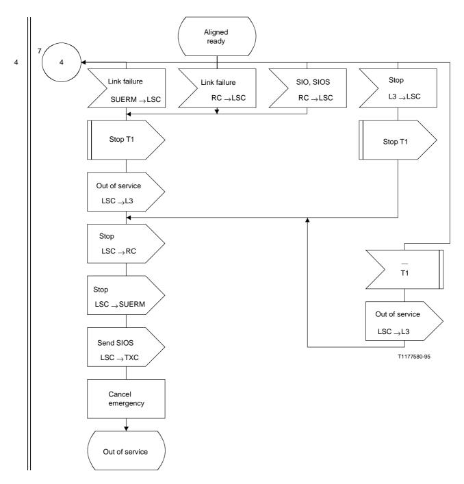
Figure 8/Q.703 (sheet 6 of 14) – Link state control
