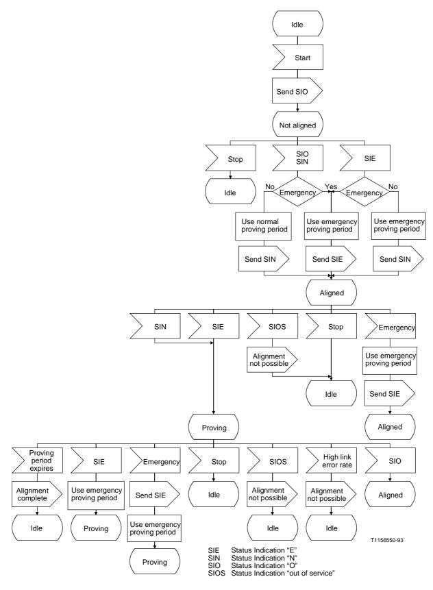
Figure 4/Q.703 - Overview diagram of initial alignment control
