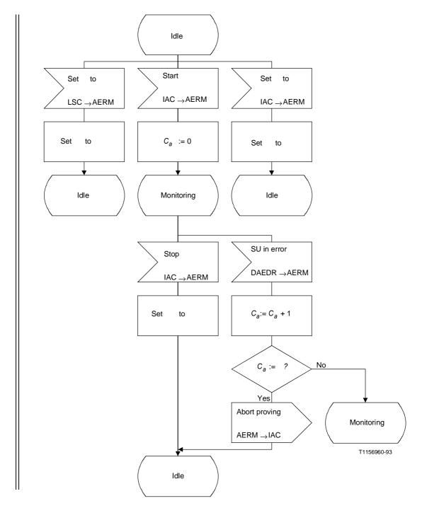
Figure 17/Q.703 – Alignment error rate monitor
