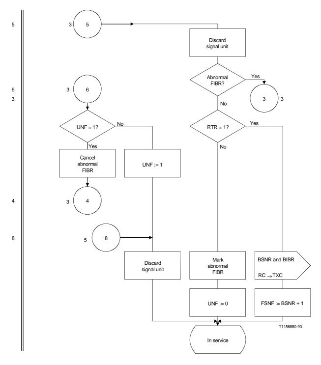
Figure 14/Q.703 (sheet 4 of 7) – Basic reception control
