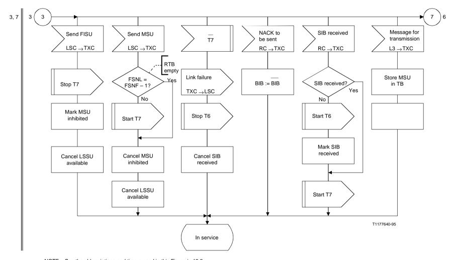
Figure 13/Q.703 (sheet 5 of 7) – Basic transmission control
