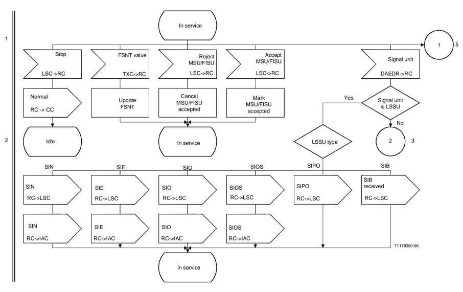
Figure 16/Q.703 (sheet 2 of 6) – Preventive cyclic retransmission – Reception control
