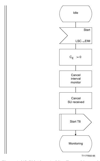
Figure A.2/Q.703 (sheet 1 of 2) – Errored interval monitor for 1.5 and 2.0 Mbit/s links
