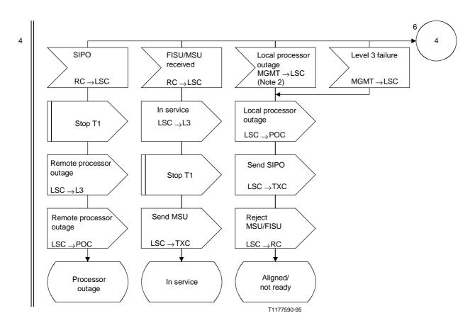
Figure 8/Q.703 (sheet 7 of 14) – Link state control
