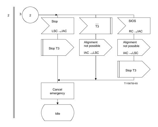
Figure 9/Q.703 (sheet 4 of 6) – Initial alignment control
