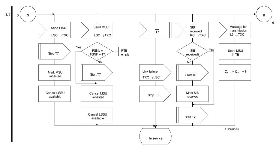
Figure 15/Q.703 (sheet 5 of 7) – Preventive cyclic retransmission – Transmission control
