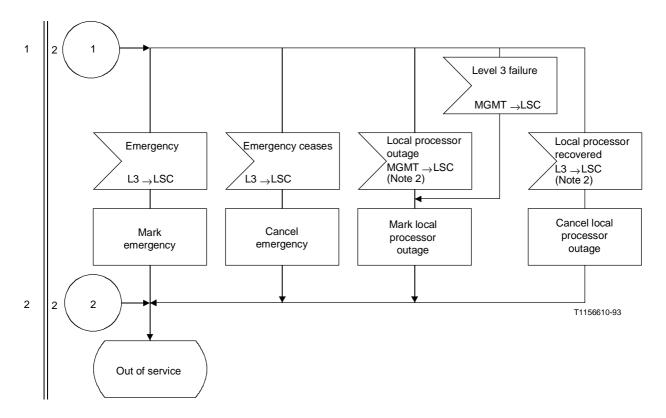
Figure 8/Q.703 (sheet 3 of 14) – Link state control
