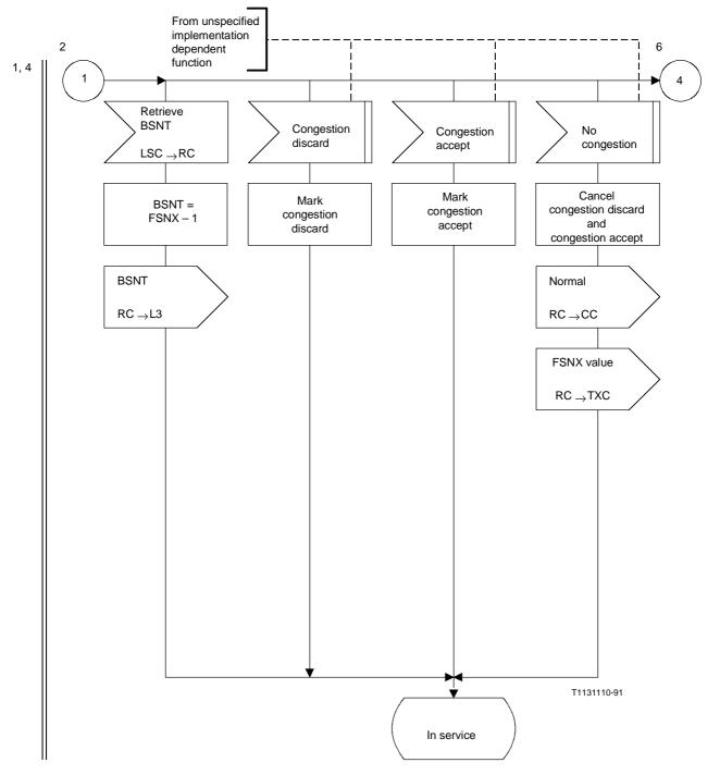
Figure 16/Q.703 (sheet 5 of 6) – Preventive cyclic retransmission – Reception control
