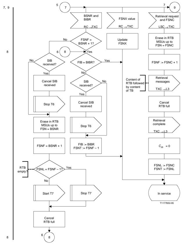
Figure 13/Q.703 (sheet 6 of 7) – Basic transmission control
