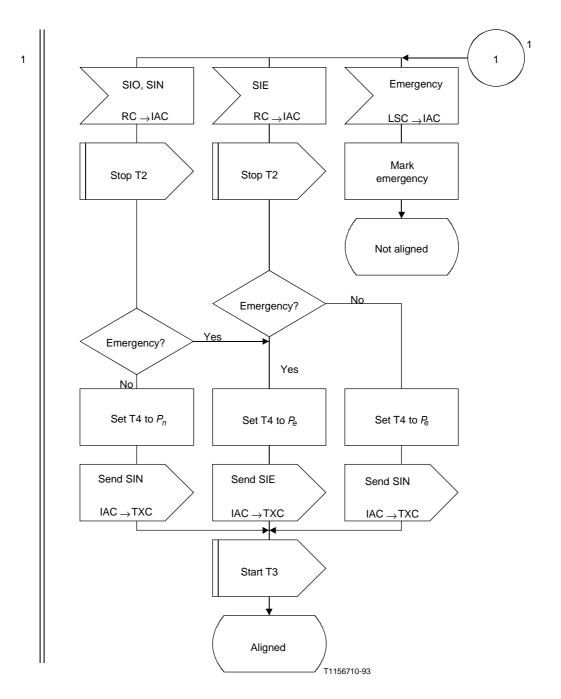
Figure 9/Q.703 (sheet 2 of 6) – Initial alignment control
