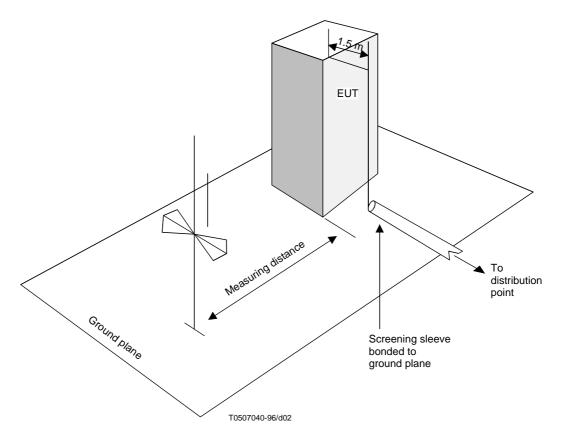
NOTE 1 – The EUT is separated from the ground plane with an electrically isolating support, and electrically bonded to the site power supply ground using normal installation practice as possible.
