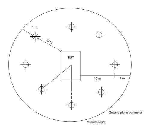
NOTE - The envelope of the EUT in this figure includes the cables as shown in Figures 2, 3 and 4.
