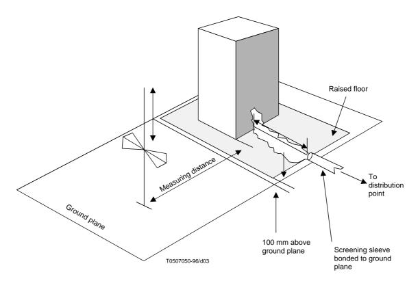
NOTE 1 - If the raised floor does not form part of the screen, the floor panels are removed. The raised floor is isolated from the EUT screen.
