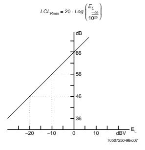
Figure I.4/K.10 – Admissible minimum  $LCL_R$  value as a function of the interference level parameter Ud = 0.5 mV (-66 dBV)
