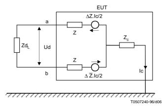
$\mathrm{Zd}_{\mathrm{L}}\,$  differential mode impedance measured at the end of the line connected to the EUT
