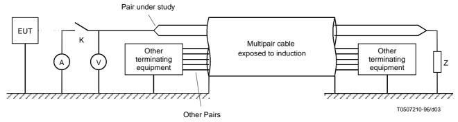
Z common mode impedance characterizing the remote termination connected at the pair under study
