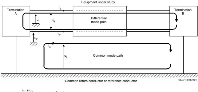
$\begin{aligned} \mathbf{u_c} &= \frac{\mathbf{u_1} + \mathbf{u_2}}{2} & \text{common mode voltage} \\ \mathbf{i_c} &= \mathbf{i_1} + \mathbf{i_2} & \text{common mode current} \\ \mathbf{u_d} &= \mathbf{u_1} - \mathbf{u_2} & \text{differential mode voltage} \end{aligned}$
