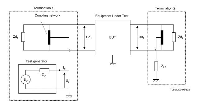
Zd<sub>1</sub>, Zd<sub>2</sub> differential mode impedance of terminations
