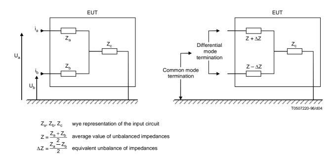
Figure I.1/K.10 – wye equivalent circuit of an equipment with unbalance about common conductor
