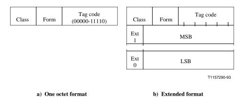
Figure 6/Q.773 – Format of the Tag code
