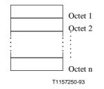
Figure 2/Q.773 – Octet labelling scheme
