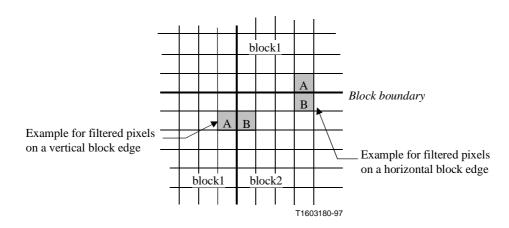
Figure Q.10/H.263 – Default block boundary filter
