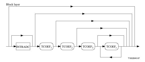
Figure E.1/H.263 – Structure of SAC Block layer
