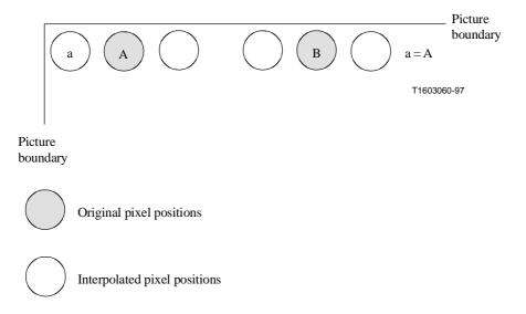
Figure O.11/H.263 – Method for 1-D interpolation at picture boundaries
