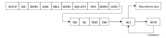
Figure N.3/H.263 – Structure of slice layer for NEWPRED
