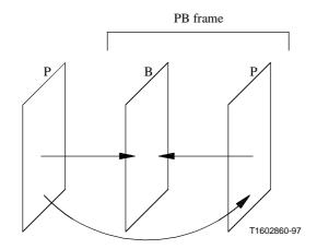
Figure G.1/H.263 – Prediction in PB-frames mode
