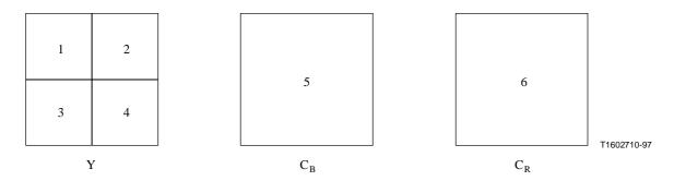
Figure 5/H.263 – Arrangement of blocks in a macroblock
