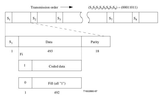
Figure H.1/H.263 – Error correcting frame
