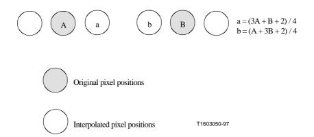
Figure O.10/H.263 – Method for interpolating pixels for 1-D scalability
