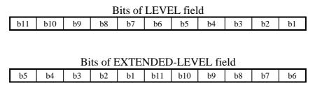
Figure T.1/H.263 – Cyclic rotation of coefficient representation
