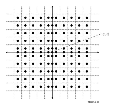
Figure Q.3/H.263 – Reconstruction of motion vector
