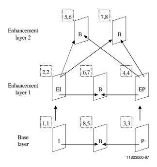
Figure O.5/H.263 – Example of picture transmission order
