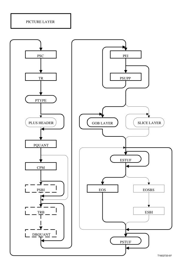
Figure 6/H.263 (part 1 of 7) – Syntax diagram for the video bitstream
