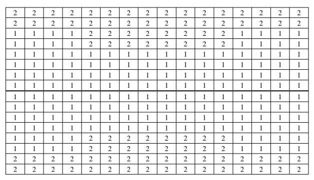
Figure Q.5/H.263 – Weighting values,  $H_1$ , for prediction with motion vector of current  $16 \times 16$  luminance blocks on top or bottom of current  $16 \times 16$  luminance block
