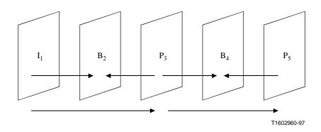
Figure O.1/H.263 – Illustration of B-picture prediction dependencies
