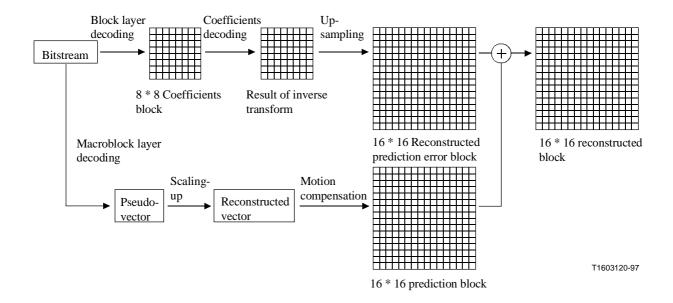
Figure Q.1/H.263 – Block diagram of block decoding in Reduced-Resolution Update mode
