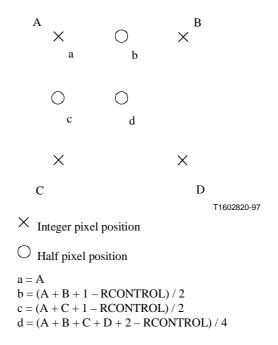
Figure 13/H.263 – Half-pixel prediction by bilinear interpolation
