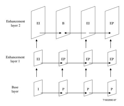
Figure O.4/H.263 – Illustration of multilayer scalability
