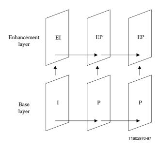
Figure O.2/H.263 – Illustration of SNR scalability
