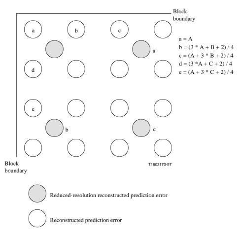
Figure Q.9/H.263 – Creation of reconstructed prediction error for pixels at the block boundary
