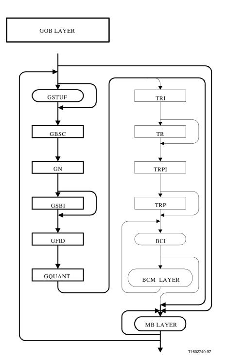
Figure 6/H.263 (part 3 of 7) – Syntax diagram for the video bitstream
