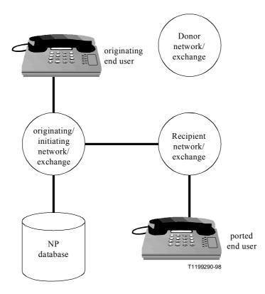
Figure 2 – PNCC-SPP configuration – Identical originating and initiating networks/exchanges
