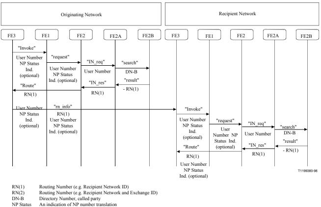
Route An operation from SSF storing a new routing number in CCF
