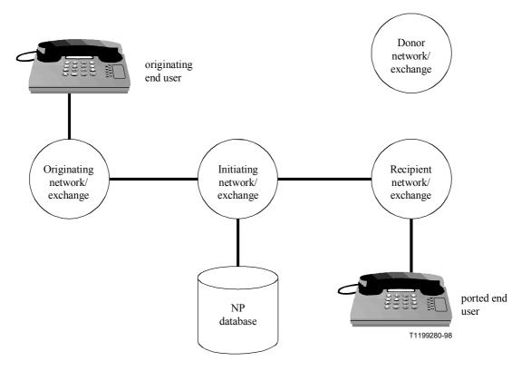
Figure 1 – PNCC-SPP configuration – Separate originating, initiating, donor networks/exchanges
