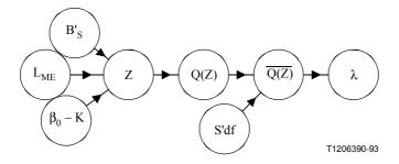
Figure A.3/P.79 – Simplified flow diagram showing how loudness,  $\lambda$ , is related to sensation level, Z
