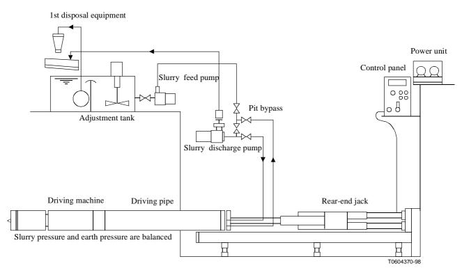
Figure I.5/L.38 – Example of slurry method
