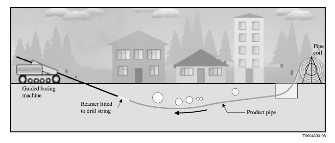
Figure I.1b/L.38 – General scheme of the directional drilling technique: backreaming and pulling in the product pipe
