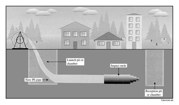
Figure I.2/L.38 – Pipe installation by impact moling
