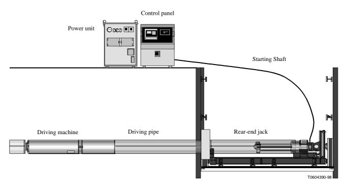
Figure I.7/L.38 – Example of penetrating method
