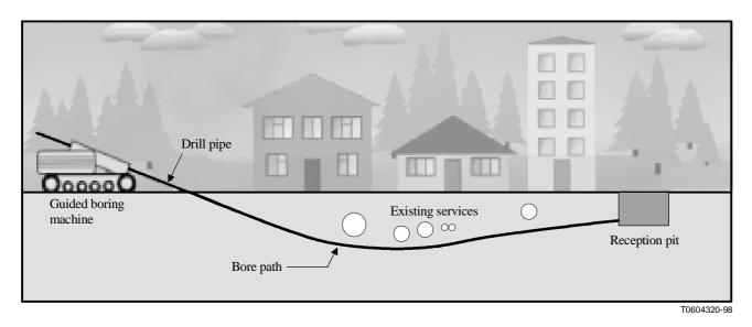
Figure I.1a/L.38 – General scheme of the directional drilling technique: drilling the pilot hole
