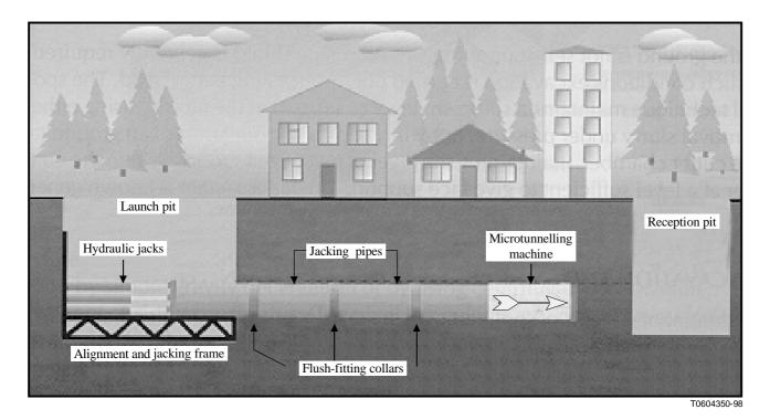
Figure I.3/L.38 – Installing pipes by microtunnelling
