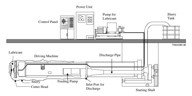
Figure I.6/L.38 – Example of slurry pressure balanced method
