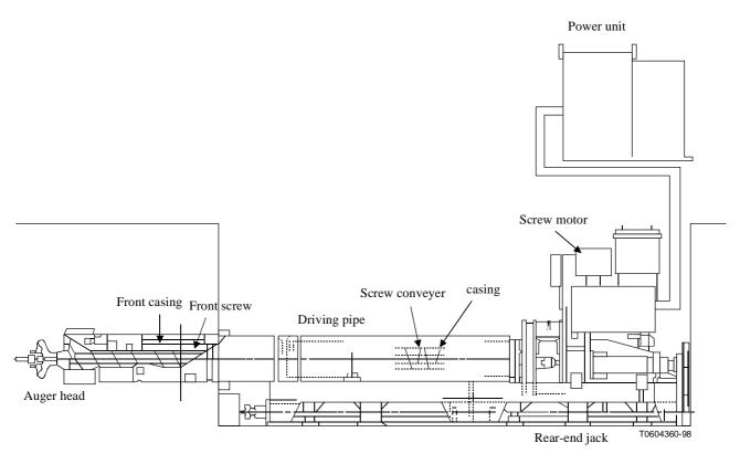
Figure I.4/L.38 – Example of auger excavation method
