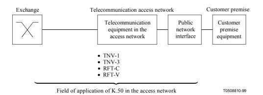
Figure 1b/K.50 – Field of application of K.50 in the access network
