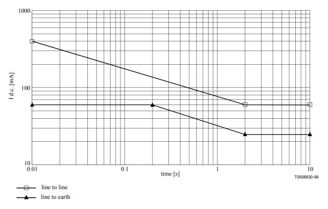
Figure B.1/K.50 – Maximum current after a single fault
