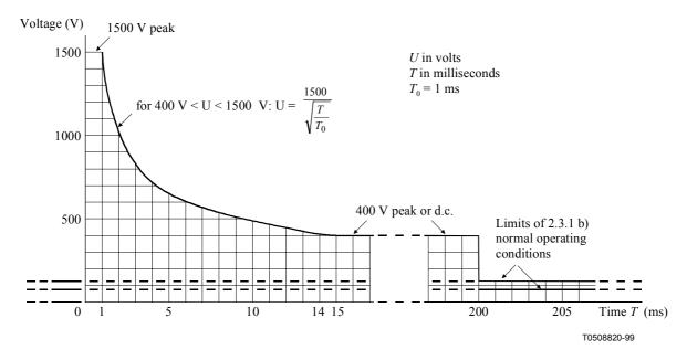
Figure A.1/K.50 – Maximum voltages permitted after a single fault (IEC 60950 [2] Figure 2D)
