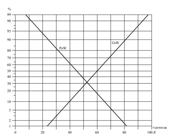
Figure B.1/G.107 – GoB (Good or Better) and PoW (Poor or Worse) as functions of rating factor *R*
