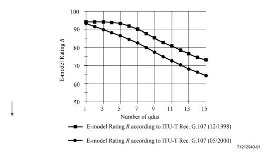
Figure A.1/G.107 – Relation between the number of qdu and E-model Rating R
