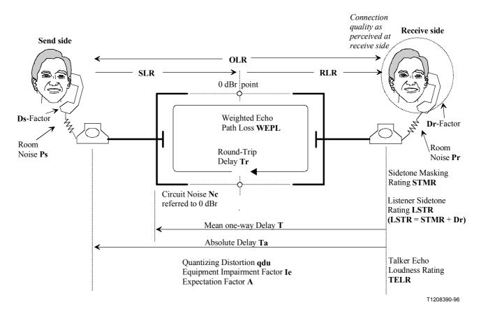
Figure 1/G.107 – Reference connection of the E-model
