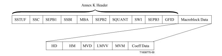
Figure V.1/H.263 – Data partitioning syntax
