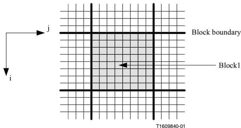
**Figure III.4/H.263 – Example of pixels' positions**
