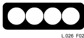
Figure 2/L.26 – Cross-section of a typical encapsulated ribbon
