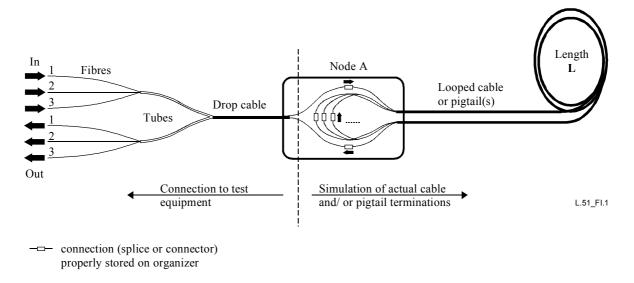
Figure I.1/L.51 – Storage of single fibre splices or connectors
