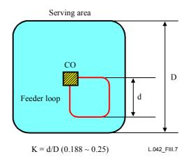
Figure III.7/L.42 – K, one side length ratio of feeder loop (d) versus the boundary (D) of CO's serving area
