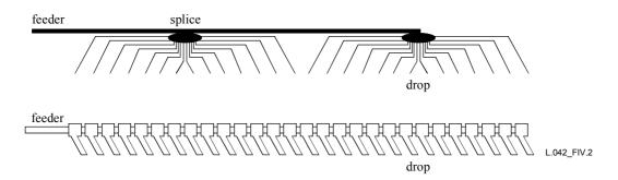
Figure IV.2/L.42 – Network structure with traditional cabling (above) and with mini-tubes (below)
