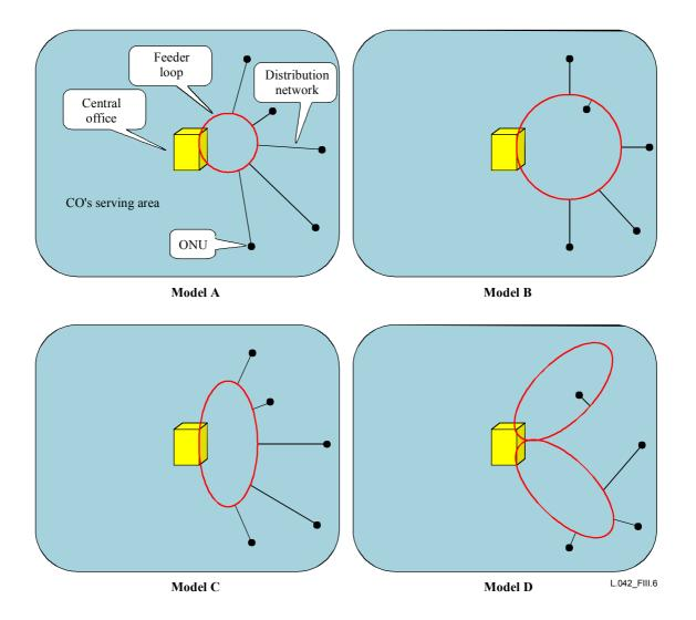
Figure III.6/L.42 – Some models of feeder loop configuration
