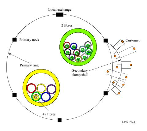
Figure IV.5/L.42 – Example of redundant network with mini-tube cabling for business customers
