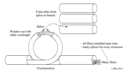
Figure IV.4/L.42 – A splice-point with cable-overlength when using traditional optical cabling
