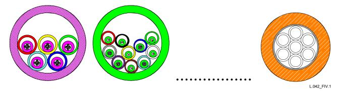
Figure IV.1/L.42 – Examples of loose bundles of mini-tubes (left and middle, for microcables with 24-60 and 2-24 optical fibres per mini-tube, respectively) and tight bundle of mini-tubes (right, for fibre members)
