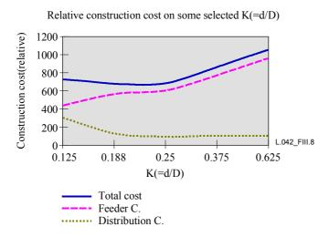
Figure III.8/L.42 – Relative construction cost on some selected K(=d/D)
