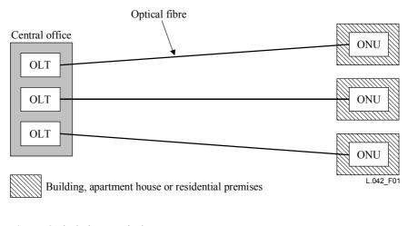
OLT Optical Line Terminal ONU Optical Network Unit
