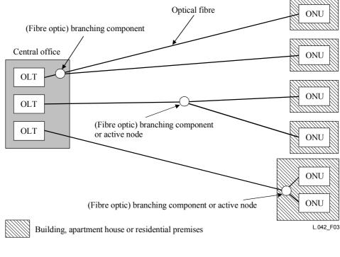
OLT Optical Line Terminal ONU Optical Network Unit
