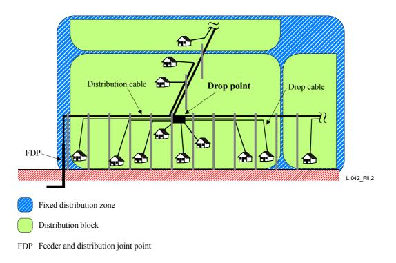
Figure II.2/L.42 – Distribution block configuration
