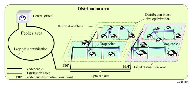
Figure II.1/L.42 – Optical access network configuration
