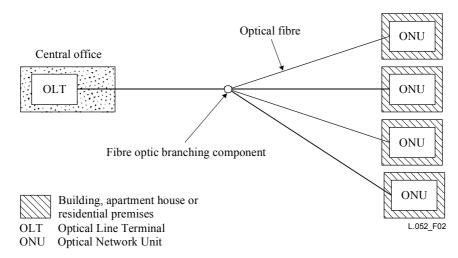
Figure 2/L.52 – PON configuration using (fibre optic) branching components for an outside plant (with 4 branches)
