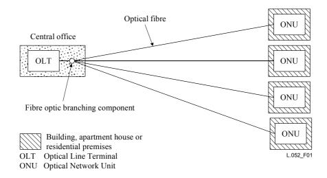
Figure 1/L.52 – PON configuration using (fibre optic) branching components for a central office (with 4 branches)
