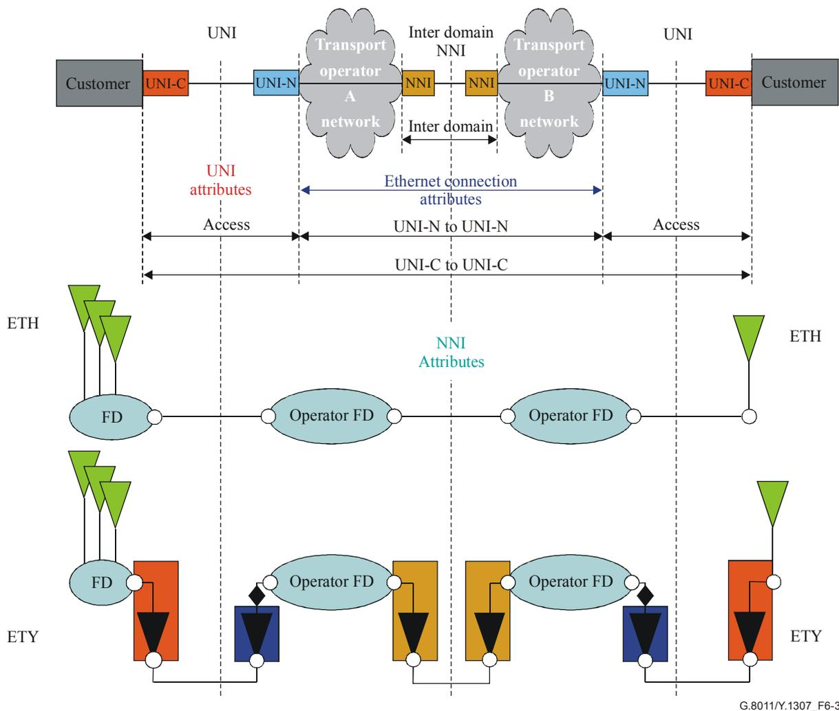
**Figure 6-3/G.8011/Y.1307 – Multi-provider with NNI view of Ethernet service areas**
