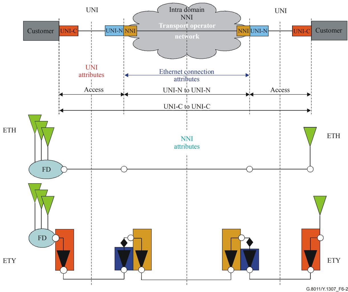
**Figure 6-2/G.8011/Y.1307 – Single provider with NNI view of Ethernet service areas**
