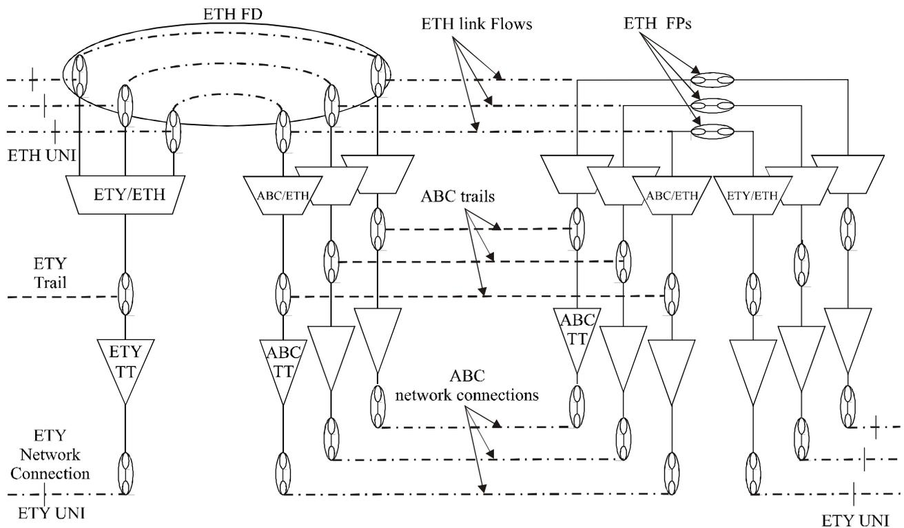
NOTE – for simplicity connection oriented technology ABC is shown on all server trails. Different technologies can also be used on each.
