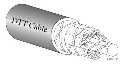
Figure I.1/L.60 – The 3-dimensional sketch map of the optical fibre/copper hybrid cable
