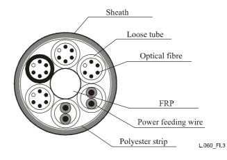
Figure I.3/L.60 – Cross-section of optical fibre/stranded copper wire hybrid cable
