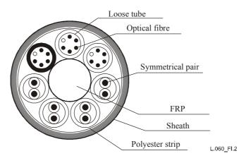
Figure I.2/L.60 – Construction of an optical fibre/symmetrical pair hybrid cable
