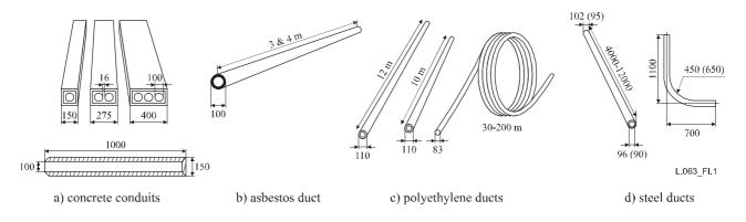
Figure I.1 – Different types of duct (concrete, asbestos, polyethylene, steel)
