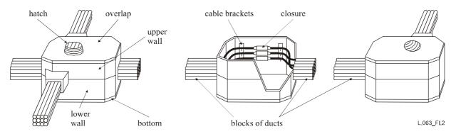
Figure I.2 – Building blocks of a communication duct
