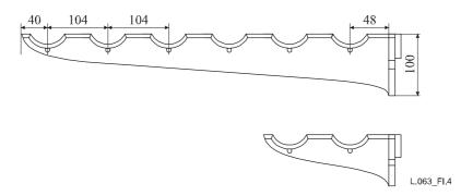
Figure I.4 – Cable brackets
