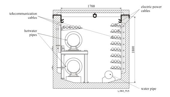
**Figure I.5 – Underground collector**
