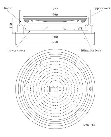
Figure I.3 – Cast hatch
