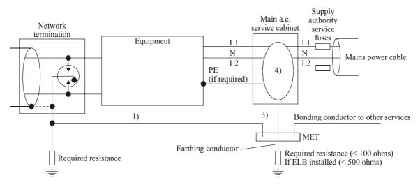
NOTE 1 – Total bonding wire to MET should be as short as possible (< 1.5 m if there is a significant risk of a direct lightning strike).
