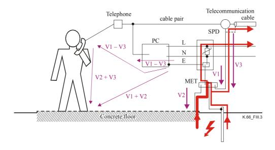
Figure III.3/K.66 – Lightning strike to ground resulting in EPR
