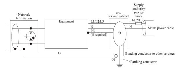
NOTE 1 – Total bonding wire to MET should be as short as possible (< 1.5 m if there is a significant risk of a direct lightning strike). NOTE 2 – Total of SPD connecting wires should be as short as possible (< 0.5 m).
