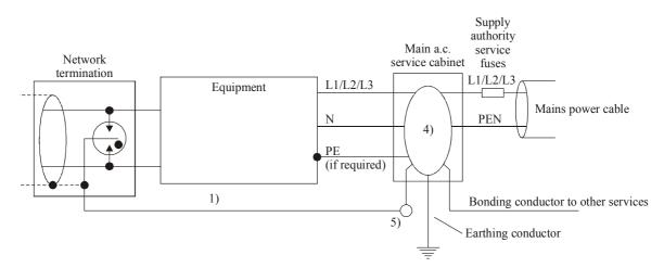
NOTE 1 – Total bonding wire to MET should be as short as possible (< 1.5 m if there is a significant risk of a direct lightning strike).
