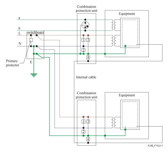
NOTE - SPDs 1), 2) and 3) need to be suitable for use on the mains. SPD 4) will need to be suitable to protect the equipments internal port.
