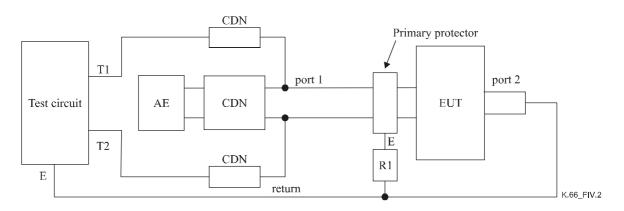
Figure IV.2/K.66 – Testing between ports R1: An earth resistance for a primary protector
