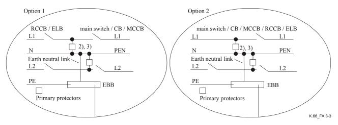
NOTE 5 – The SPD may be installed before the ELB (option 1) or after the ELB (option 2). If option 2 is used, nuisance tripping of the circuit breaker, particularly if it contains an RCD, may occur.
