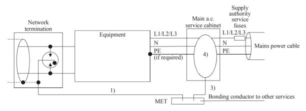
NOTE 1 – Total bonding wire to MET should be as short as possible (< 1.5 m if there is a significant risk of a direct lightning strike). NOTE 2 – Total of SPD connecting wires should be as short as possible (< 0.5 m).
