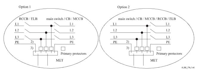
NOTE 6 – The SPD may be installed before the ELB (option 1) or after the ELB (option 2). If option 2 is used, nuisance tripping of the circuit breaker, particularly if it contains an RCD, may occur.
