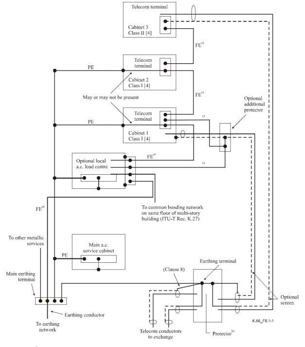
Figure 8.1-1 provides an example of a bonding configuration and earthing inside a customer's building.
