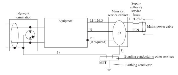
NOTE 1 – Total bonding wire to MET should be as short as possible (< 1.5 m if there is a significant risk of a direct lightning strike). NOTE 2 – Total of SPD connecting wires should be as short as possible (< 0.5 m).
