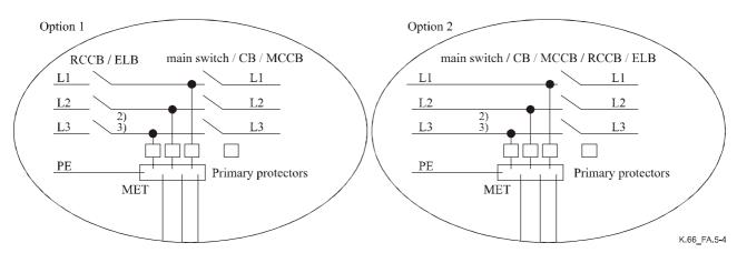
NOTE 6 – The SPD may be installed before the ELB (option 1) or after the ELB (option 2). If option 2 is used, nuisance tripping of the circuit breaker, particularly if it contains an RCD, may occur.
