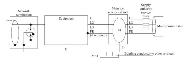
NOTE 1 – Total bonding wire to MET should be as short as possible (< 1.5 m if there is a significant risk of a direct lightning strike). NOTE 2 – Total of SPD connecting wires should be as short as possible (< 0.5 m).
