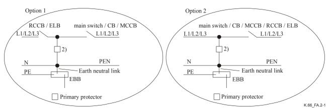
NOTE 5 – The SPD may be installed before the ELB (option 1) or after the ELB (option 2). If option 2 is used, nuisance tripping of the circuit breaker, particularly if it contains an RCD, may occur.
