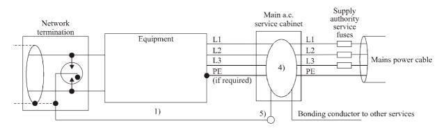
NOTE 1 – Total bonding wire to MET should be as short as possible (< 1.5 m if there is a significant risk of a direct lightning strike). NOTE 2 – Total of SPD connecting wires should be as short as possible (< 0.5 m).
