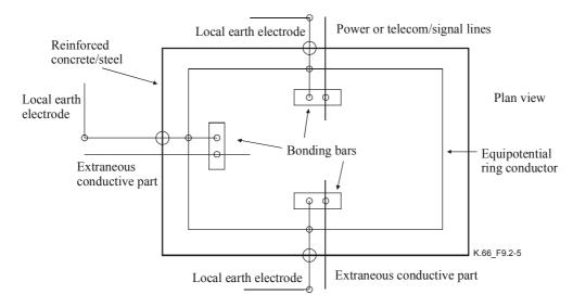
Figure 9.2-5/K.66 – Equipotential bonding of incoming metallic services entering at several points: Use of internal ring conductor
