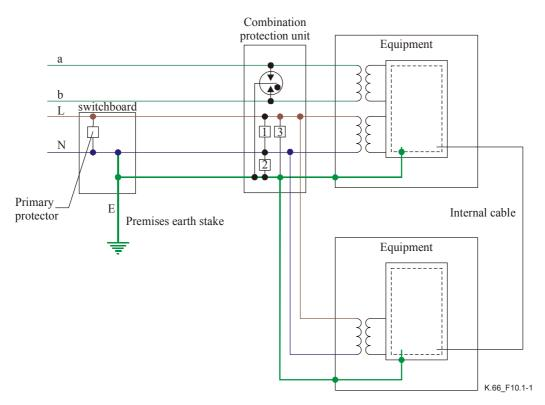
Figure 10.1-1/K.66 – Equipment protected by the same combination protector
