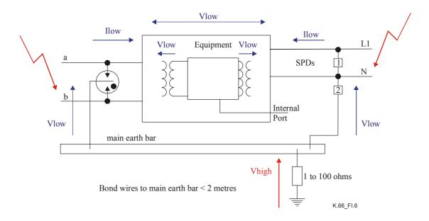
Figure I.6/K.66 – Installation has recommended earthing and bonding; equipment protected
