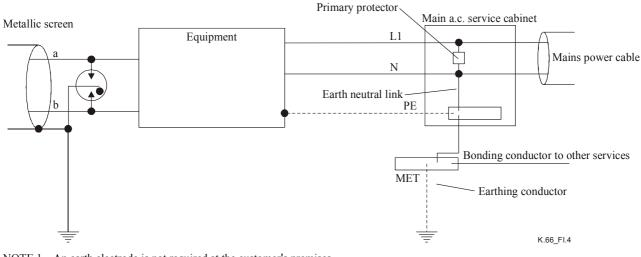
NOTE 1 – An earth electrode is not required at the customer's premises in all power systems, it may be supplied in the distribution network. NOTE 2 – The telecommunication cable may not always have a shield or be earthed.
