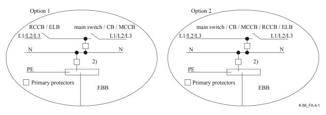
NOTE 5 – The SPD may be installed before the ELB (option 1) or after the ELB (option 2). If option 2 is used, nuisance tripping of the circuit breaker, particularly if it contains an RCD, may occur.
