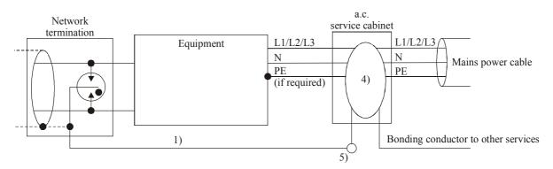
NOTE 1 – Total bonding wire to MET should be as short as possible (< 1.5 m if there is a significant risk of a direct lightning strike). NOTE 2 – Total of SPD connecting wires should be as short as possible (< 0.5 m).
