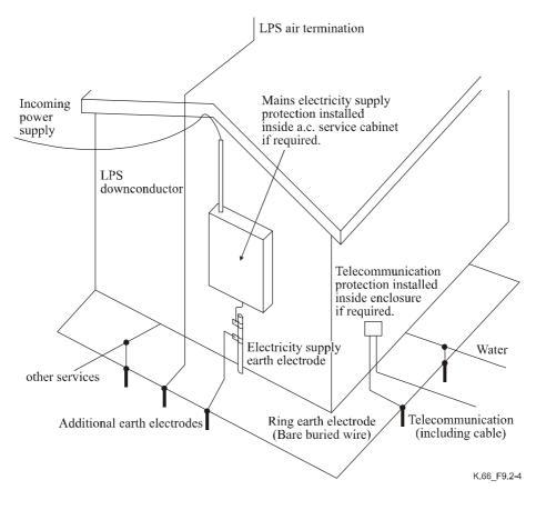
Figure 9.2-4/K.66 – Ring earth electrode
