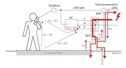
Figure III.1/K.66 – Lightning strike to phase conductor of the power line change all E to PE on diagram
