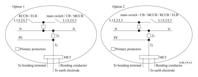
NOTE 6 – The SPD may be installed before the ELB (option 1) or after the ELB (option 2). If option 2 is used, nuisance tripping of the circuit breaker, particularly if it contains an RCD, may occur.
