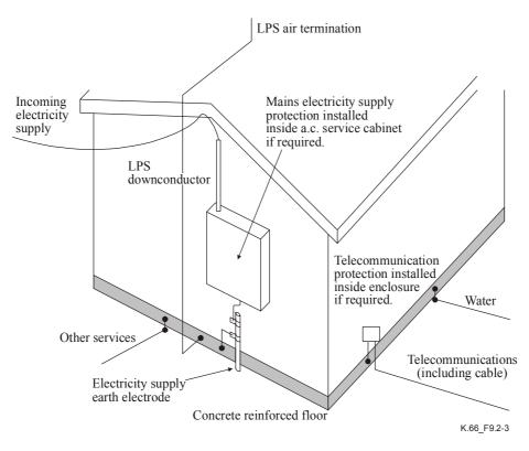
Figure 9.2-3/K.66 – Common bonding network (CBN)
