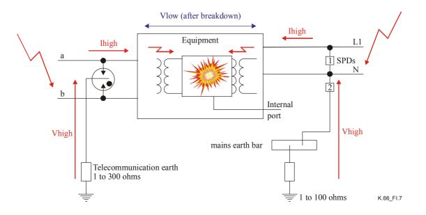
Figure I.7/K.66 – Installation has poor earthing and bonding; equipment damaged
