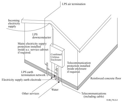
NOTE - The MET in this example is inside the combined utilities enclosure.
