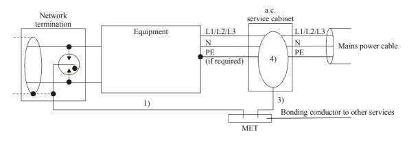
NOTE 1 – Total bonding wire to MET should be as short as possible (< 1.5 m if there is a significant risk of a direct lightning strike).
