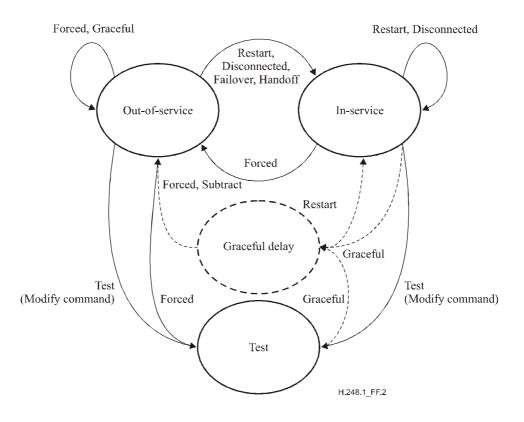
Figure F.2/H.248.1 – Simple ServiceChange state model
