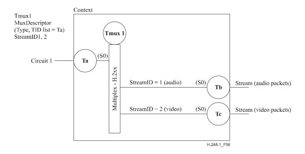
Figure 6/H.248.1 – Multiplexed termination scenario – Single-to-multiple terminations
