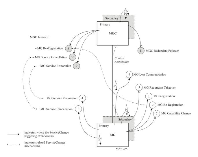
Figure F.1/H.248.1 – Trigger events for ServiceChange
