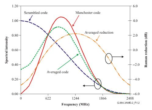
Figure V.2/G.984.3 – Spectra of ordinary scrambled pattern, Manchester-coded pattern, the average code, and the average reduction in spectral intensity
