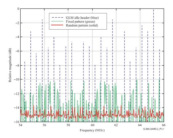
Figure V.1/G.984.3 – Spectrum after scrambling of the GEM idle header (blue-dashed), fixed 53-byte pattern (green-dotted), and random 53-byte pattern (red-solid)
