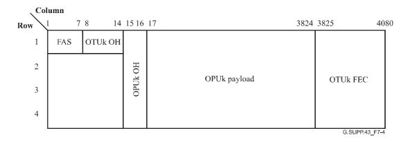
Figure 7-4 – Mapping frame without fixed stuff bytes
