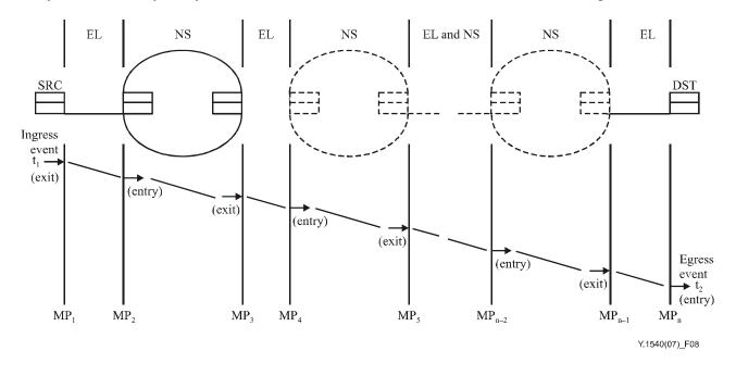
Figure 8 – IP packet transfer delay events (illustrated for the end-to-end transfer of a single IP packet)
