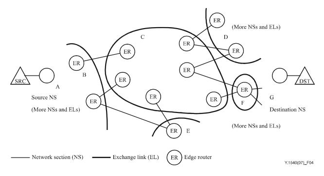
Figure 4 – IP network connectivity
