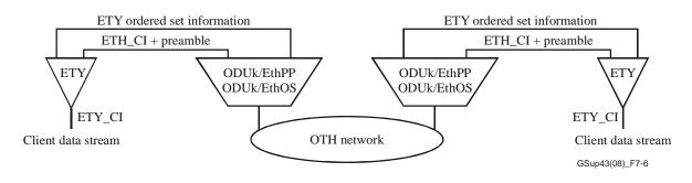
Figure 7-6 – Functional model for mapping 10GE information into the ODUk
