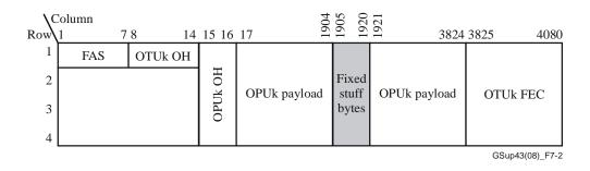
Figure 7-2 – Mapping frame with fixed stuff bytes
