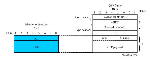
Figure 7-8 – Ethernet ordered set mapping into GFP-F
