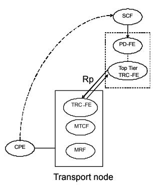
Figure IV.1 – Reference architecture for unicast and multicast admission control
