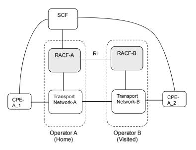
Figure VII.1 – Inter-operator RACF communications where one CPE is accommodated in a visited operator
