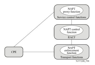
Figure 4 – NAPT and NAT traversal control mechanisms
