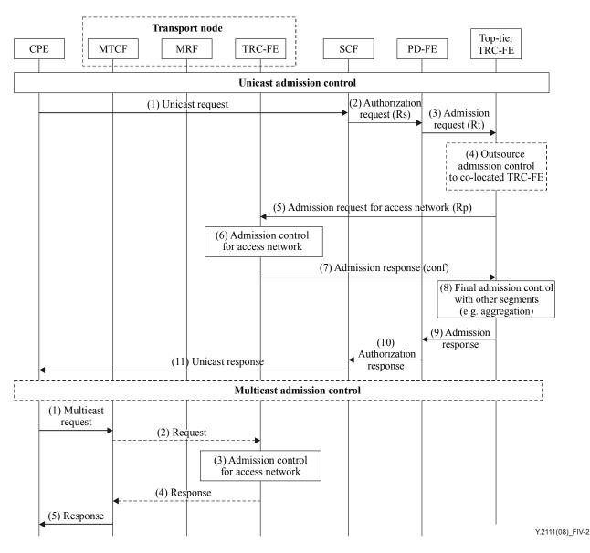
Figure IV.2 - Unicast and multicast admission control for fully shared resources
