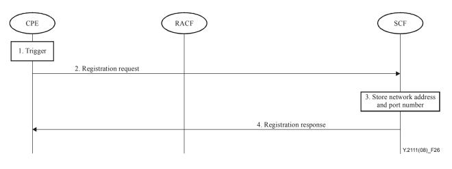
Figure 26 – NAT traversal procedure for signalling registration flows
