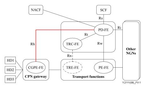
Figure V.1 – Resource and admission control functional architecture for the CPN gateway
