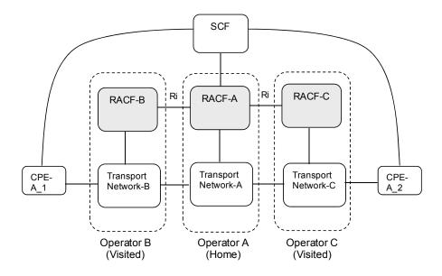
Figure VII.3 – Inter-operator RACF communications where two CPEs are accommodated in different visited operators
