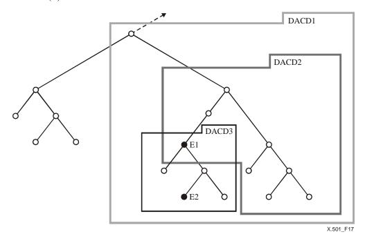
Figure 17 – Effective Access Control using DACDs
