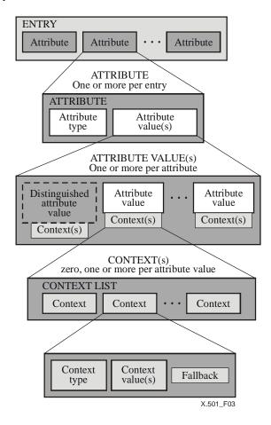
Figure 3 – Structure of an entry
