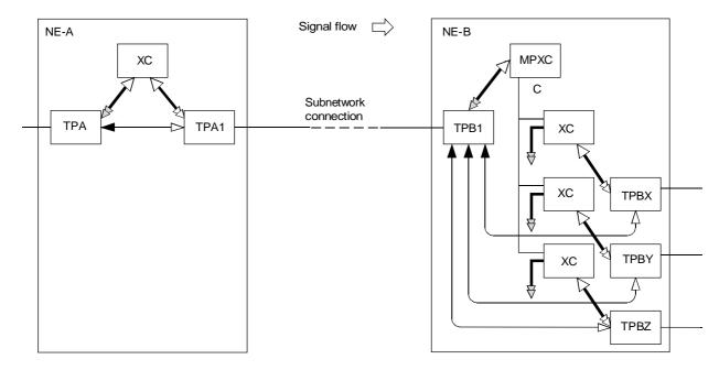
a) Non-protected unidirectional subnetwork connection between NE-A and NE-B with broadcast in NE-B
