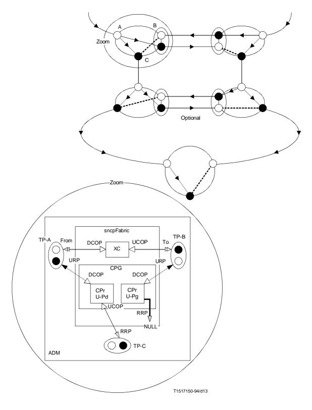
FIGURE B.11/G.774.04 Interconnections of subnetwork with ADMs (SNCP/SNCP) in SNCP interworking
