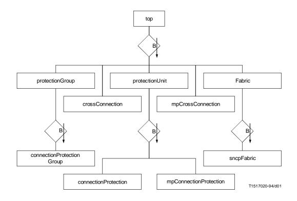
FIGURE A.1/G.774.04 Inheritance subtree of subnetwork connection protection
