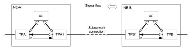
a) Non-protected bidirectional subnetwork connection between NE-A and NE-B
