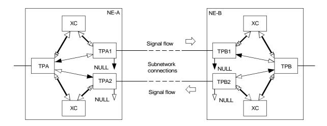
a) Non-protected bidirectional subnetwork connection diverse route between NE-A and NE-B
