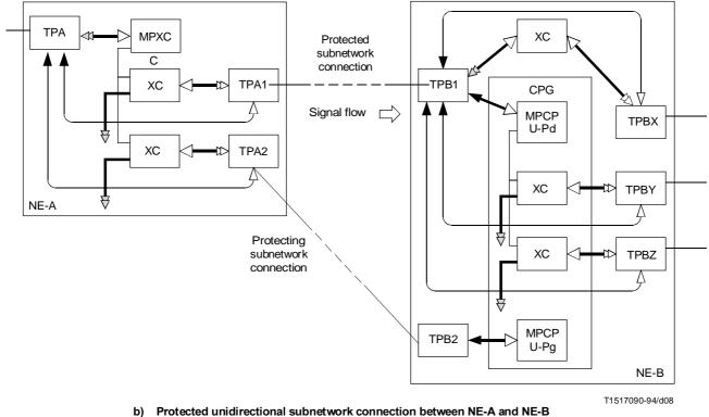
Protected unidirectional subnetwork connection between NE-A and NE-B with broadcast in NE-B
