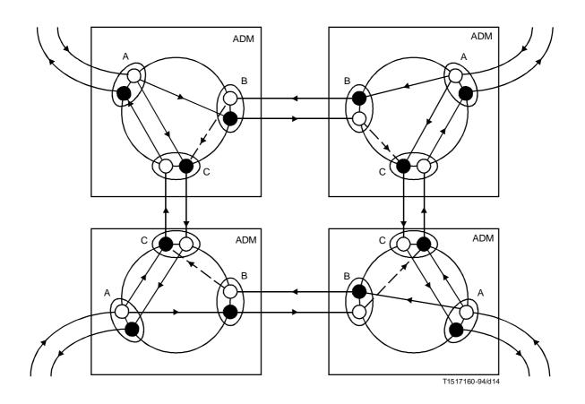
FIGURE B.12/G.774.04 Logical connections in SNCP interworking rings connectivity view
