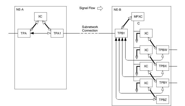
a) Non-protected unidirectional subnetwork connection between NE-A and NE-B with broadcast in NE-B
