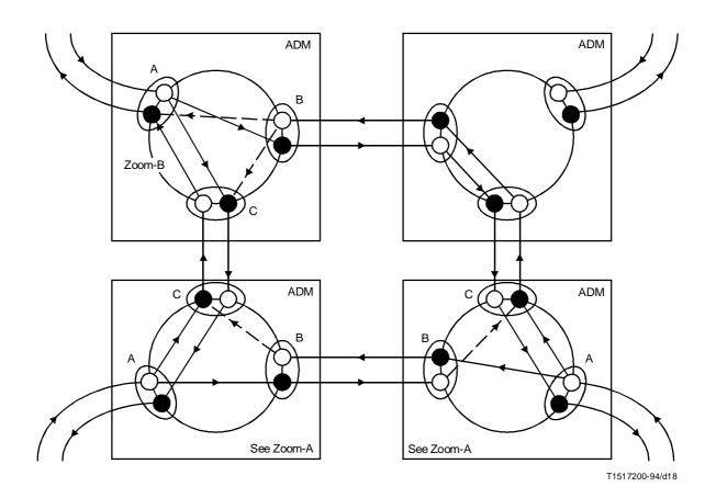
FIGURE B.16/G.774.04 Logical connections in SNCP Ring and MS SHARED RING interworking: connectivity view
