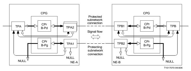
b) Protected bidirectional subnetwork connection between NE-A and NE-B
