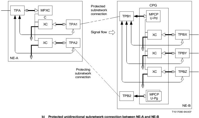
Protected unidirectional subnetwork connection between NE-A and NE-B with broadcast in NE-B
