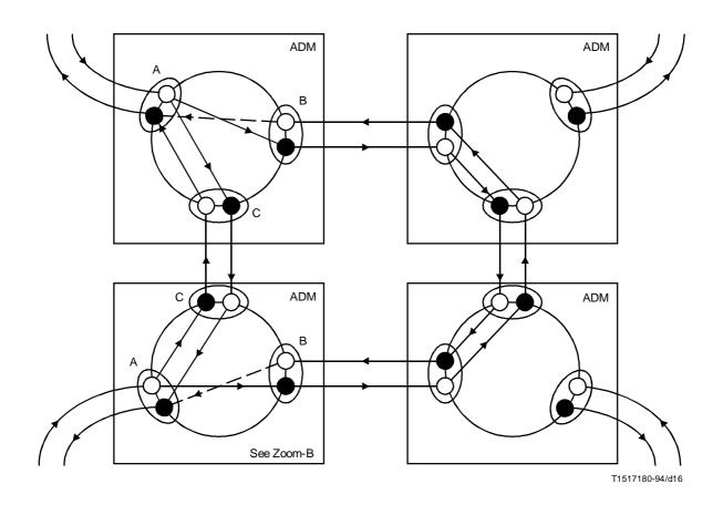
FIGURE B.14/G.774.04 Logical connections in MS SHARED RINGS interworking: connectivity view
