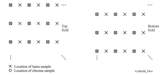
Figure 6-4 – Nominal vertical and horizontal sampling locations of 4:2:2 samples top and bottom fields
