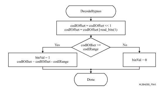
Figure 9-5 – Flowchart of bypass decoding process
