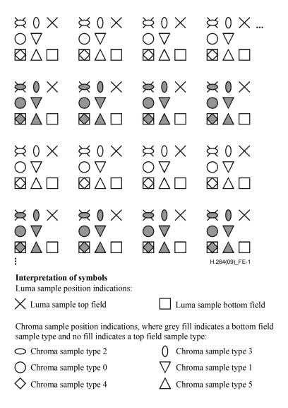
Figure E-1 – Location of chroma samples for top and bottom fields for chroma\_format\_idc equal to 1 (4:2:0 chroma format) as a function of chroma sample loc type top field and chroma sample loc type bottom field
