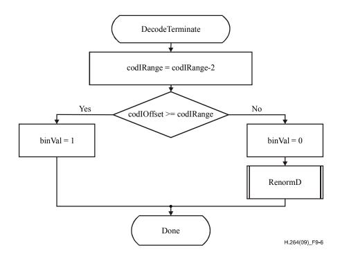
Figure 9-6 – Flowchart of decoding a decision before termination
