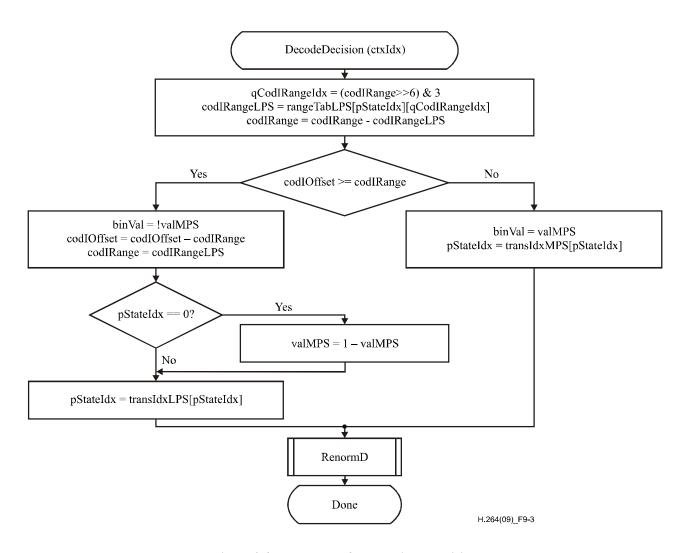
Figure 9-3 - Flowchart for decoding a decision
