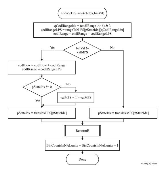
Figure 9-7 – Flowchart for encoding a decision
