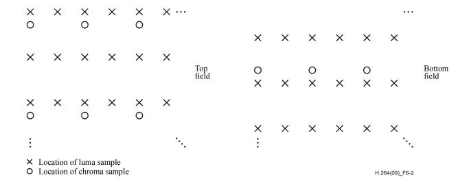
Figure 6-2 - Nominal vertical and horizontal sampling locations of 4:2:0 samples in top and bottom fields
