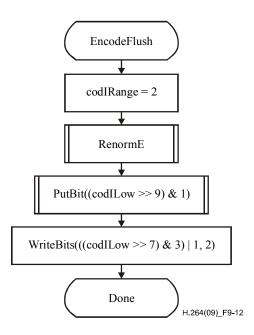
Figure 9-12 - Flowchart of flushing at termination
