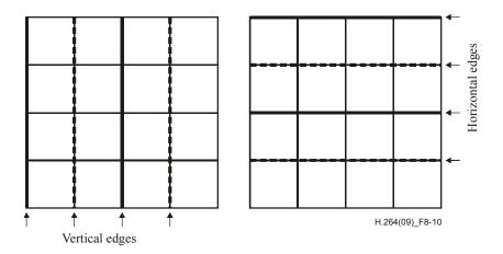
Figure 8-10 – Boundaries in a macroblock to be filtered
