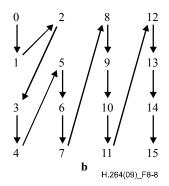
Figure 8-8 – 4x4 block scans. (a) Zig-zag scan. (b) Field scan (informative)
