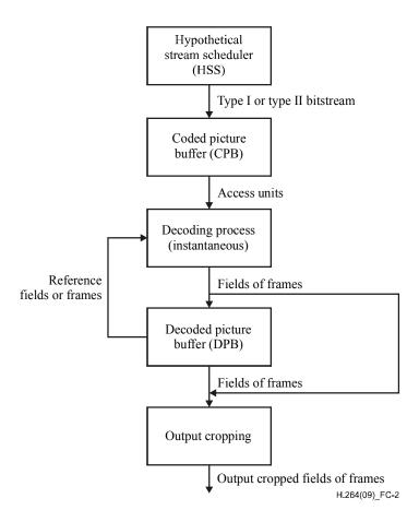
Figure C-2 – HRD buffer model
