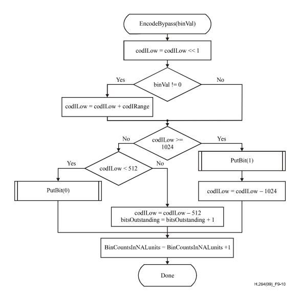
Figure 9-10 - Flowchart of encoding bypass
