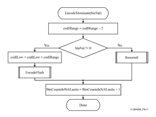
Figure 9-11 - Flowchart of encoding a decision before termination
