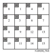
Figure 8-6 – Assignment of the indices of dcY to luma4x4BlkIdx
