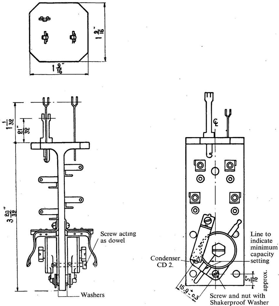
FIGURE 1. — Mounting for condensers and resistors used on carrier-cable distant-end crosstalk balancing networks
