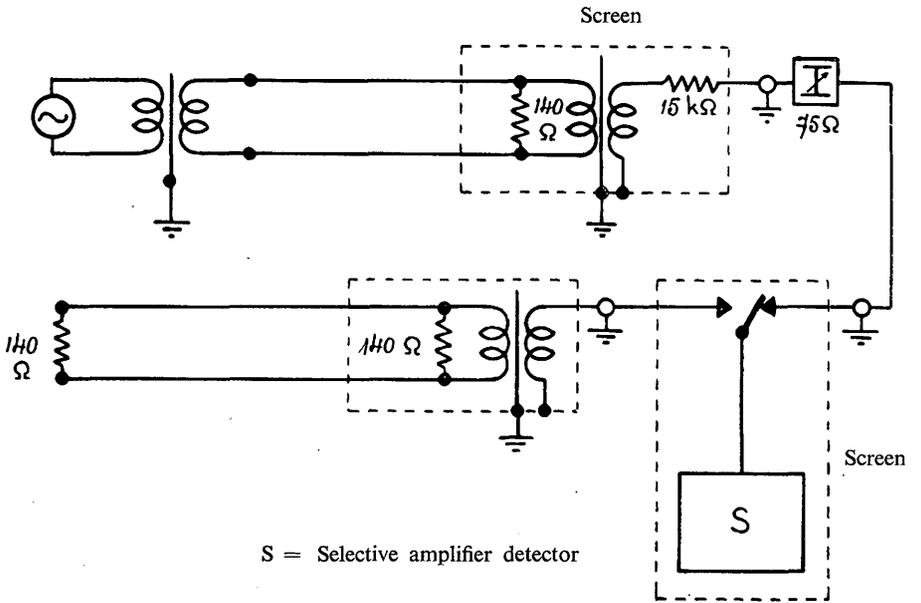
FIGURE 27. — Far-end crosstalk measurement between symmetrical pairs for carrier systems
