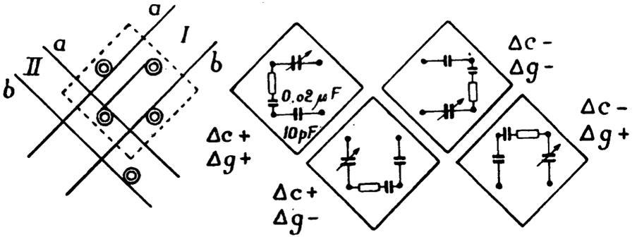
FIGURES 1. — Connection of balancing units to two pairs of wires
