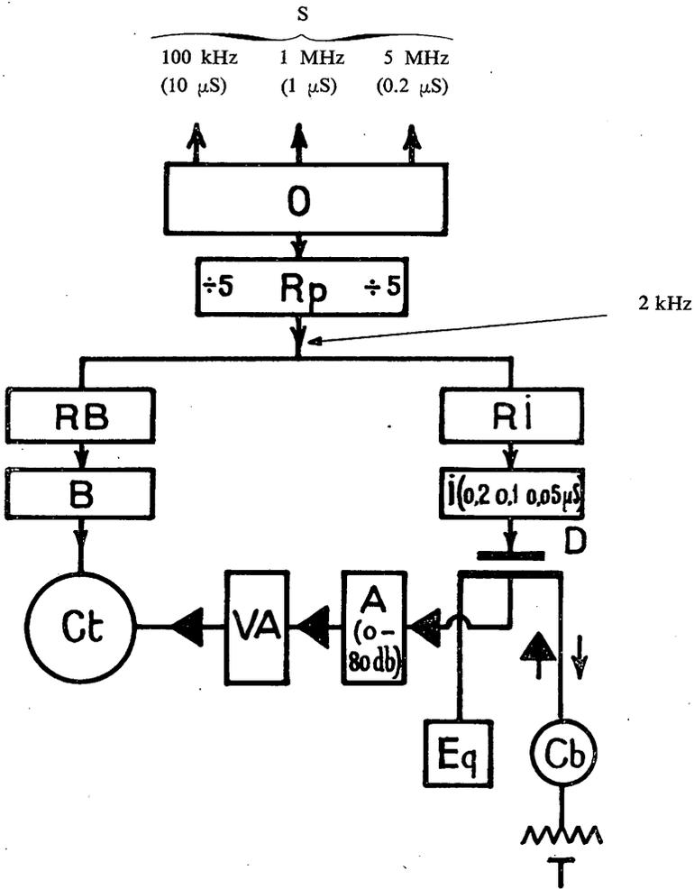
FIGURE 2. — Block schemater of Pulse Echo Measuring Equipment
