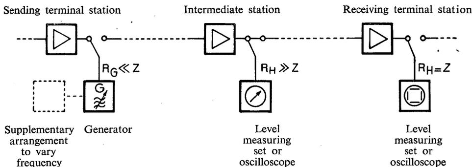
FIGURE 1. — Reference measurements carried out on a carrier system line
