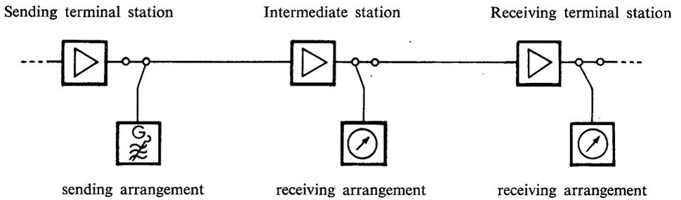
FIGURE 2. — Maintenance measurements made on a carrier system line in service by means of apparatus for measuring interstice frequencies
