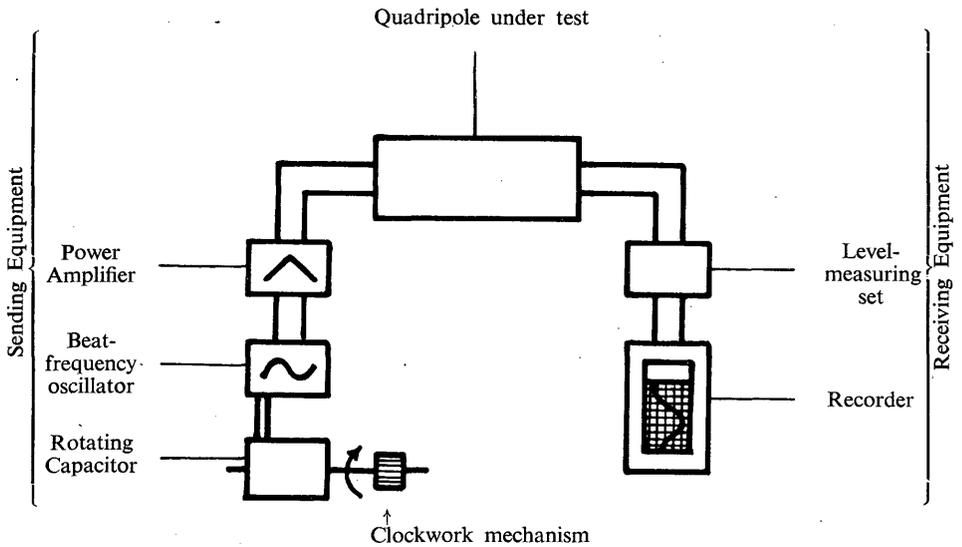
FIGURE 4. — Schematic of the automatic level recorder
