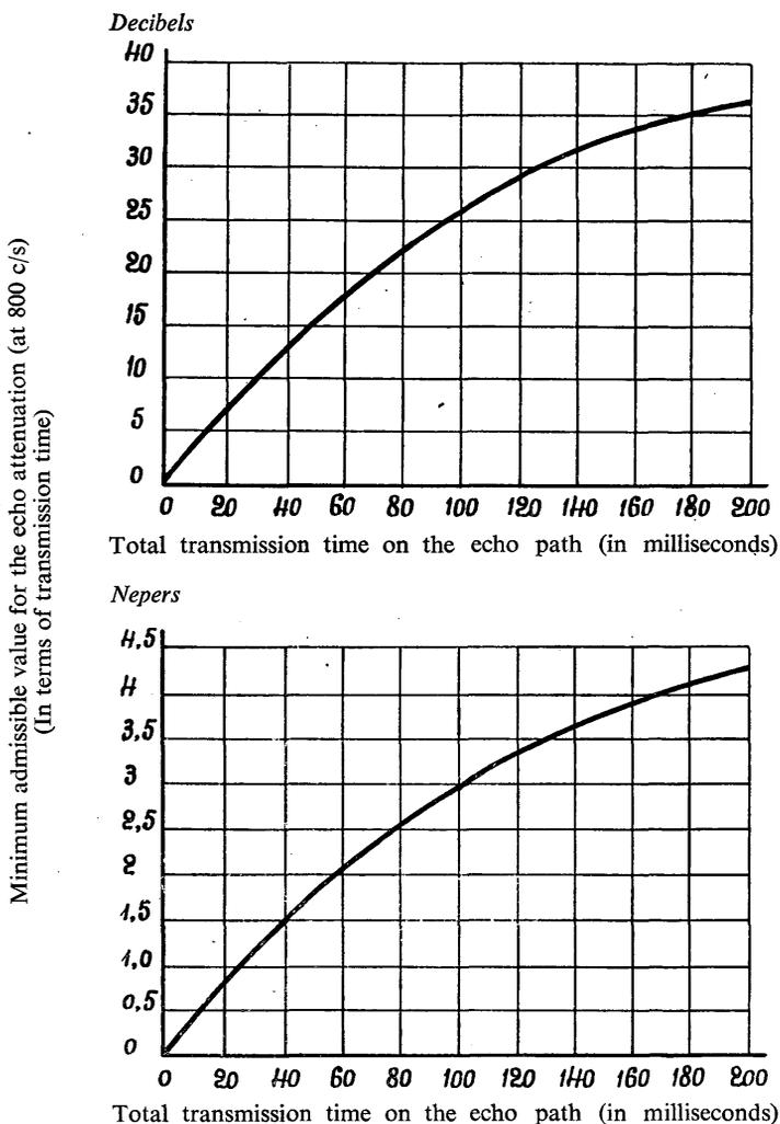
FIGURE 1. — Curve giving the minimum admissible value for echo attenuation for circuits without echo suppressors, as a function of total transmission time on the echo path
