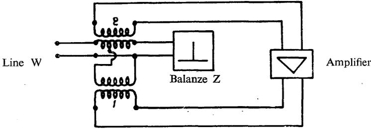
FIGURE 19. — *Return loss measuring set*
