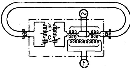
FIGURE 1. — *Impedance measuring set*
