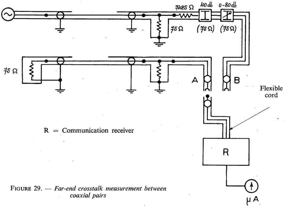
FIGURE 29. — Far-end crosstalk measurement between coaxial pairs
