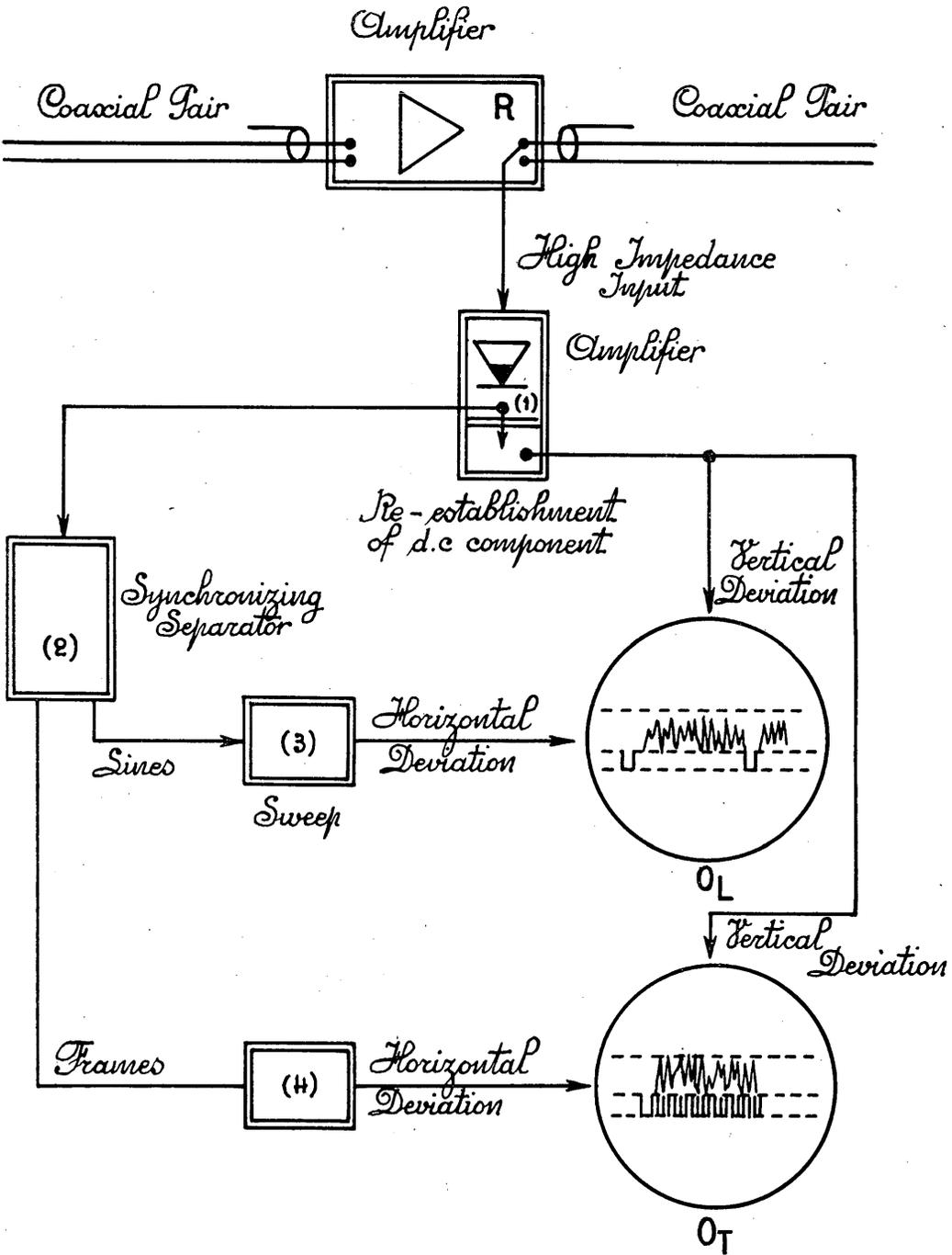
Apparatus for monitoring television transmissions by the Radiodiffusion française
