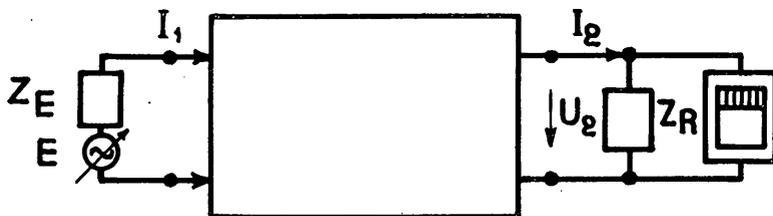
FIGURE 6. — *Measurement of Effective Insertion Loss or Gain with the Automatic Level Recorder*
