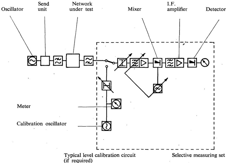
FIGURE 21. — Typical assembly of test equipment for measurement of harmonic distortion
