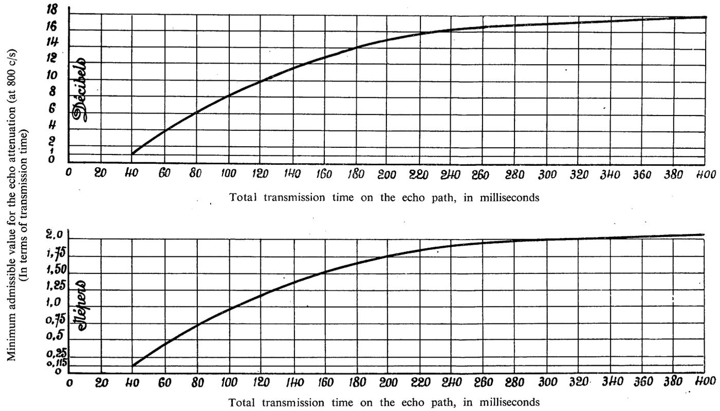
FIGURE 2. — Curve giving the minimum admissible value for the zero attenuation for circuits fitted with echo suppressors (sensitivity referred to echo relative level: 30 db)
