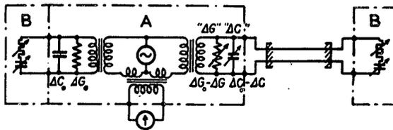
FIGURE 3. — Admittance deviation measuring set
