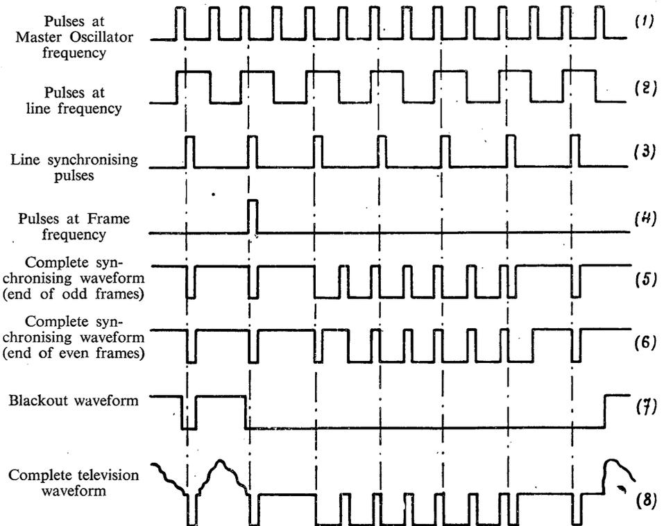
FIGURE 2. — *Output waves from the various television waveform generators units*
