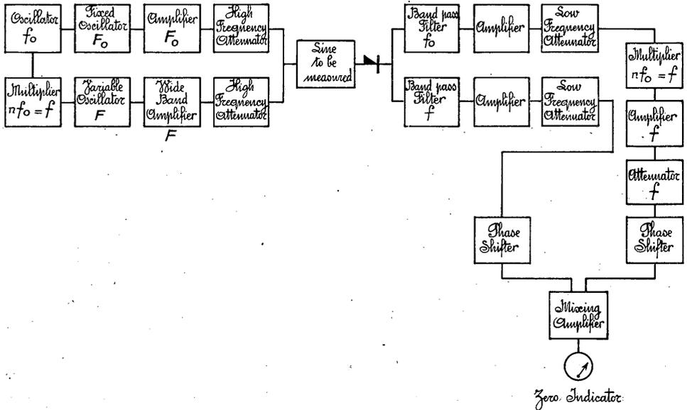
FIGURE 1. — Measurement of the differences of group delay on a line
