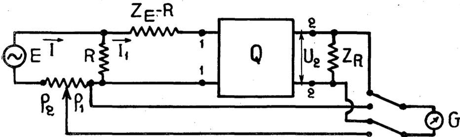
FIGURE 3. — *Measurement of loss by the Z — R method*
