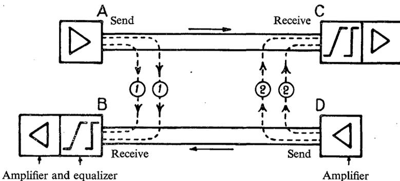
FIGURE 1. — Near-end crosstalk between cables
