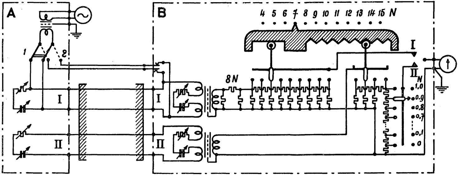
FIGURE 4. — Crosstalk measuring set used in Mexico by the Empresa de Teléfonos Ericsson
