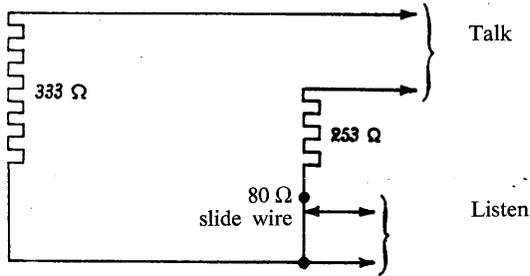
FIGURE 25. — Schematic of audio crosstalk meter
