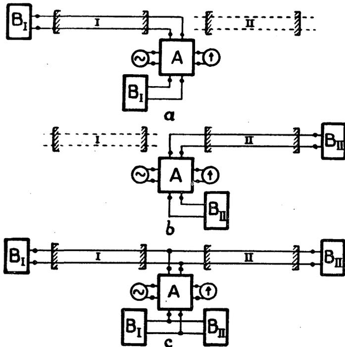
FIGURE 4. — Admittance deviation measuring set
