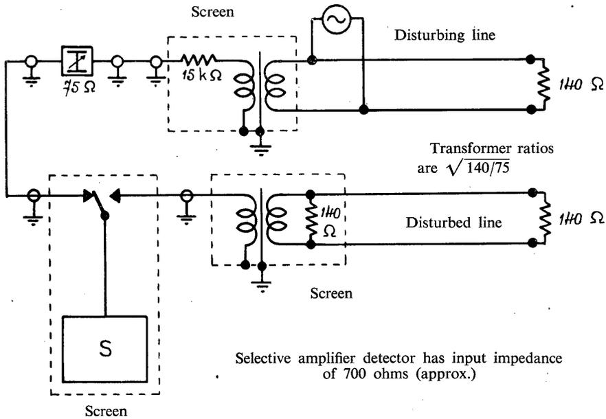
FIGURE 26. — Near-end crosstalk measurement between symmetrical pairs for carrier systems
