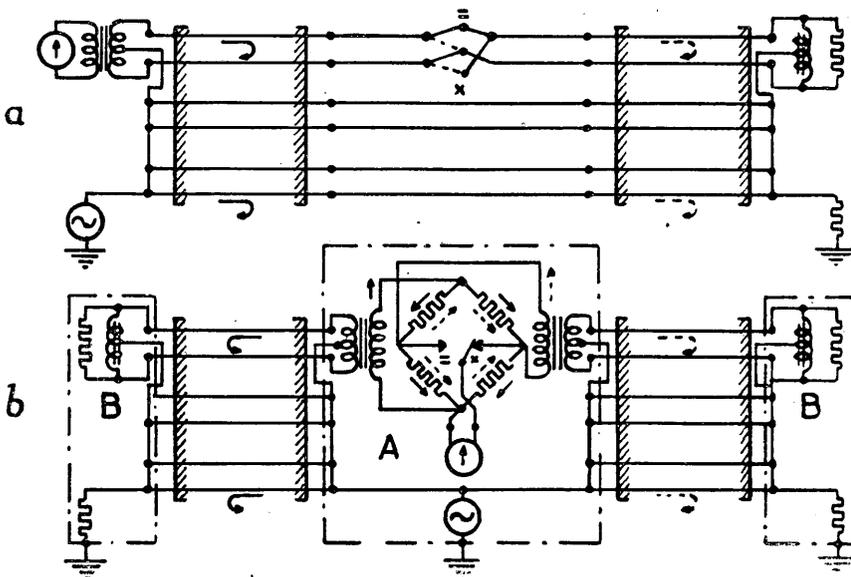
FIGURE 5. — *Unbalance measuring set*
