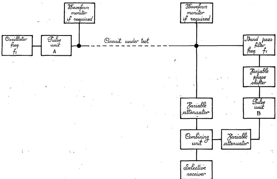
FIGURE 1. — Method proposed for measuring "attenuation-frequency" and "phase delay-frequency" characteristics of a circuit
