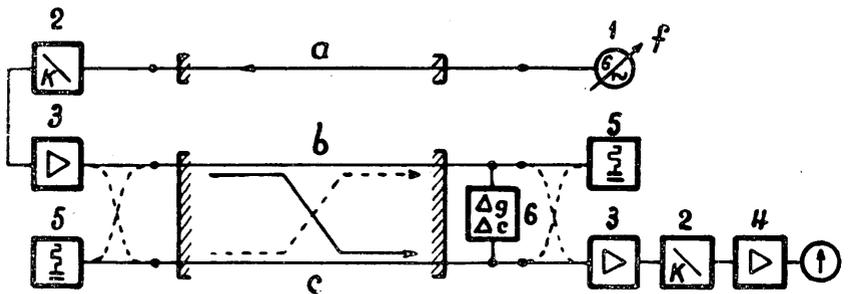
FIGURE 3. — Arrangement of the instruments used to compensate far-end crosstalk on a repeater section
