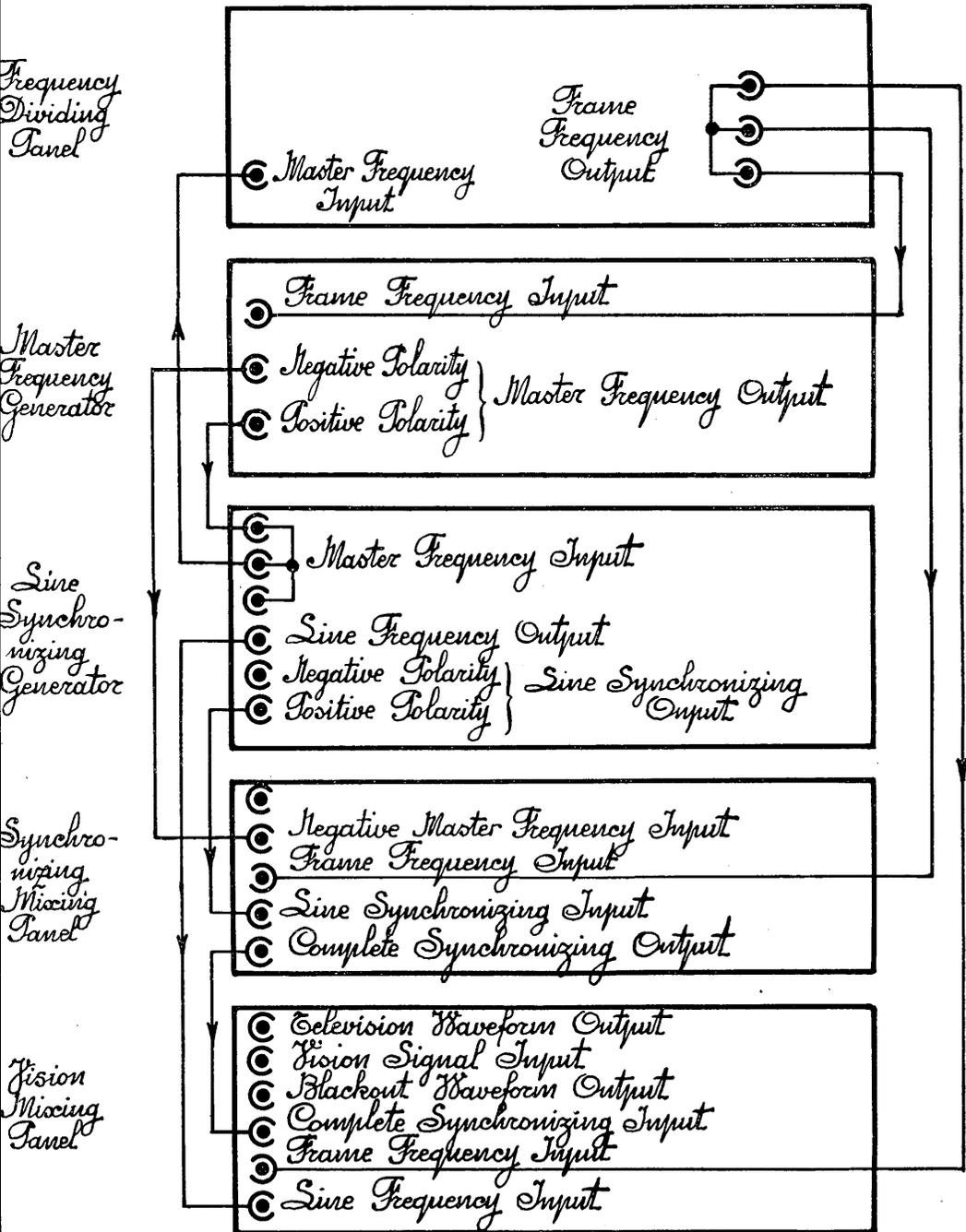
FIGURE 1. — Inter panel connections of the television waveform generator
