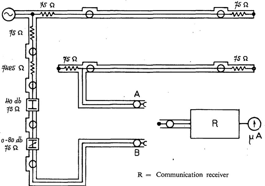
FIGURE 28. — Near-end crosstalk measurement between coaxial pairs
