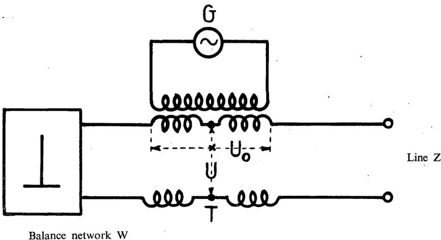
FIGURE 17. — Return-Loss Measuring set
