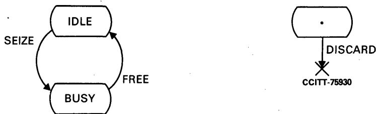
FIGURE D-133 Example of a separated state overview diagram
