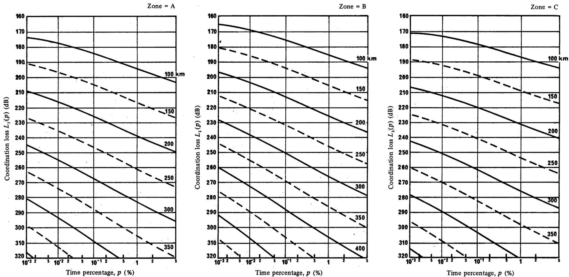
FIGURE 38 – Coordination loss  $L_1(p)$ , dB as a function of time percentage,  $p$ , for isopleths of distance in km
