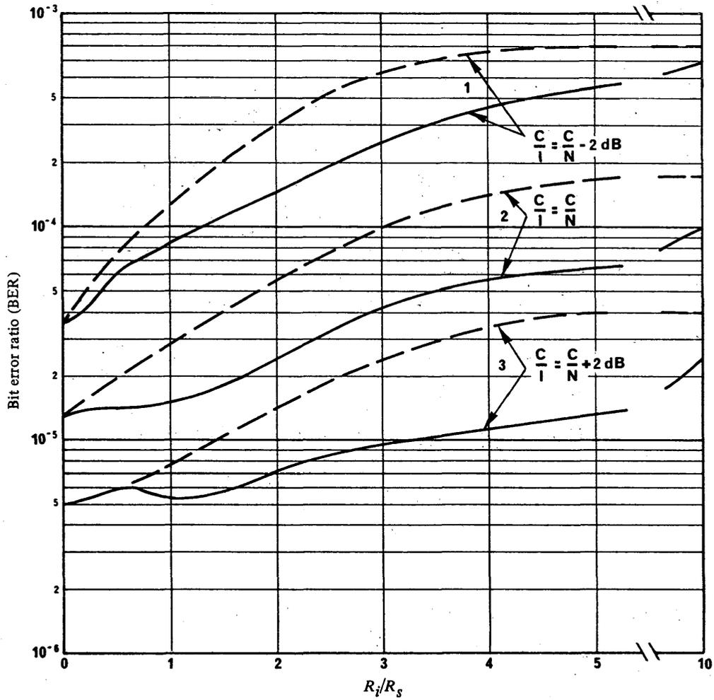
FIGURE 11 - Coherent 4-PSK demodulator error ratio as a function of  $R_i/R_s$  transmission speed ratio
