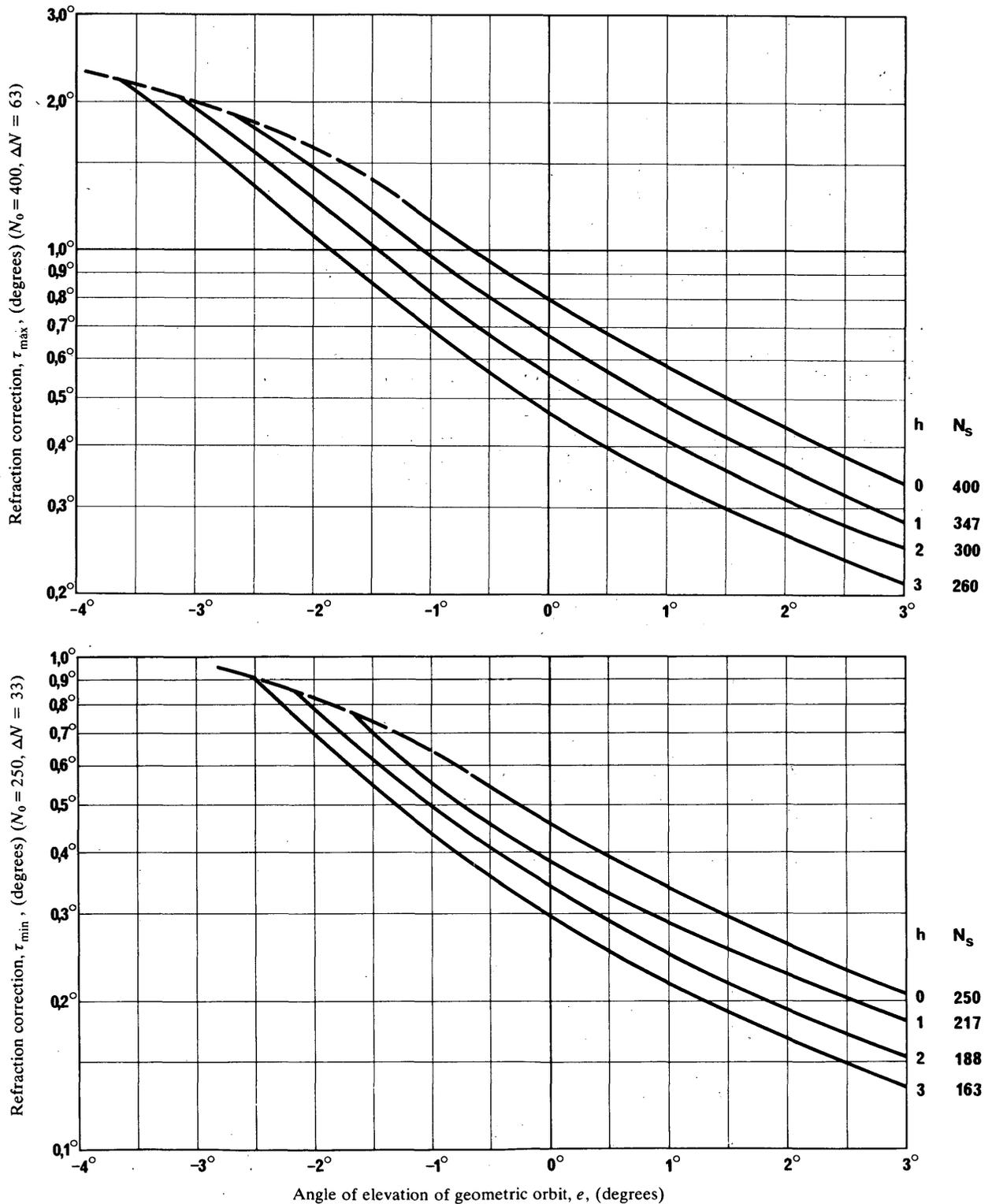
FIGURE 7 - Refraction correction for angle  $e$
