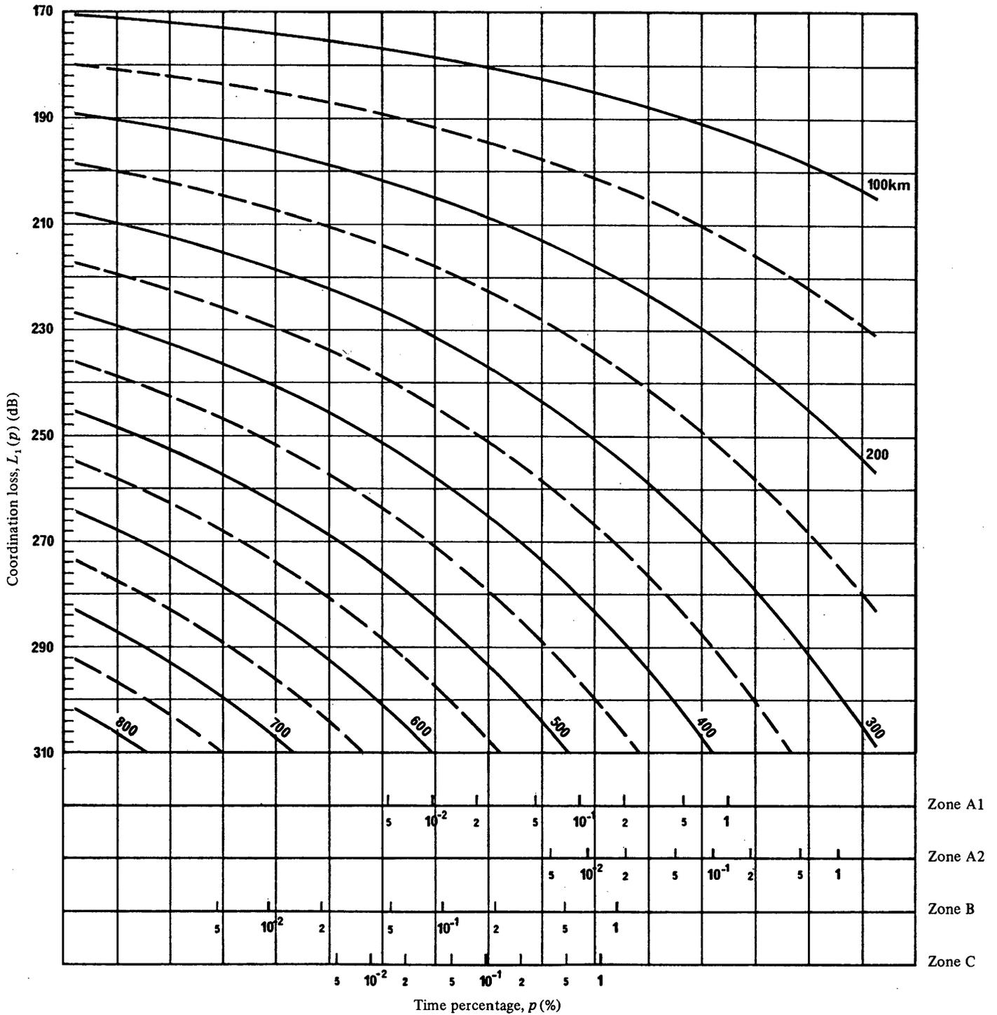
FIGURE 11 – Coordination loss as a function of time percentage,  $p$ , for isopleths of distance;  $f = 40$  GHz
