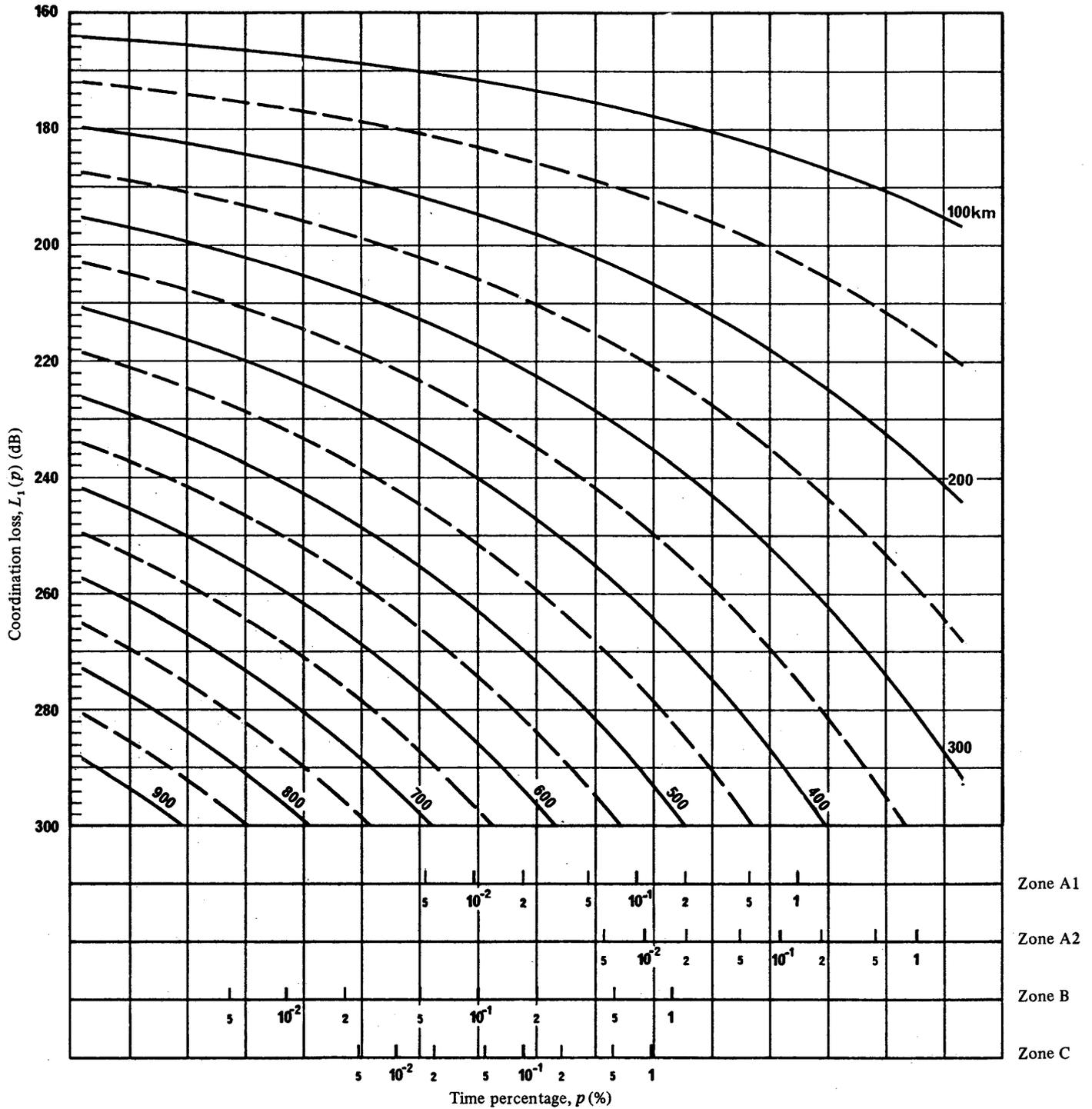
FIGURE 10 – Coordination loss as a function of time percentage,  $p$ , for isopleths of distance;  $f = 28$  GHz
