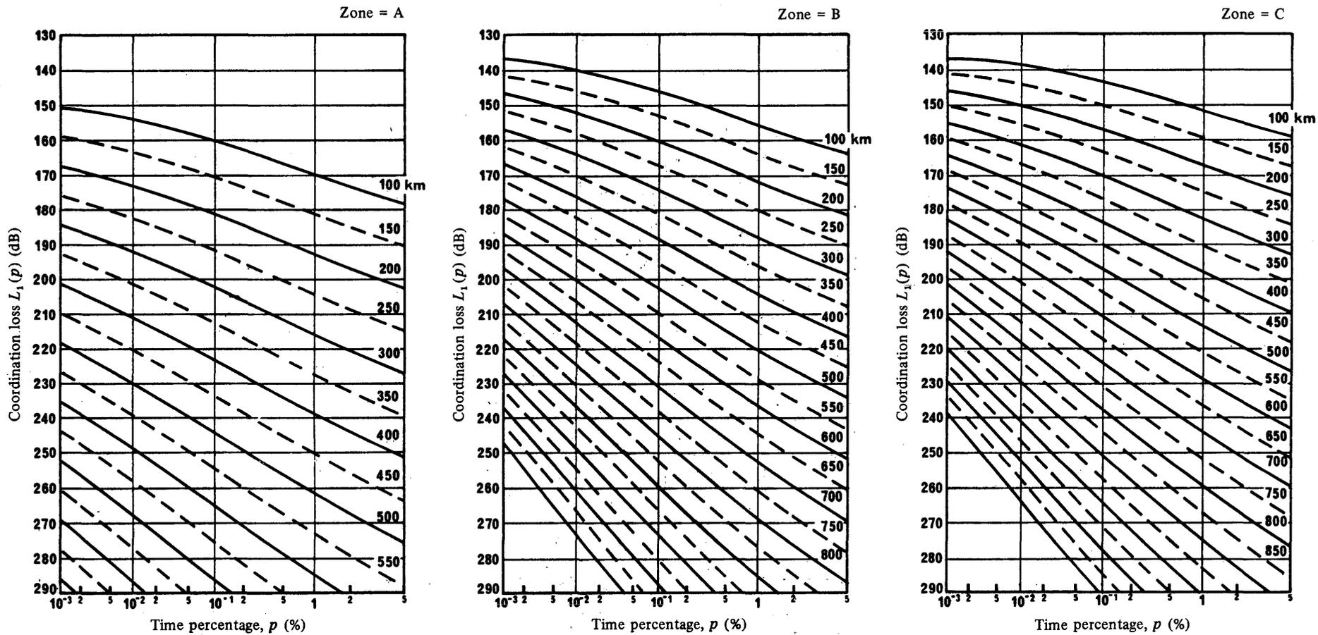
FIGURE 34 – Coordination loss  $L_1(p)$ , dB as a function of time percentage,  $p$ , for isopleths of distance in km
