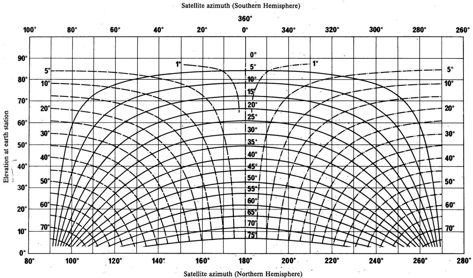
FIGURE 24— *Position arcs of geostationary satellites*
