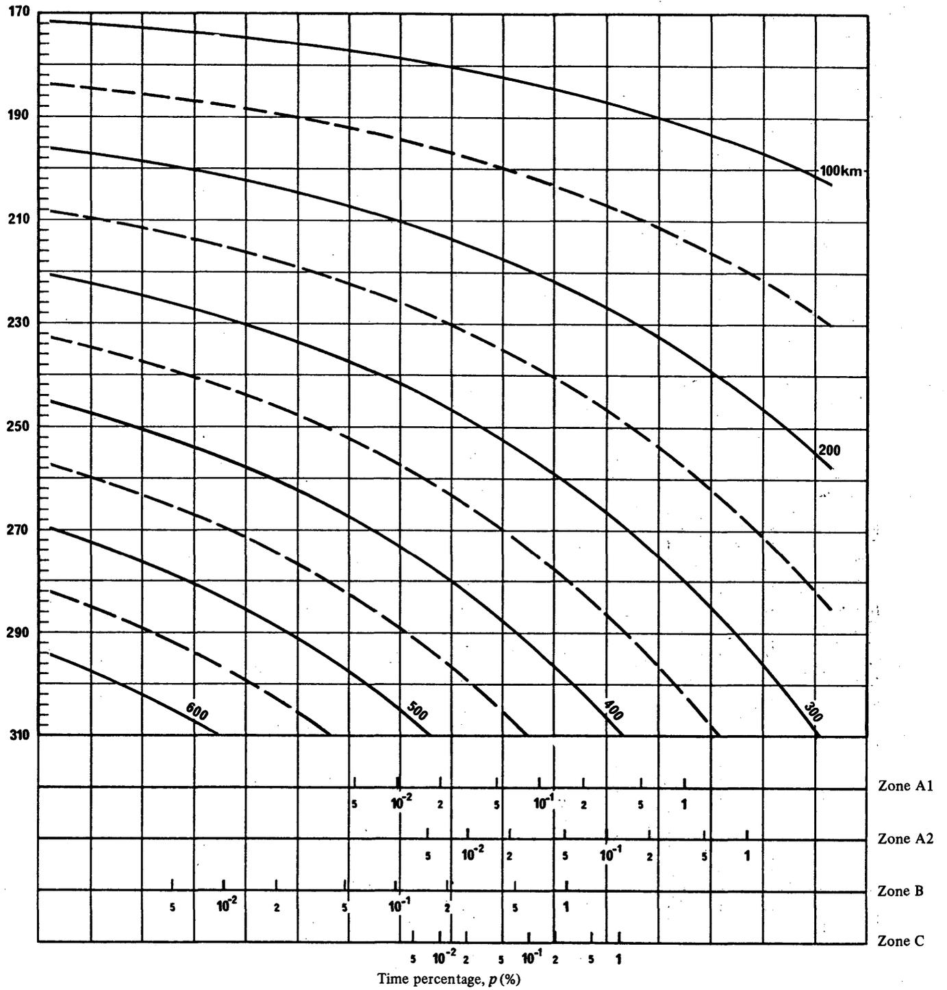
FIGURE 9 - Coordination loss as a function of time percentage,  $p$ , for isopleths of distance;  $f = 22.3$  GHz
