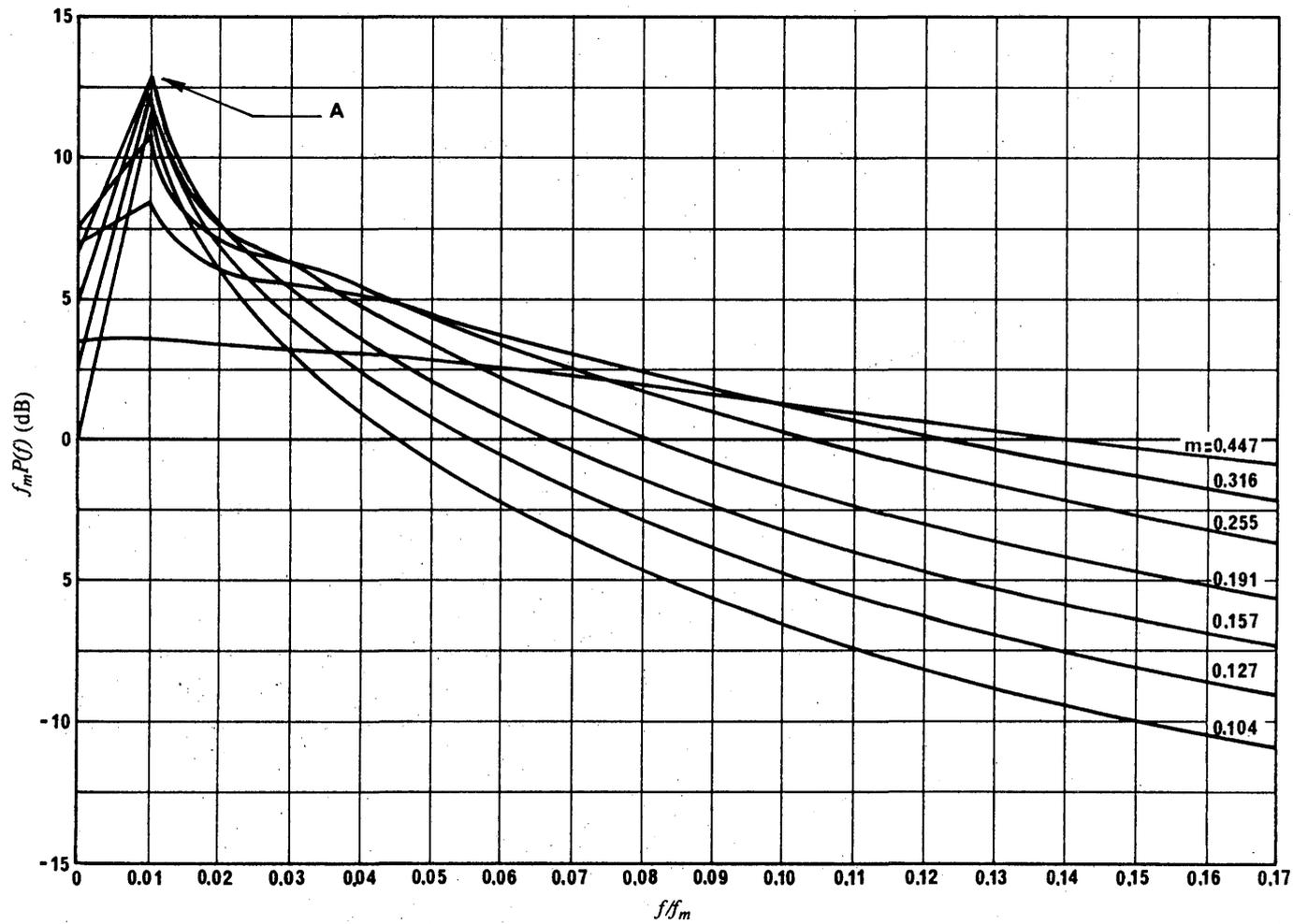
FIGURE 9g – Normalized power spectral densities for various modulation indices and for  $\epsilon = 0.01$
