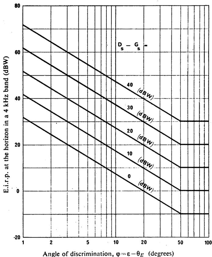
FIGURE 1 - *E.i.r.p.* towards the horizon as a function of the angle of discrimination,  $\phi$
