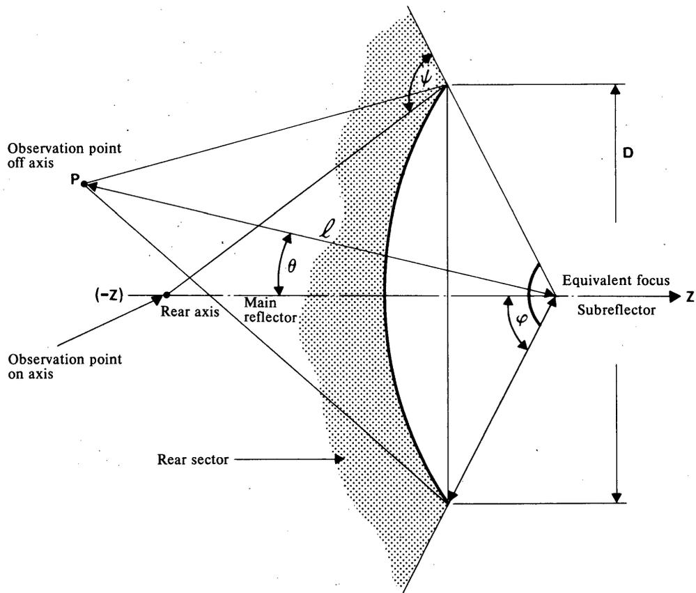
FIGURE 1 - Geometry for calculation of coupling factor between a large Cassegrain antenna and isotropic antenna located in its geometrical shadow
