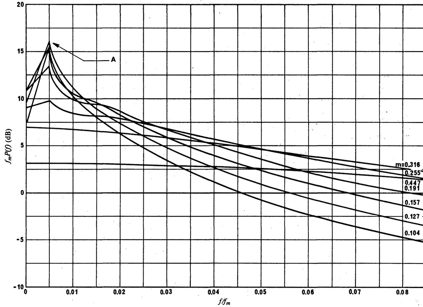
FIGURE 9f – Normalized power spectral densities for various modulation indices and for  $\epsilon = 0.005$
