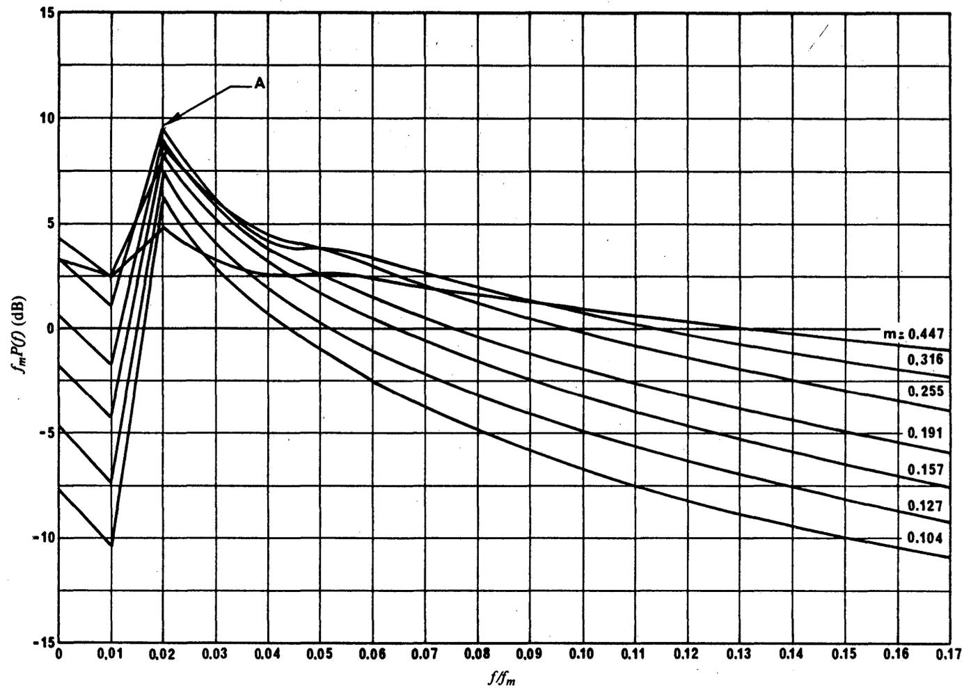
FIGURE 9h - Normalized power spectral densities for various modulation indices and for  $\epsilon = 0.02$
