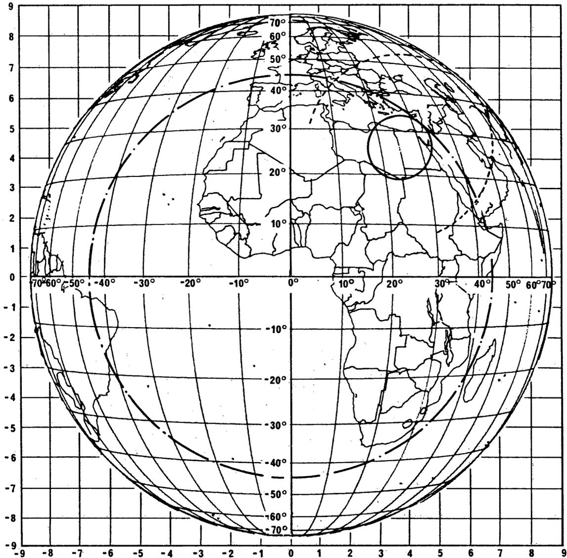
FIGURE 1 – Permissible range for RBW with 2° beams avoiding additional sharing constraints with terrestrial services
