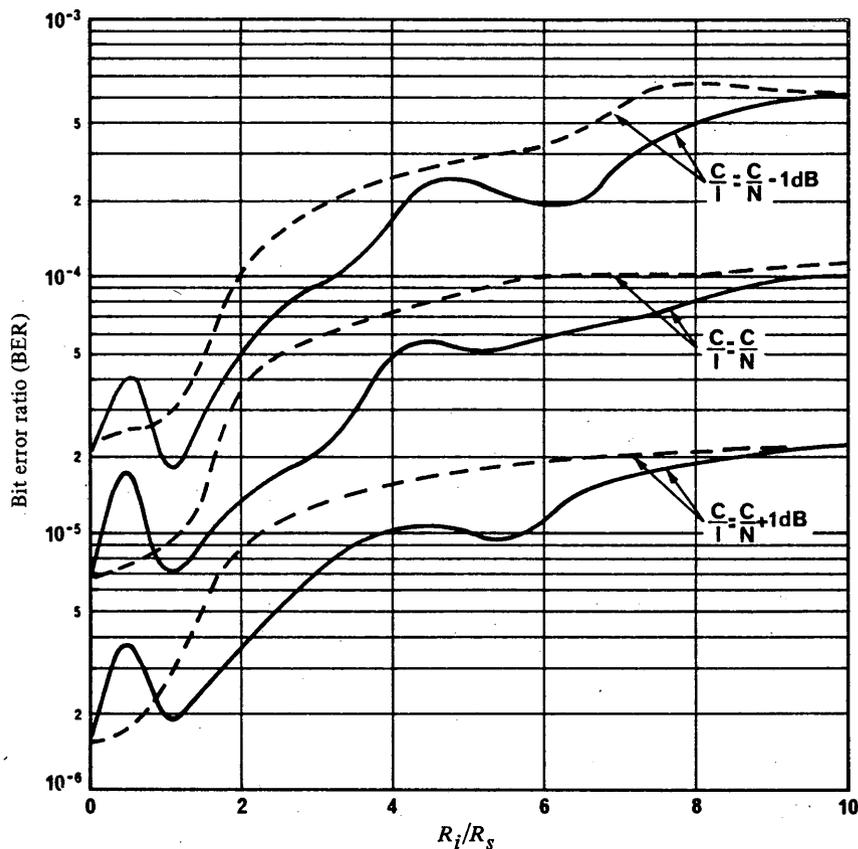
FIGURE 12 – Error ratio at convolution code decoder output as a function of  $R_i/R_s$  transmission speed ratio
