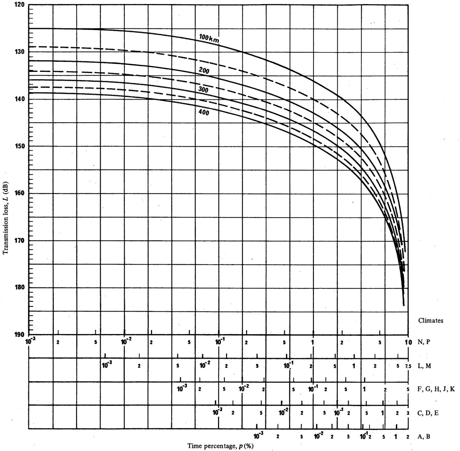
FIGURE 15 – Transmission loss as a function of time percentage,  $p$ , for the different rain climates with hydrometeor scatter distance as a parameter;  $f = 8$  GHz
