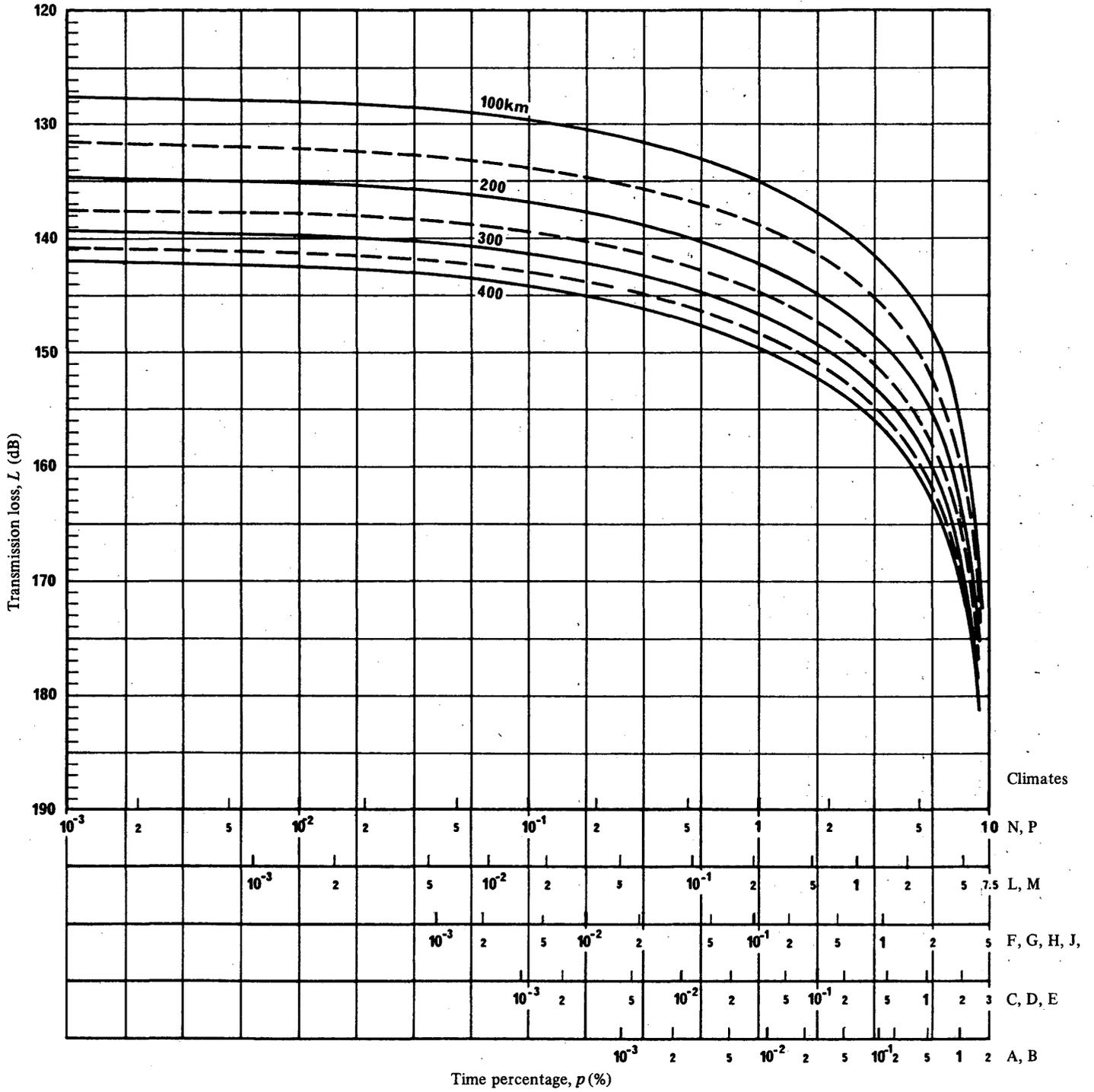
FIGURE 17 – Transmission loss as a function of time percentage,  $p$ , for the different rain climates with hydrometeor scatter distance as a parameter;  $f = 14$  GHz
