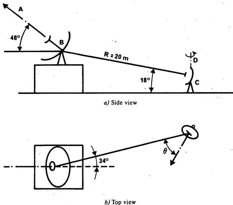
FIGURE 4 - Antenna location for coupling measurement ( $R = 20\text{ m}$ )
