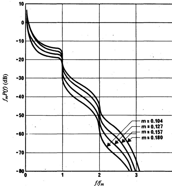
FIGURE 9a - Normalized power spectral densities for various modulation indices
