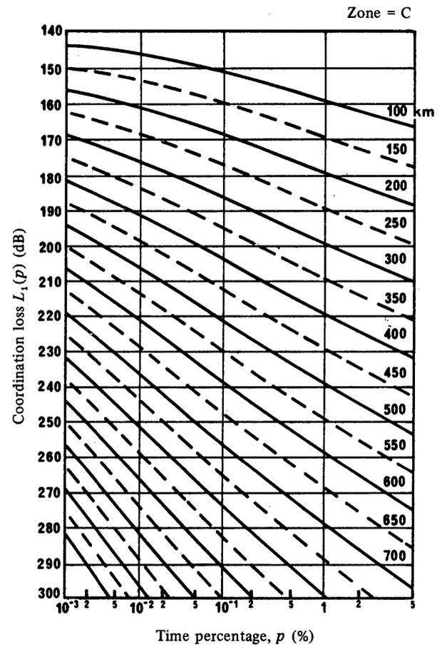
FIGURE 36 – Coordination loss  $L_1(p)$ , dB as a function of time percentage,  $p$ , for isopleths of distance in km
