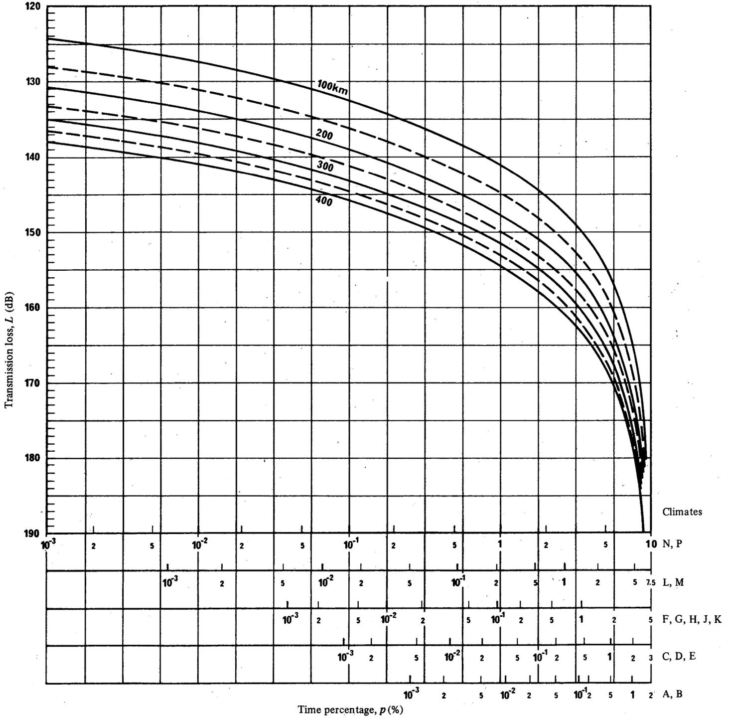
FIGURE 13 - Transmission loss as a function of time percentage,  $p$ , for the different rain climates with hydrometeor scatter distance as a parameter;  $f = 4$  GHz
