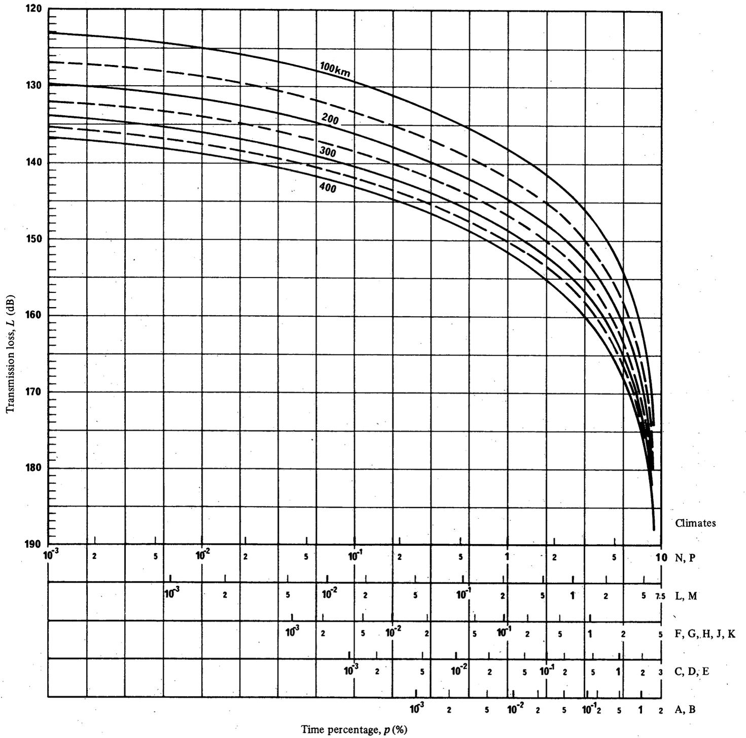
FIGURE 14 – Transmission loss as a function of time percentage,  $p$ , for the different rain climates with hydrometeor scatter distance as a parameter;  $f = 6$  GHz
