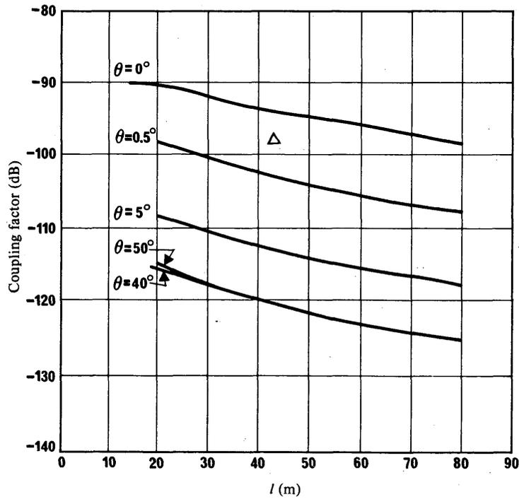
FIGURE 2a - Calculated coupling factor between 32.0 m antenna and isotropic antenna located in its rear sector (6.0 GHz)
