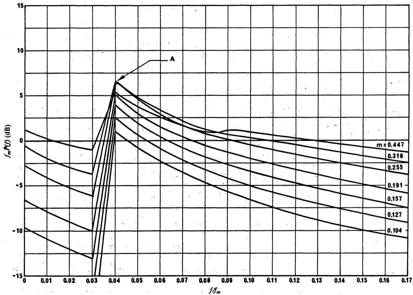
FIGURE 9i - Normalized power spectral densities for various modulation indices and for  $\epsilon = 0.04$
