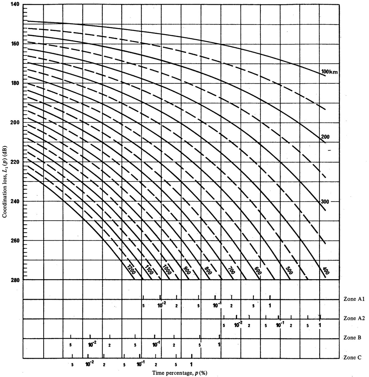
FIGURE 6 – Coordination loss as a function of time percentage,  $p$ , for isopleths of distance;  $f = 12$  GHz
