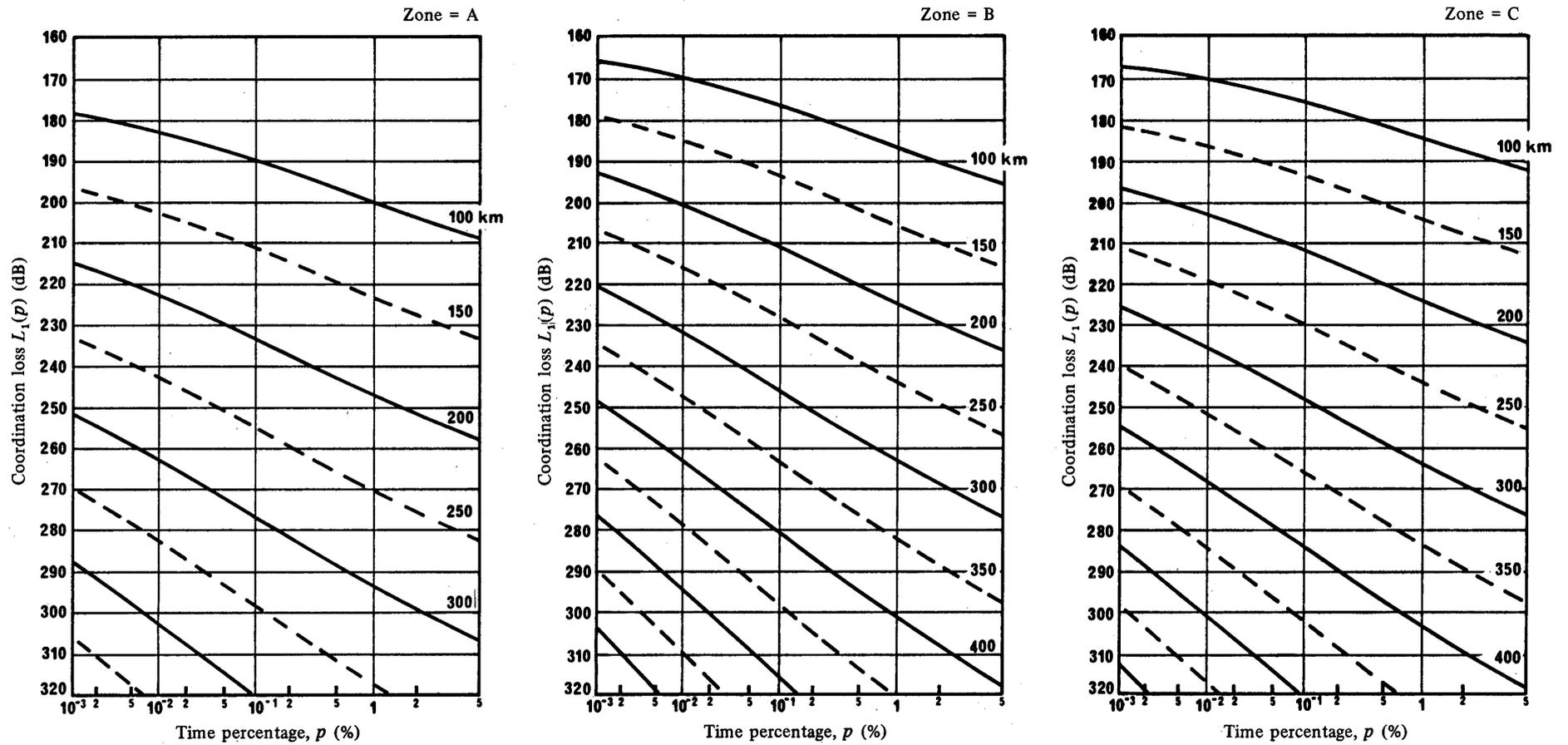
FIGURE 40 – Coordination loss  $L_1(p)$ , dB as a function of time percentage,  $p$ , for isopleths of distance in km
