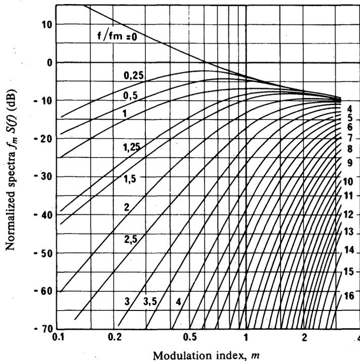
FIGURE 1 - Normalized spectral density of FDM-FM signals
