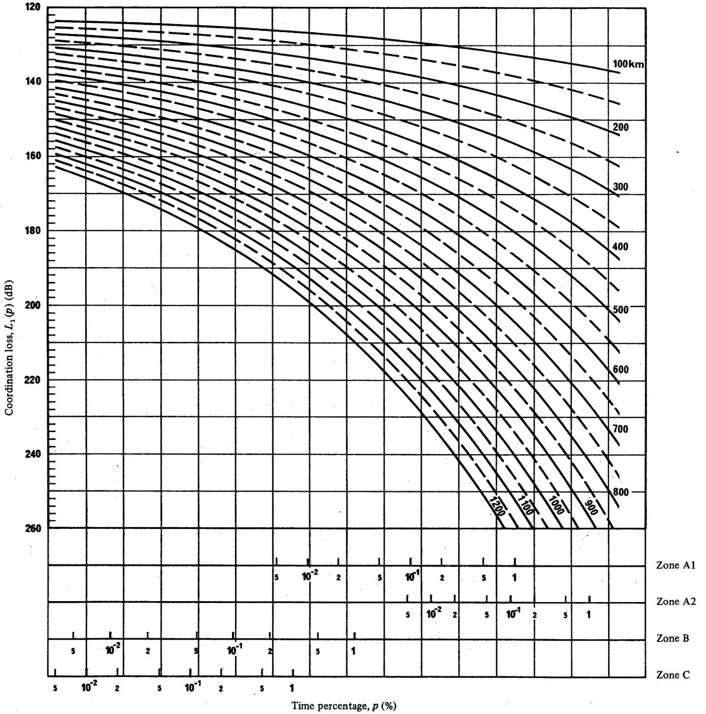
FIGURE 2 – Coordination loss as a function of time percentage,  $p$ , for isopleths of distance;  $f = 1$  GHz
