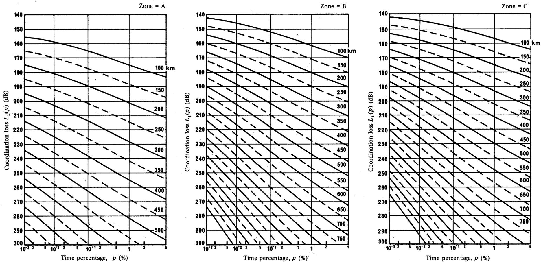
FIGURE 35 – Coordination loss  $L_1(p)$ , dB as a function of time percentage,  $p$ , for isopleths of distance in km
