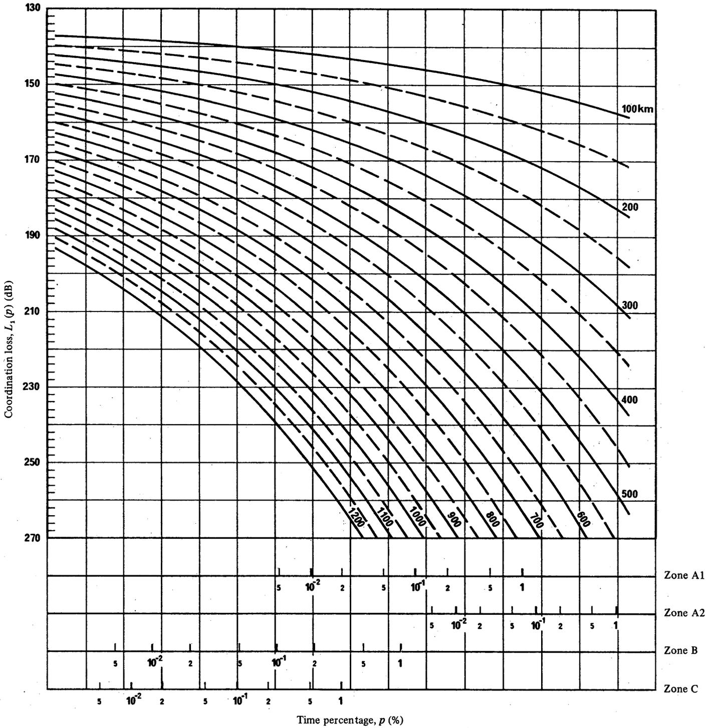
FIGURE 3 – Coordination loss as a function of time percentage,  $p$ , for isopleths of distance;  $f = 4$  GHz
