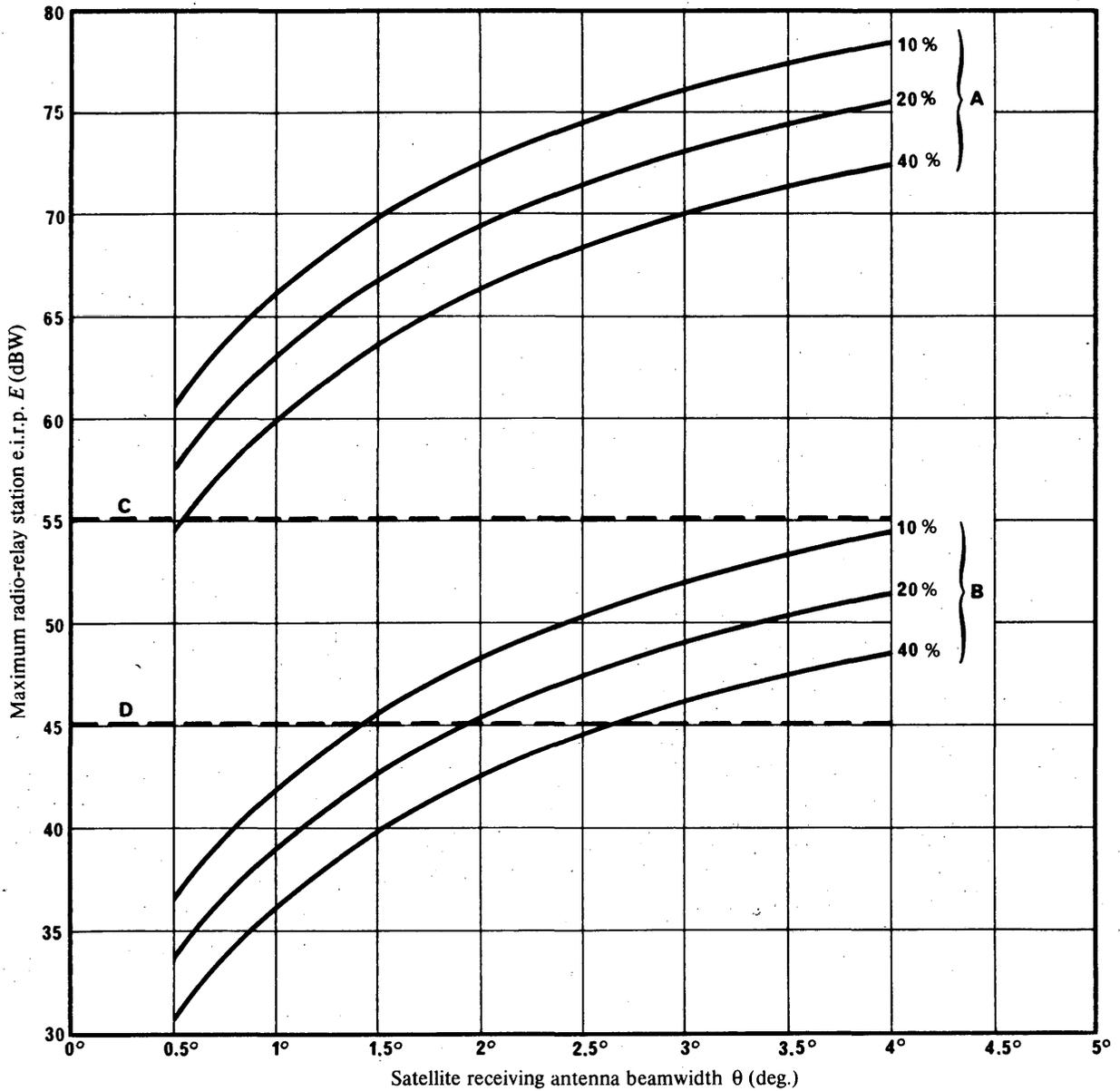
FIGURE 1 - Maximum terrestrial radio-relay station e.i.r.p. ( $E$ ), without exceeding interference criteria, for a satellite receiving antenna having a beamwidth  $\theta$ , the beam being directed towards the horizon
