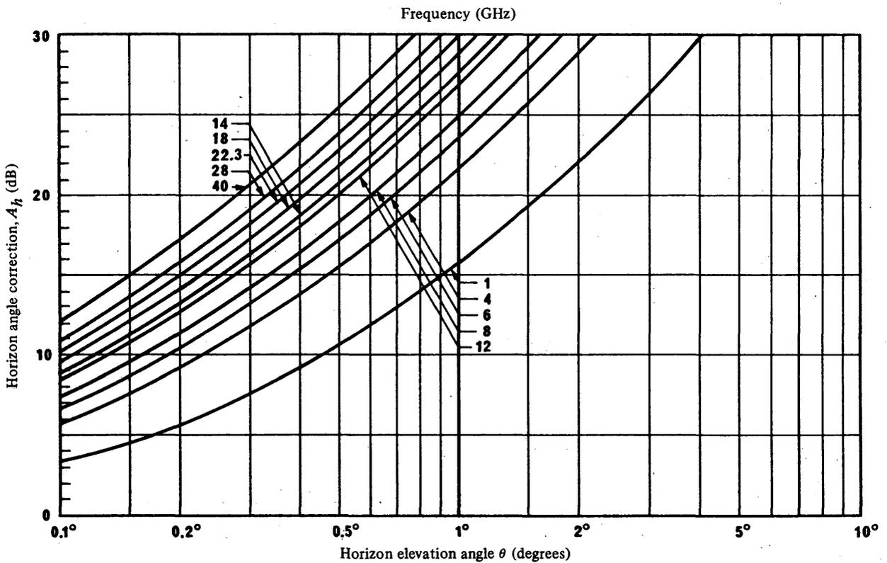
FIGURE 1 - *Horizon angle correction  $A_h$  as a function of horizon angle and frequency*
