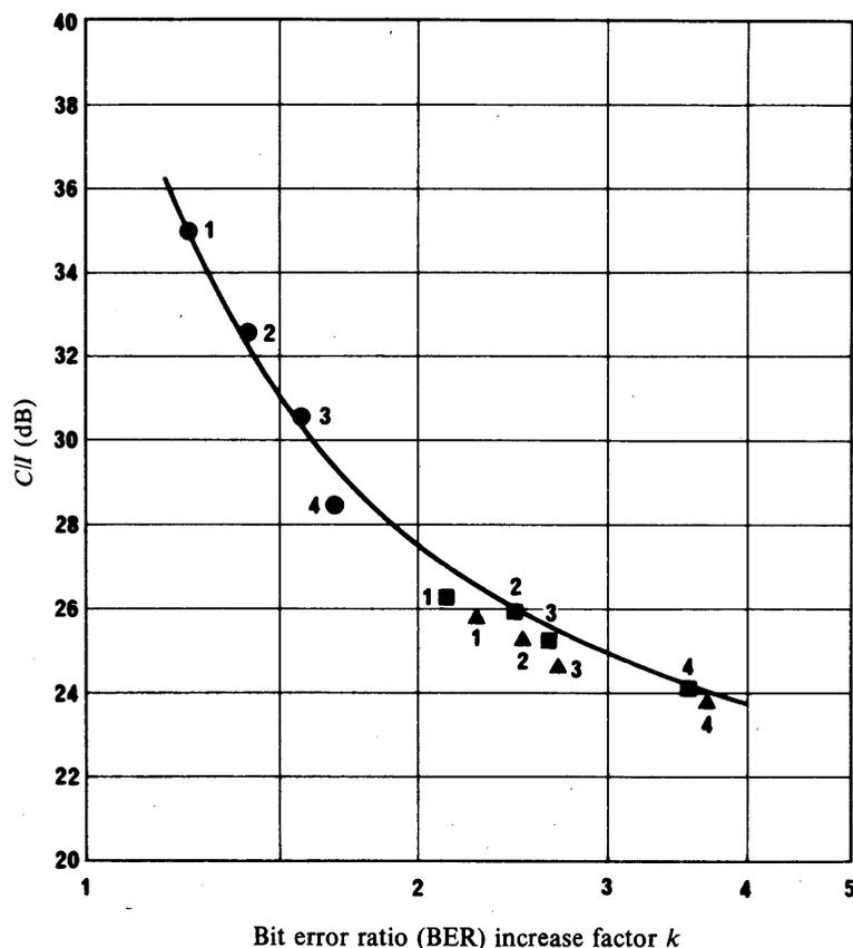
FIGURE 1 –  $C/I$  versus  $k$  for various DEQPSK transmission modes.
