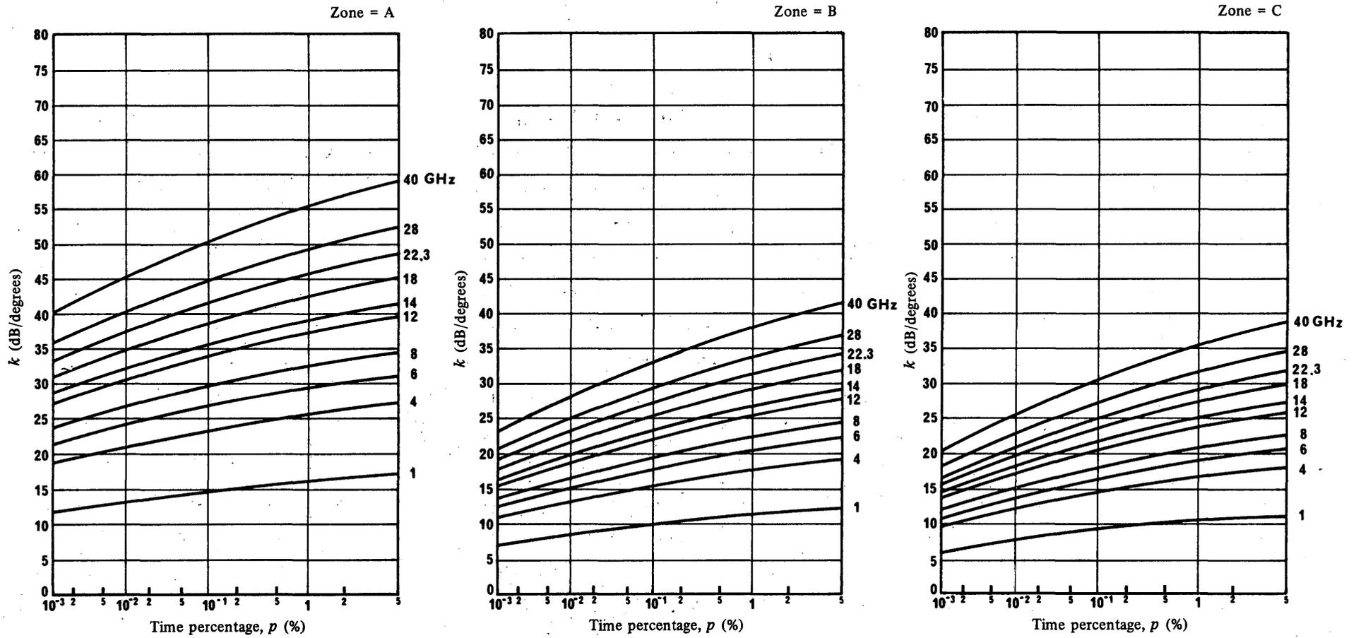
FIGURE 30 – Factor  $k$  in dB/degrees as a function of time percentage,  $p$ , for isopleths of frequency in GHz
