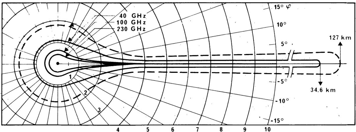
FIGURE 1 - Necessary separation for terrestrial receiving station
