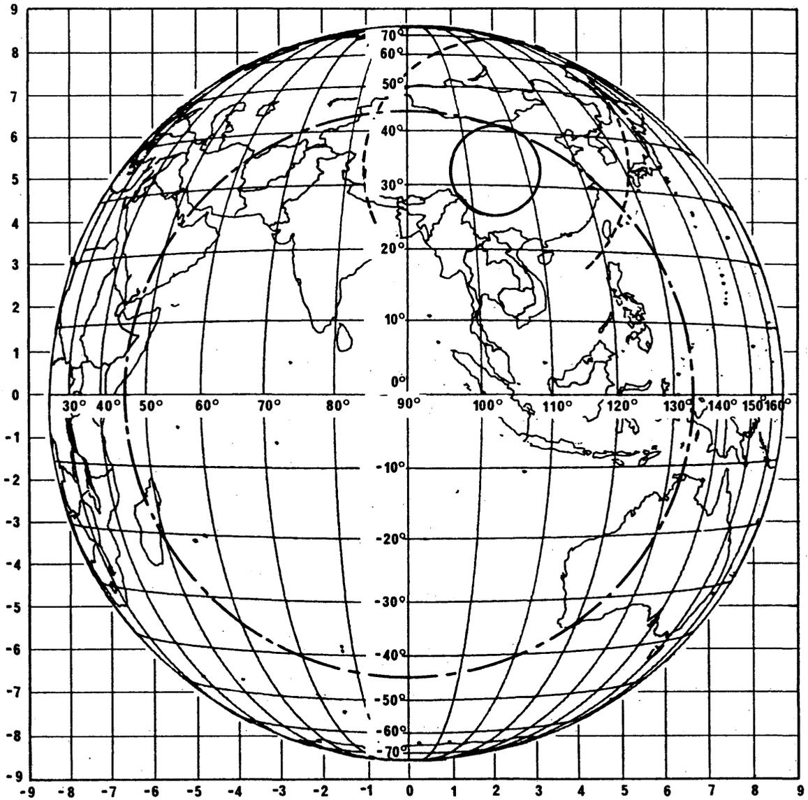
FIGURE 3 – *Permissible range for RBW with 2° beams avoiding additional sharing constraints with terrestrial services*
