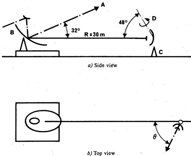
FIGURE 5 - Antenna location for coupling measurement ( $R = 30\text{ m}$ )
