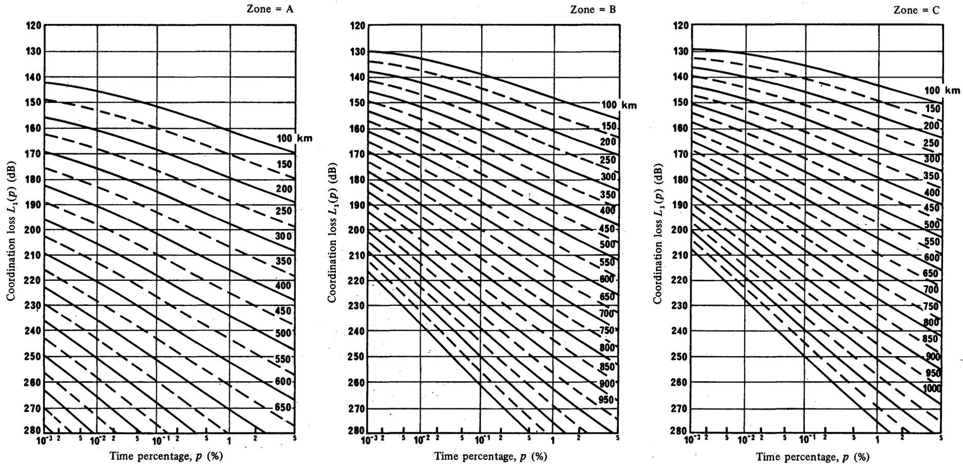
FIGURE 32 – Coordination loss  $L_1(p)$ , dB as a function of time percentage,  $p$ , for isopleths of distance in km
