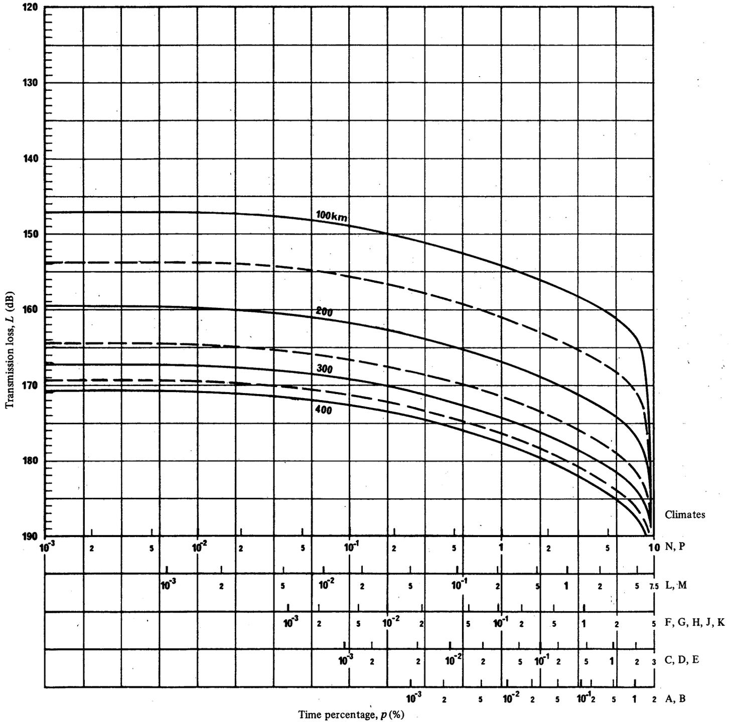
FIGURE 21 - Transmission loss as a function of time percentage,  $p$ , for the different rain climates with hydrometeor scatter distance as a parameter;  $f = 40$  GHz
