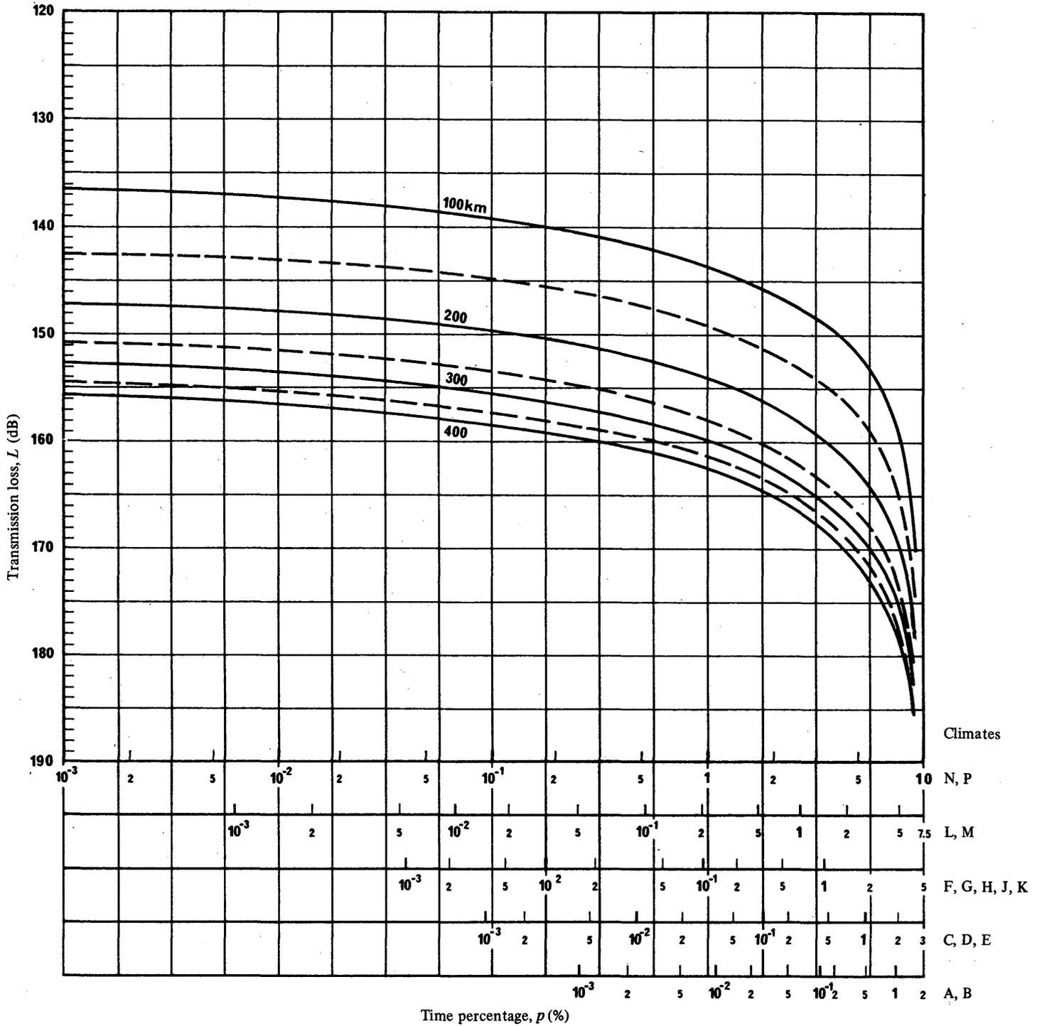
FIGURE 20 - Transmission loss as a function of time percentage,  $p$ , for the different rain climates with hydrometeor scatter distance as a parameter;  $f = 28$  GHz
