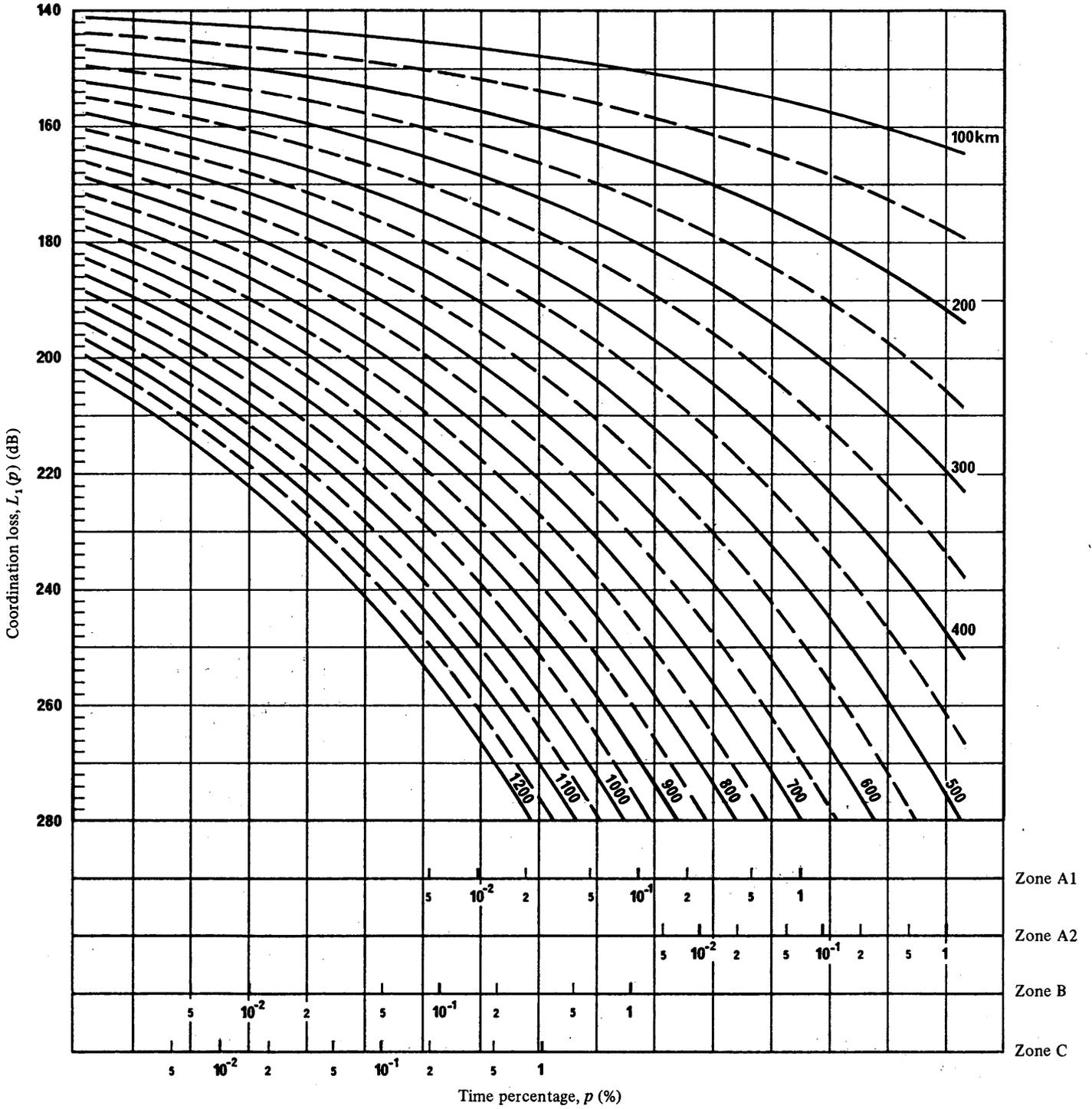
FIGURE 4 – Coordination loss as a function of time percentage,  $p$ , for isopleths of distance;  $f = 6$  GHz
