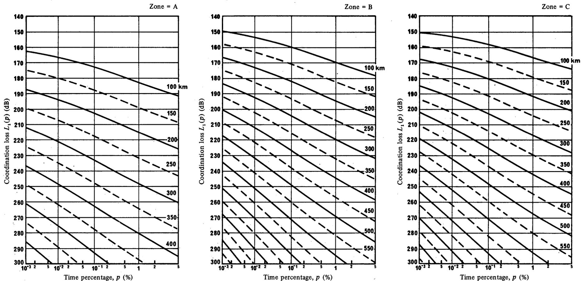
FIGURE 37 – Coordination loss  $L_1(p)$ , dB as a function of time percentage,  $p$ , for isopleths of distance in km
