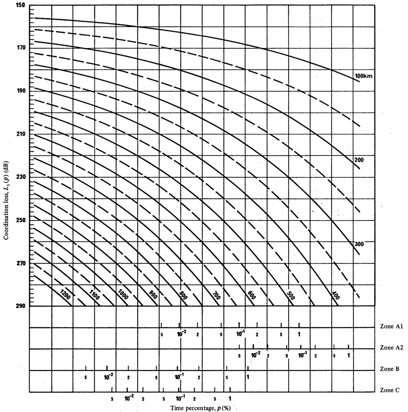
FIGURE 8 – Coordination loss as a function of time percentage,  $p$ , for isopleths of distance;  $f = 18$  GHz
