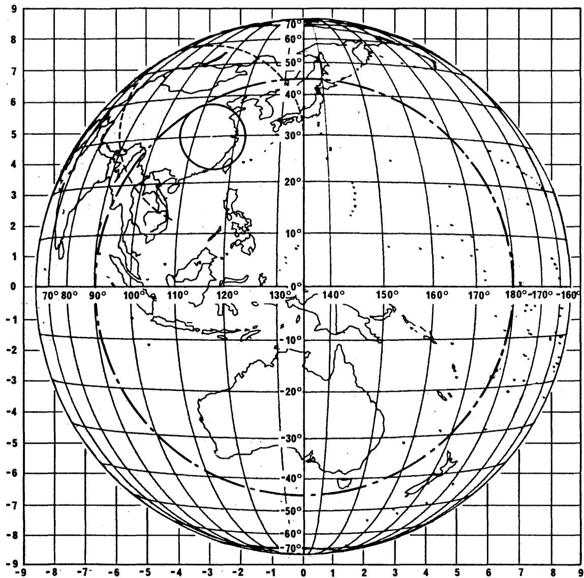
FIGURE 4 – Permissible range for RBW with  $2^\circ$  beams avoiding additional sharing constraints with terrestrial services
