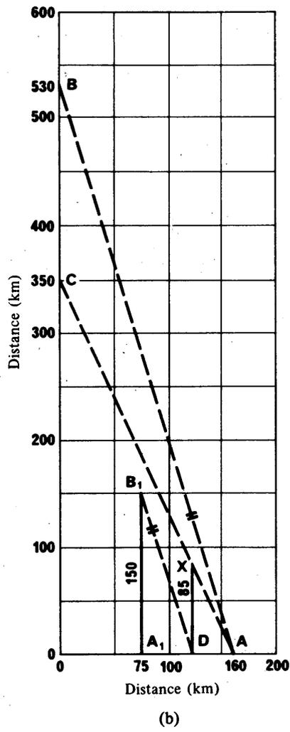
FIGURE 27 – Example of determination of coordination for mixed paths including Zones A, B and C
