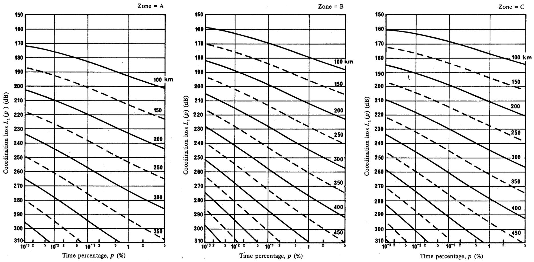
FIGURE 39 – Coordination loss  $L_1(p)$ , dB as a function of time percentage,  $p$ , for isopleths of distance in km
