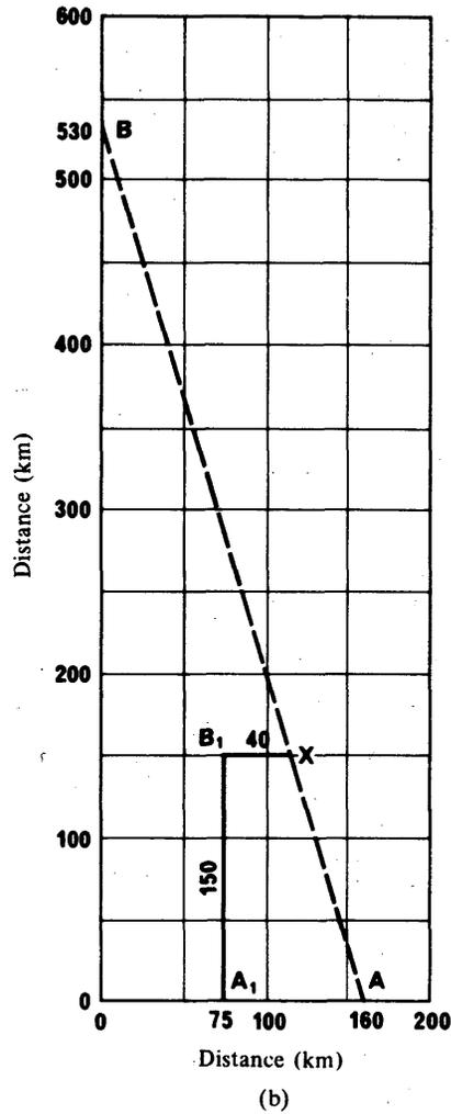
FIGURE 26 – Example of determination of coordination distance for mixed paths involving Zones A and B
