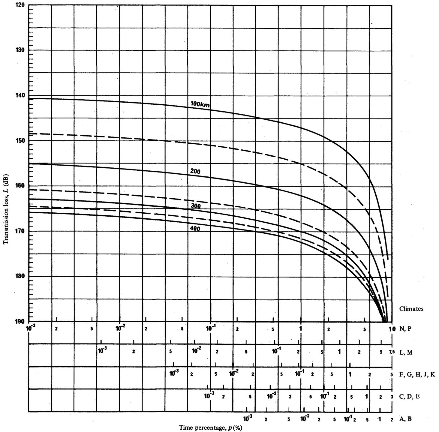
FIGURE 19 – Transmission loss as a function of time percentage,  $p$ , for the different rain climates with hydrometeor scatter distance as a parameter;  $f = 22.3$  GHz
