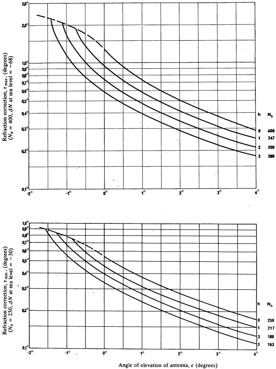
FIGURE 2 - Refraction correction for angle  $\epsilon$
