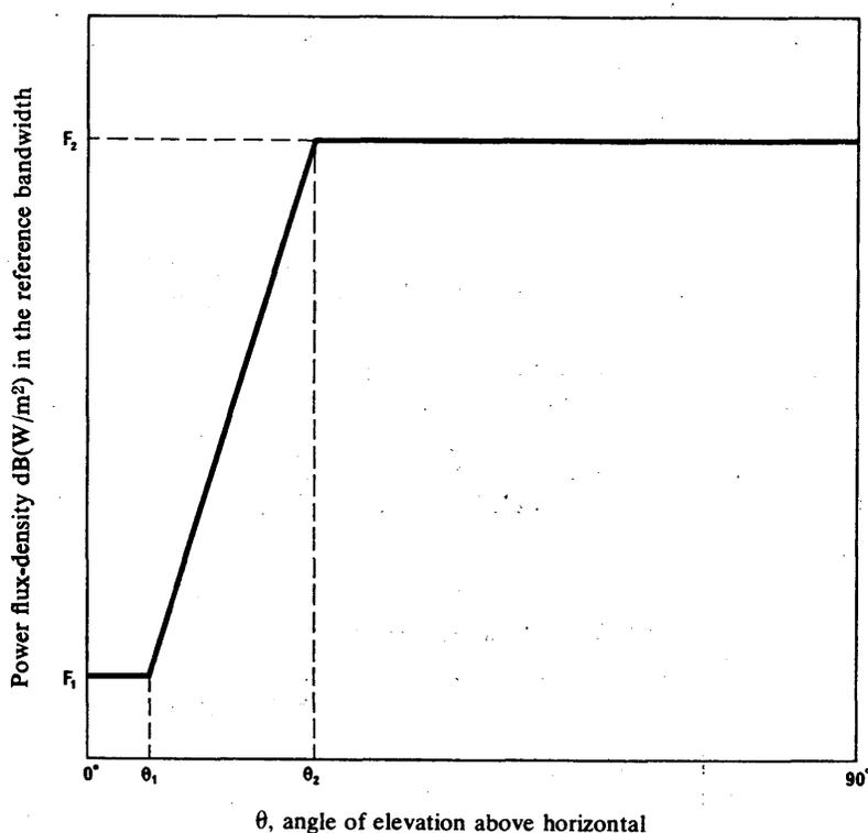
FIGURE 1 – Power flux-density limit vs. angle of arrival
