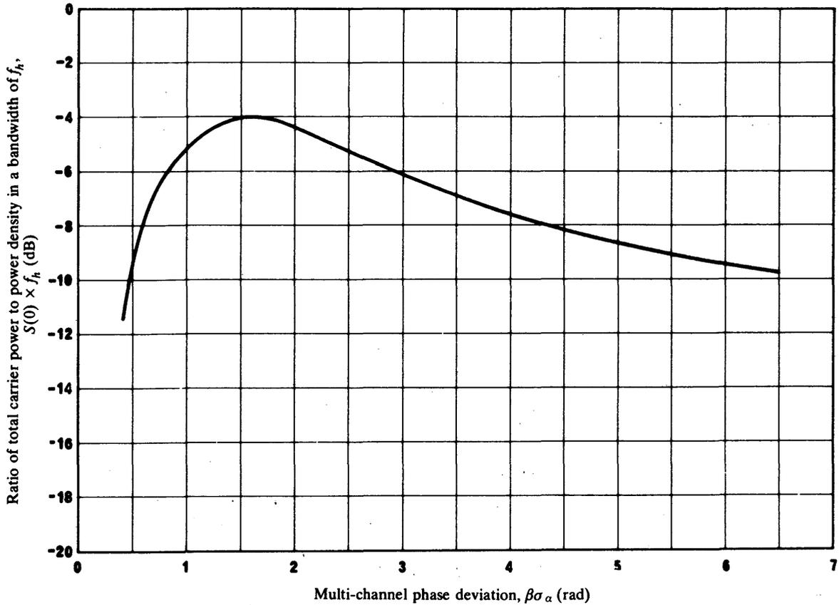
FIGURE 1 – Power density at the centre frequency of continuous power spectrum of PM carrier in a bandwidth of  $f_h$
