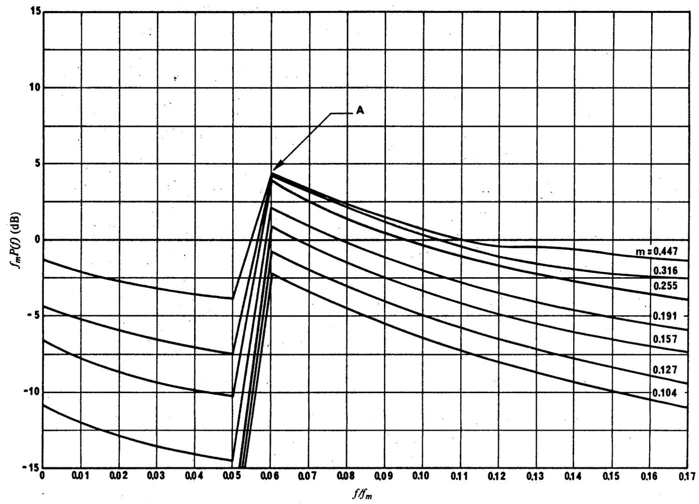
FIGURE 9j - Normalized power spectral densities for various modulation indices and for  $\epsilon = 0.06$
