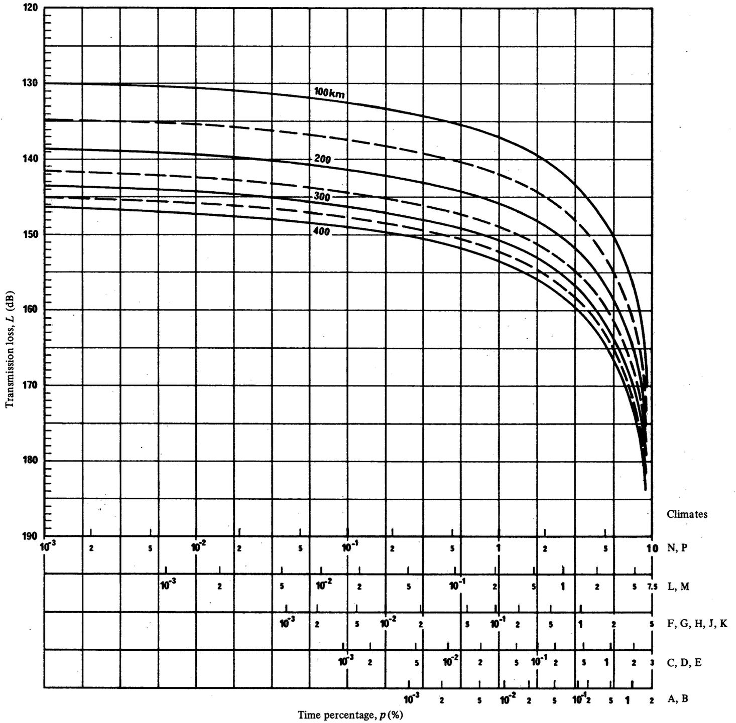
FIGURE 18 – Transmission loss as a function of time percentage,  $p$ , for the different rain climates with hydrometeor scatter distance as a parameter;  $f = 18$  GHz
