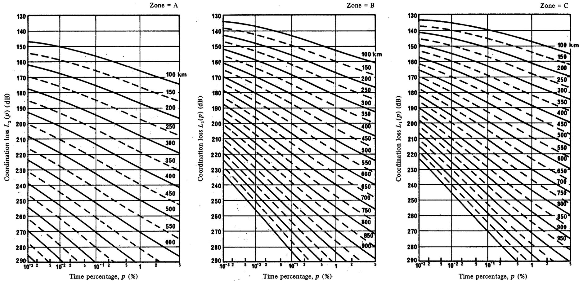
FIGURE 33 – Coordination loss  $L_1(p)$ , dB as a function of time percentage,  $p$ , for isopleths of distance in km
