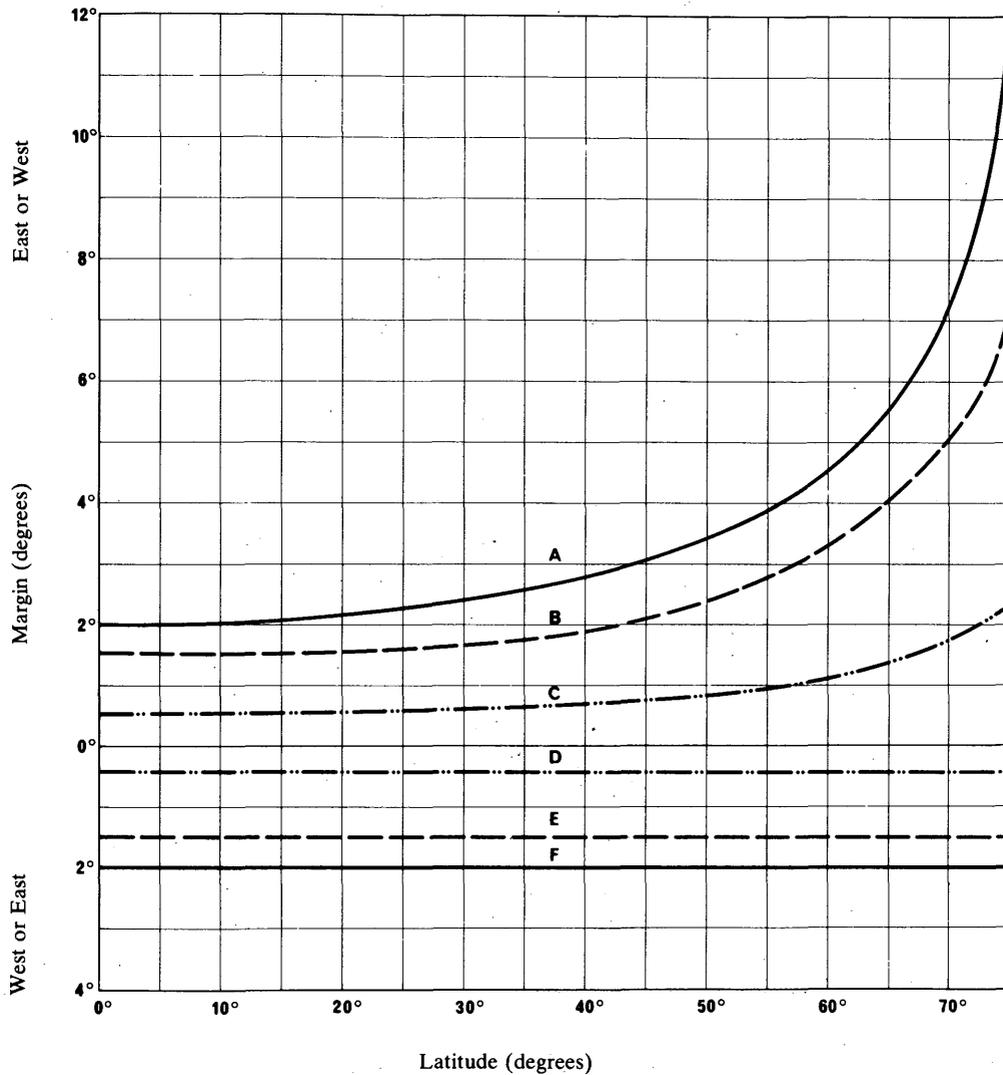
FIGURE 4 - Azimuth margins (in degrees) between the main direction of the antenna of a radio-relay system and the direction of the orbit of a geostationary satellite, to obtain a protection of  $0.5^\circ$ ,  $1.5^\circ$  or  $2^\circ$
