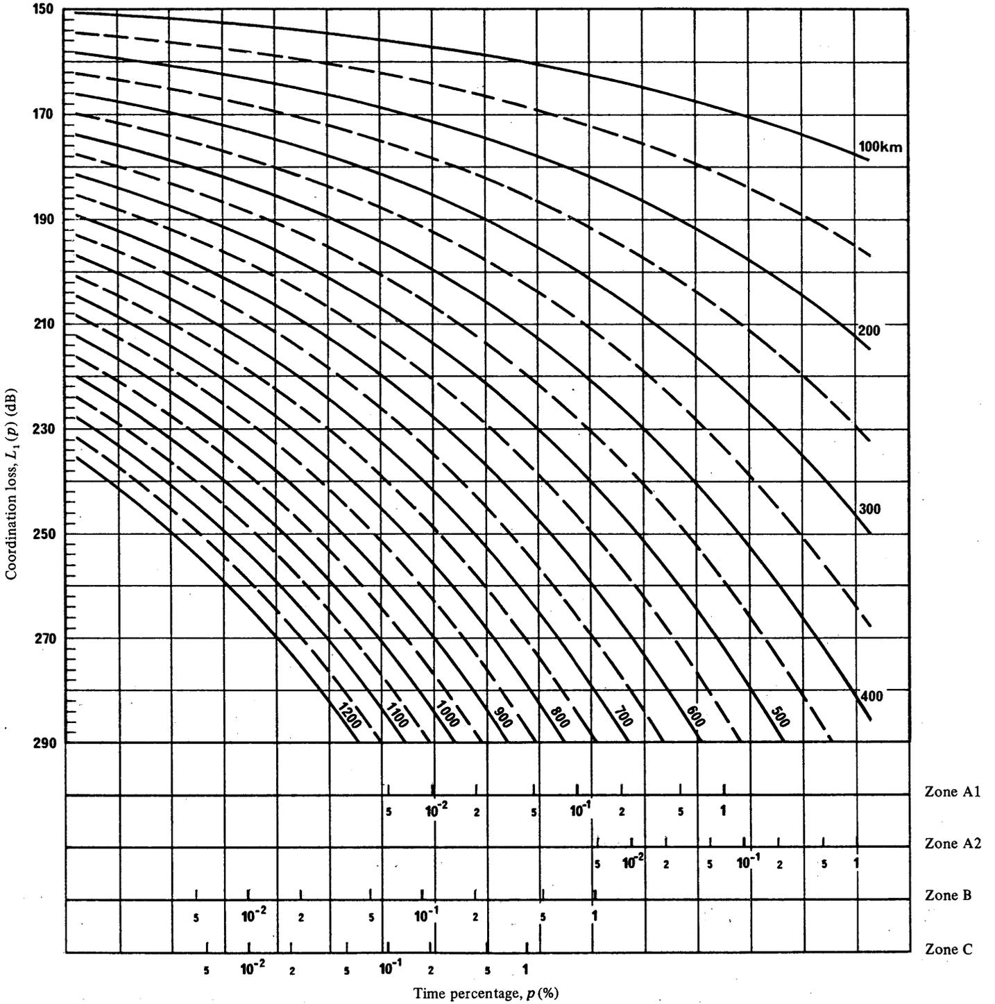
FIGURE 7 – Coordination loss as a function of time percentage,  $p$ , for isopleths of distance;  $f = 14$  GHz
