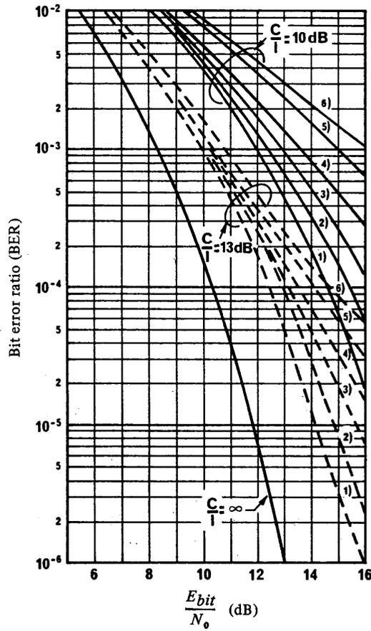
FIGURE 10 – Error ratio as a function of energy/bit-to-noise density ( $E_{bit}/N_0$ ) and carrier-to-interference  $C/I$  ratios
