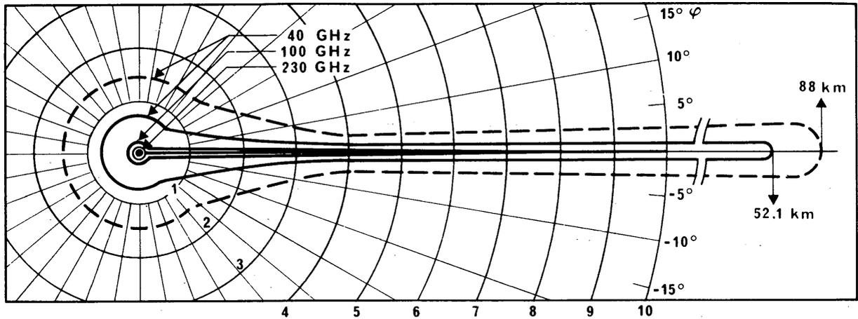
FIGURE 2 - Necessary separation for terrestrial transmitting station
