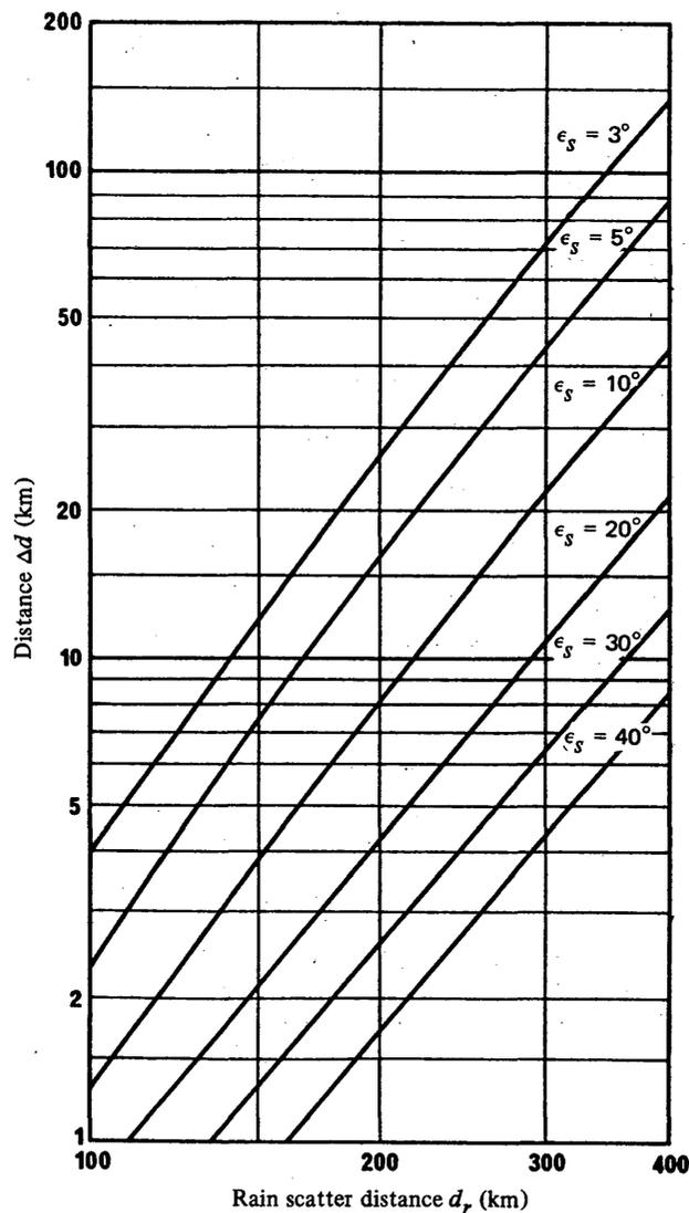
FIGURE 22 – The distance  $\Delta d$  as a function of the rain-scatter distance  $d_r$  and the earth-station antenna main beam elevation angle  $\epsilon_s$
