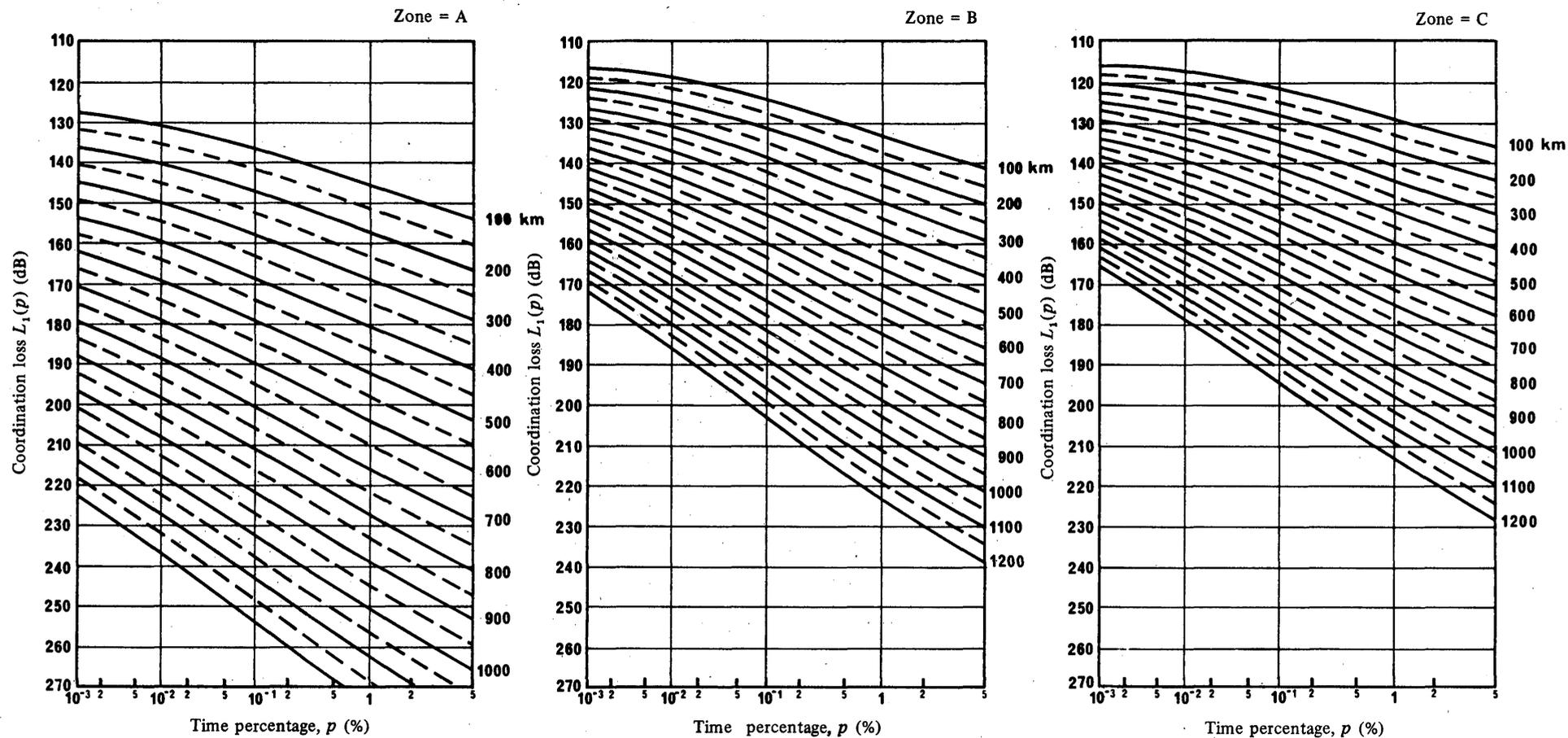
FIGURE 31 – Coordination loss  $L_1(p)$ , dB as a function of time percentage,  $p$ , for isopleths of distance in km
