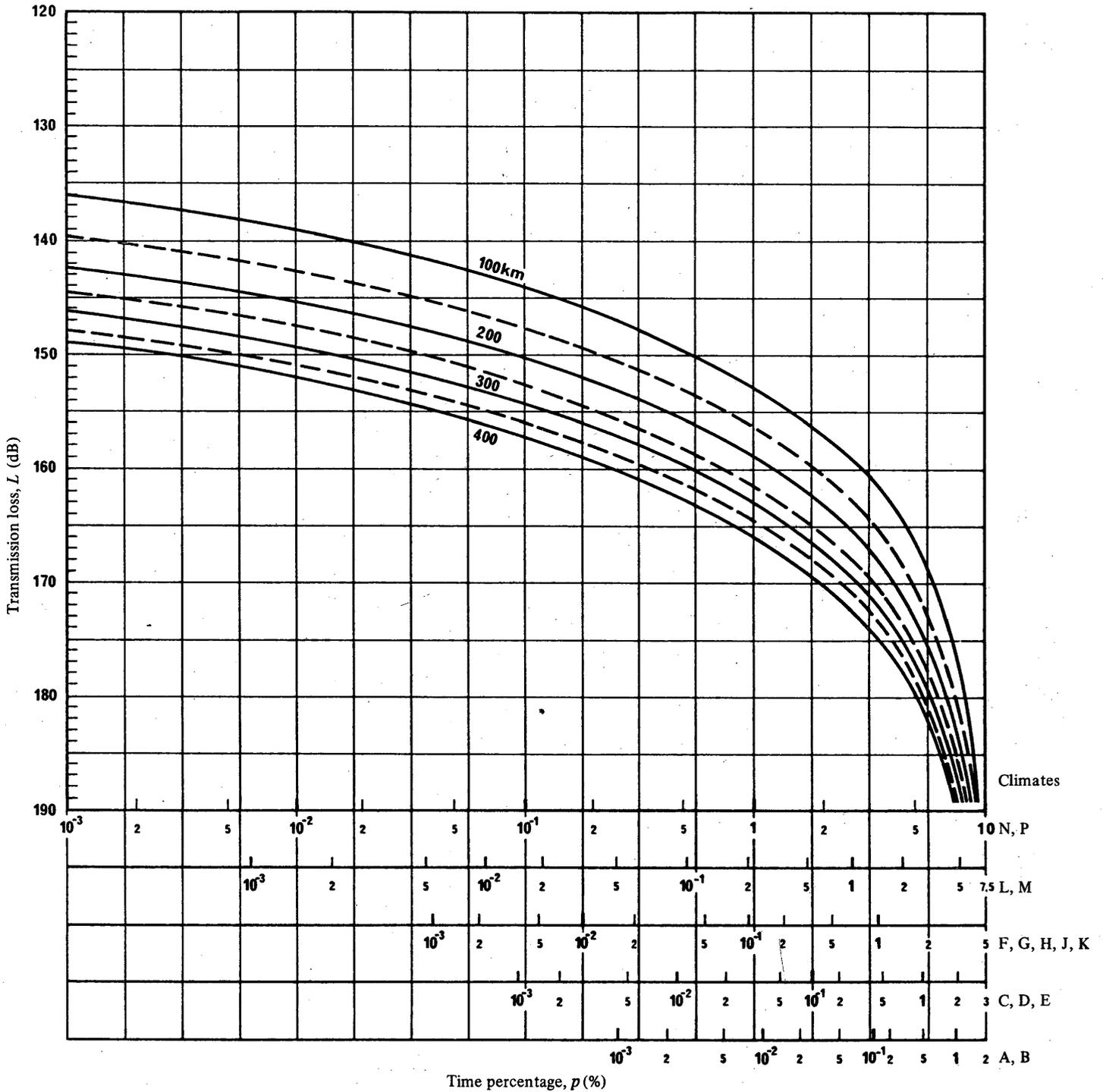
FIGURE 12 — Transmission loss as a function of time percentage,  $p$ , for the different rain climates with hydrometeor scatter distance as a parameter;  $f = 1$  GHz
