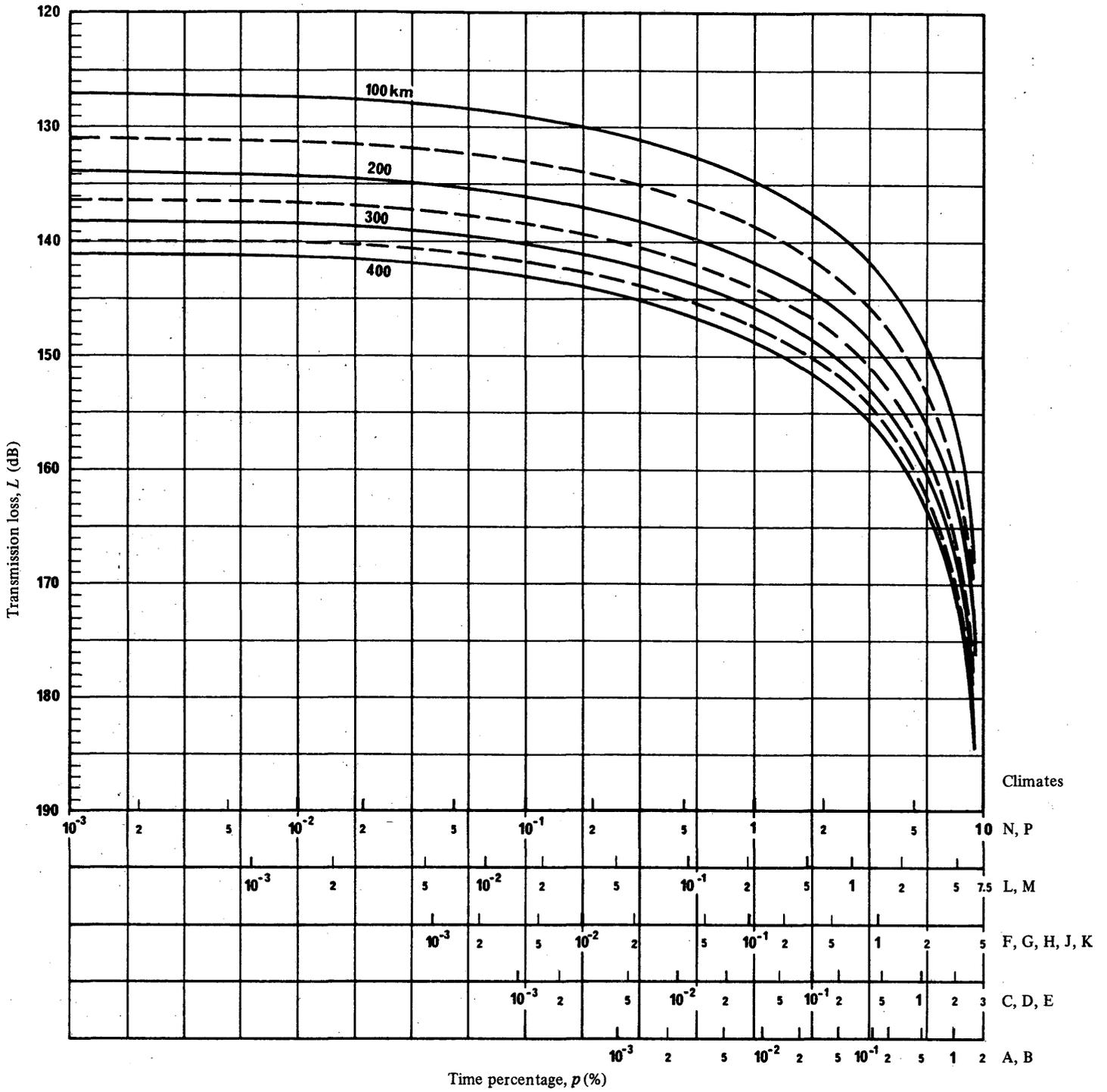
FIGURE 16 – Transmission loss as a function of time percentage,  $p$ , for the different rain climates with hydrometeor scatter distance as a parameter;  $f = 12$  GHz
