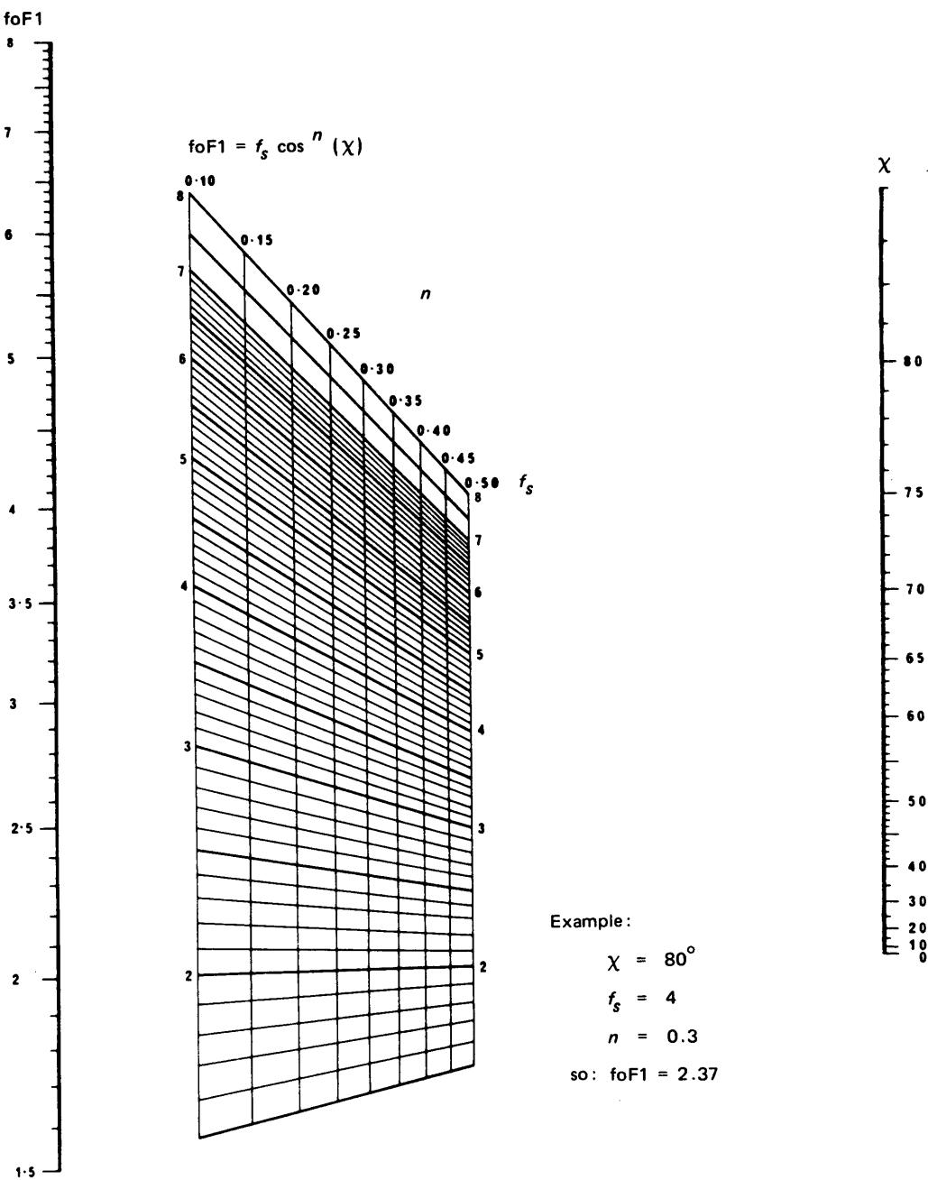
FIGURE 6 – Nomogram for determining the value of  $foF1$
