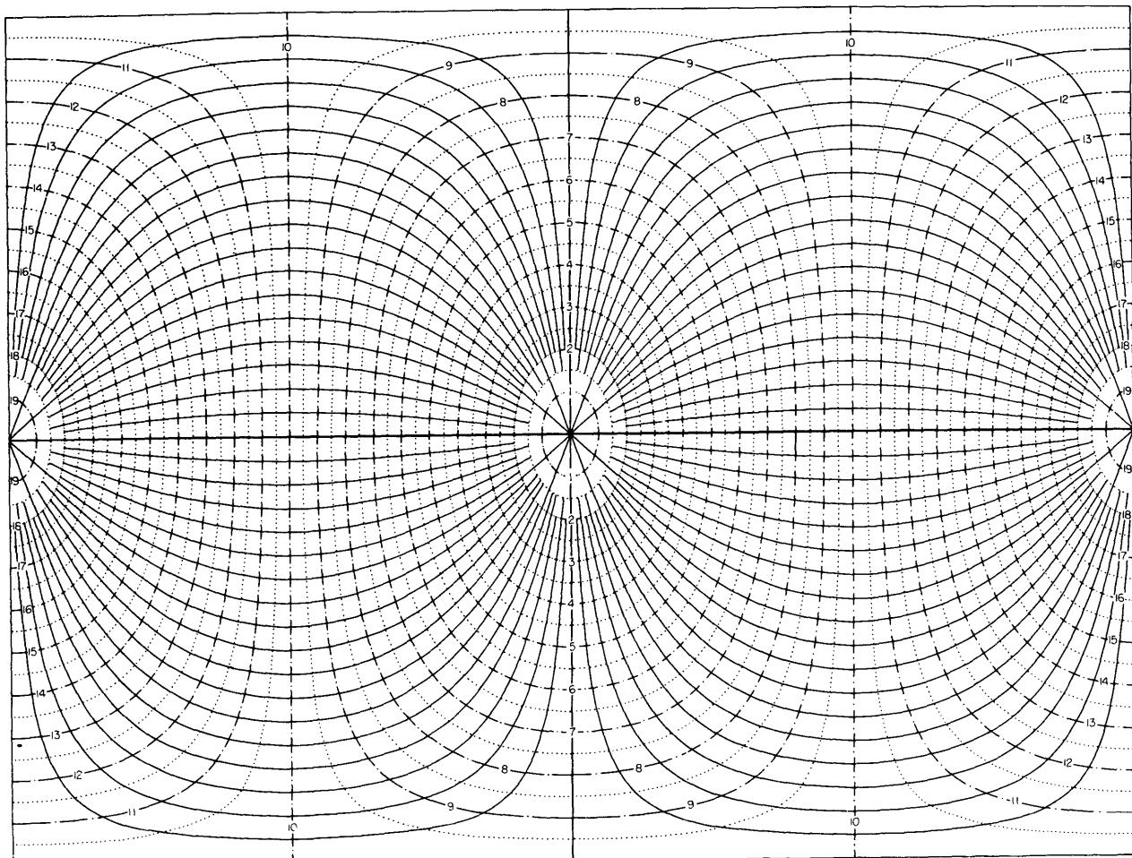
FIGURE 11 — Great-circle chart centred on the equator for use with the world map on a modified cylindrical projection
