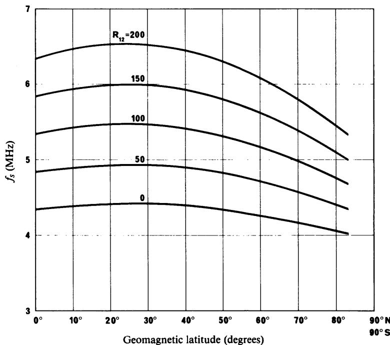
FIGURE 3 – Variation of  $f_s$  with geomagnetic latitude and  $R_{12}$
