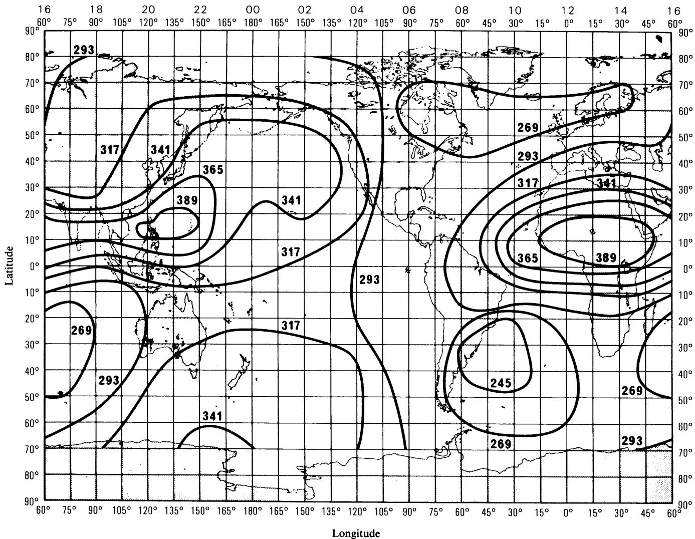
**FIGURE 9 – Predicted hmF2 for 1200 h UTC in June with  $R_{12} = 100$**
