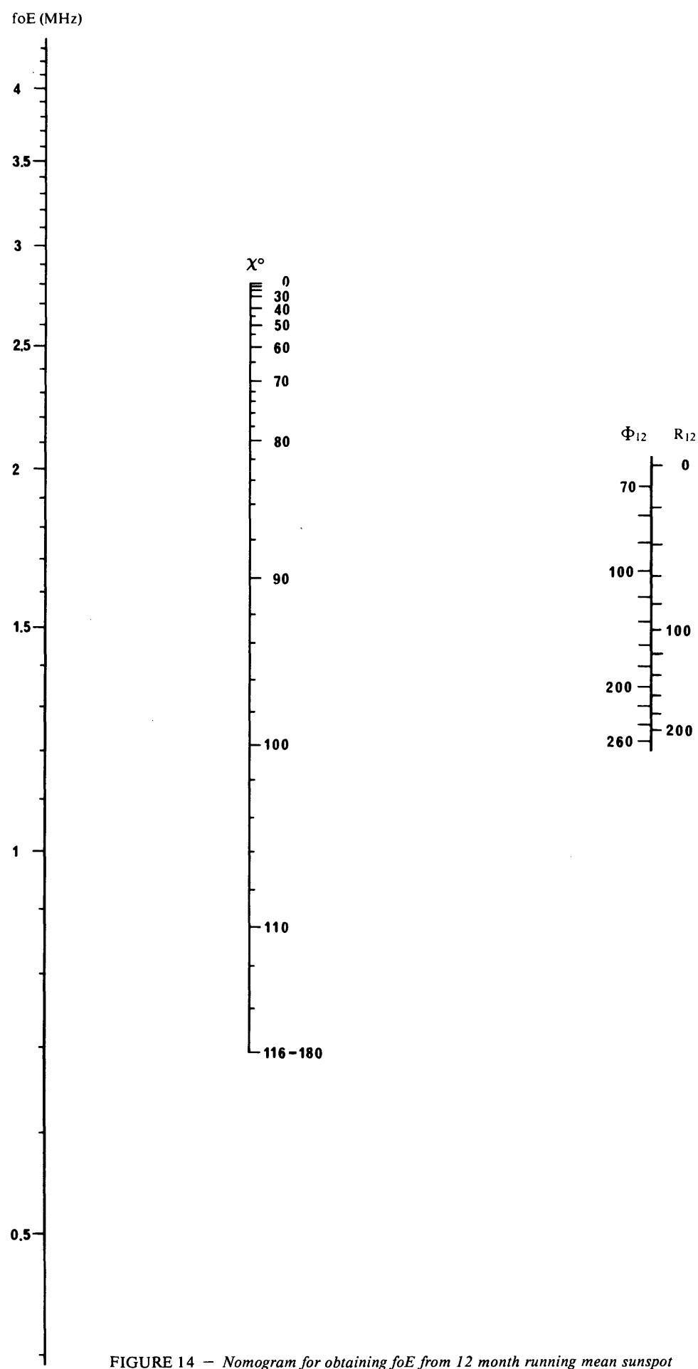
FIGURE 14 — Nomogram for obtaining  $foE$  from 12 month running mean sunspot number,  $R_{12}$ , or solar radio flux,  $\Phi_{12}$ , and the solar-z zenith angle  $\chi$
