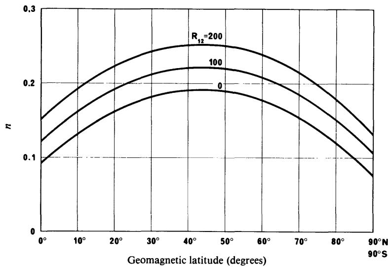
FIGURE 4 – Variation of  $n$  with geomagnetic latitude and  $R_{12}$
