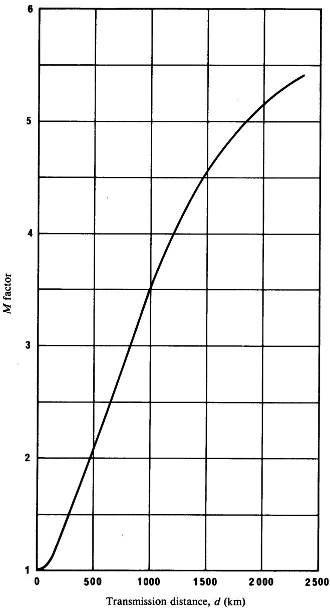
FIGURE 1 – *Distance factor curve for the E layer*
