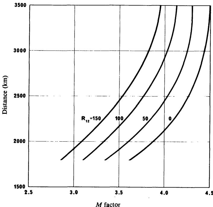
FIGURE 7 - Distance factor curves for the F1 layer
