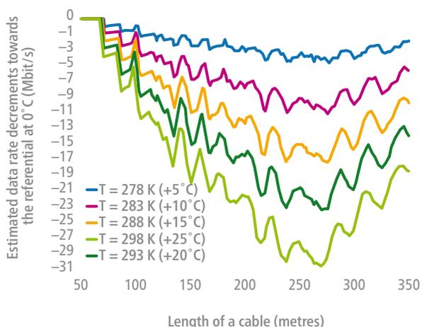
**Figure 3 — Estimated data rates for 212 MHz G.fast for 26 American wire gauge underground cable in a temperature range between 0°C and 25°C**
