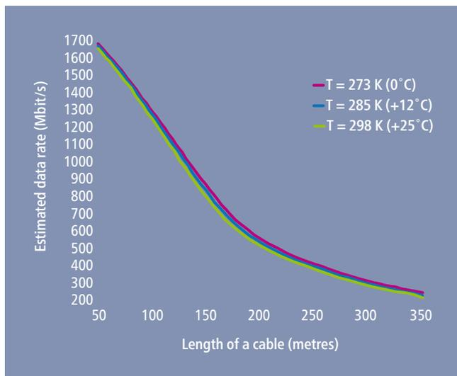
The same simulations were performed for 212 MHz G.fast, with identical temperature conditions and cable parameters. The estimated data rates for 212 MHz G.fast are presented in Figure 3
