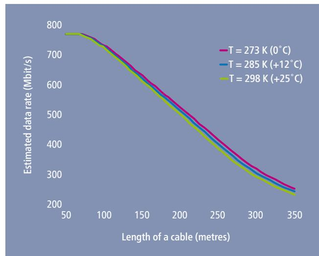
**Figure 2 — Data rate decrements of 106 MHz G.fast towards the reference temperature of 0°C**
