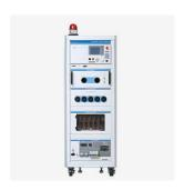
Figure I.1.8-1 – Examples of lightning-surge generators
