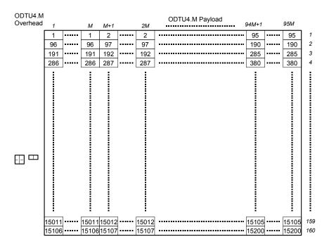
Figure 19-29 – ODTU4.M GMP byte numbering
