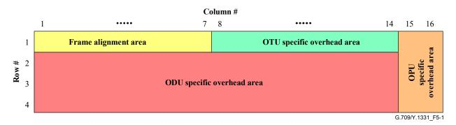
Figure 5-1 – OTUk, ODUk and OPUk overhead
