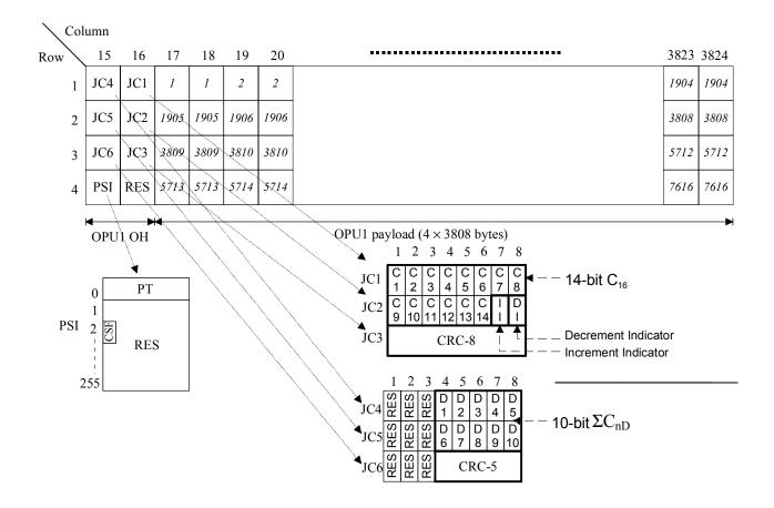
Figure 17-13 – OPU1 frame structure for the mapping of a supra-1.238 to sub-2.488 Gbit/s client signal
