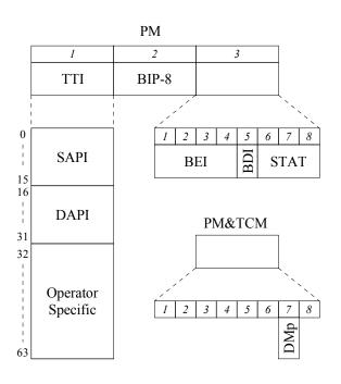
Figure 15-13 – ODUk path monitoring overhead
