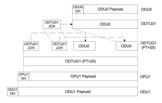
Figure 7-4 – ODU0 into ODU1 multiplexing method via ODTUG1 (PT=20)
