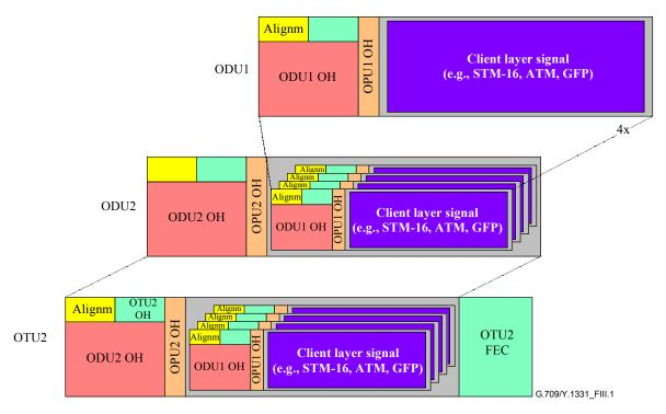
NOTE – The ODU1 floats in ¼ of the OPU2 payload area. An ODU1 frame will cross multiple ODU2 frame boundaries. A complete ODU1 frame (15296 bytes) requires the bandwidth of (15296/3808 = ) 4.017 ODU2 frames. This is not illustrated.
