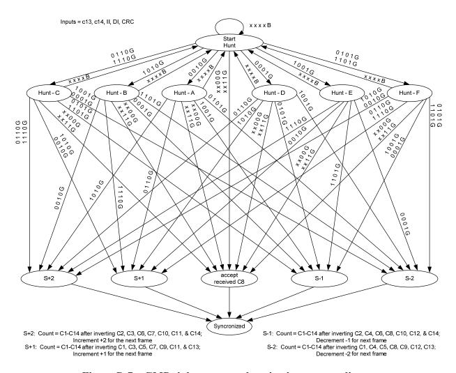
Figure D.7 – GMP sink count synchronization process diagram
