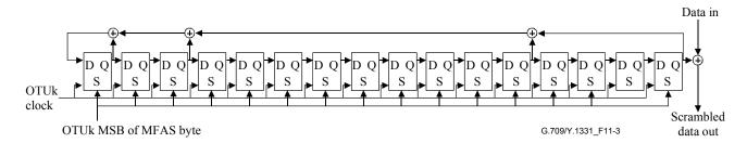
Figure 11-3 – Frame synchronous scrambler
