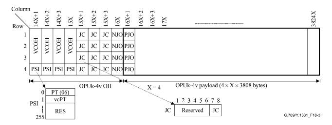
Figure 18-3 – OPUk-4v frame structure for the mapping of a CBR10G or CBR40G signal
