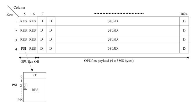
Figure 17-19 - OPUflex frame structure for the mapping of a supra-2.488 Gbit/s client signal
