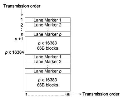
Figure VII.1 – Deskewed/serialized stream of 66B blocks
