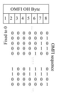
Figure 19-21 – OPU4 multiframe identifier (OMFI) overhead
