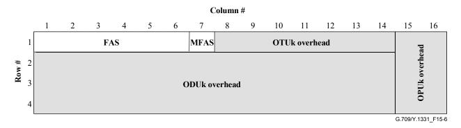
Figure 15-6 – OTUk/ODUk frame alignment overhead
