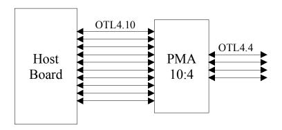
Figure X.1 – Illustration of application of OTL4.10 interface
