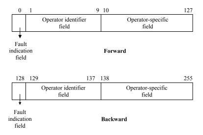
Figure 15-21 – Forward/backward field structure
