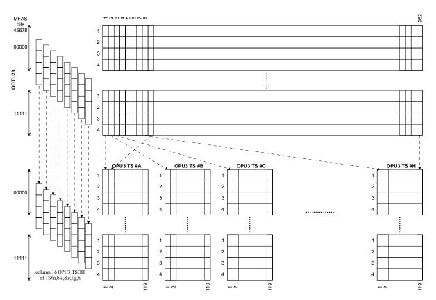
Figure 19-9 – Mapping of ODTU23 into 4 OPU3 2.5G tributary slots (#A, #B, #C, #D with A<B<C<D) (top) and 8 OPU3 1.25G tributary slots (#A, #B, #C, #D, #E, #F, #G, #H with A<B<C<D<E<F<G<H) (bottom)
