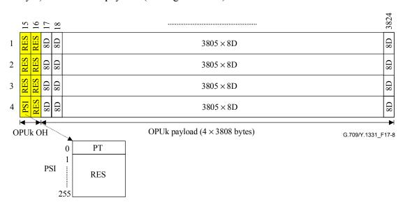
Figure 17-10 – OPUk frame structure and mapping of 2 147 483 647-bit pseudo-random test sequence into OPUk
