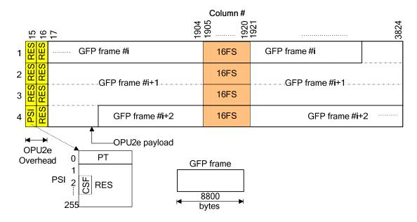
Figure 17-17 – Mapping of transcoded FC-1200 into OPU2e
