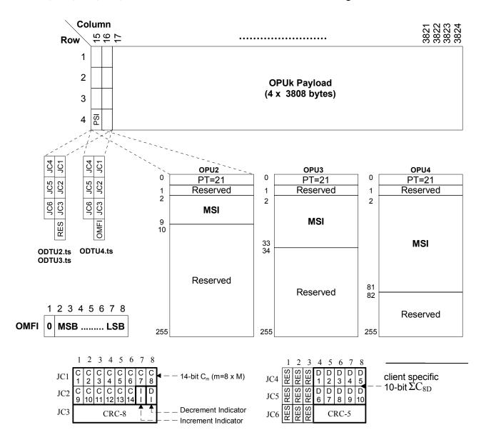
Figure 19-14C – OPUk (k=2,3,4) multiplex overhead associated with an ODTUk.ts (payload type = 21)
