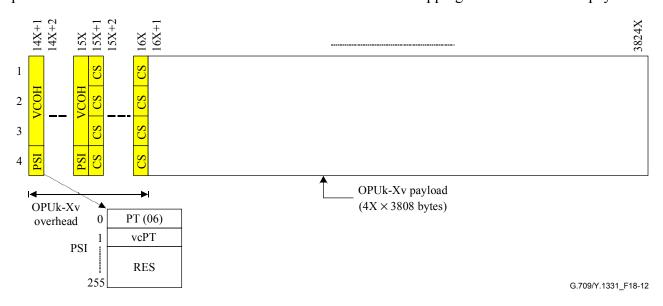
Figure 18-12 – OPUk-Xv frame structure for the mapping of a synchronous constant bit stream
