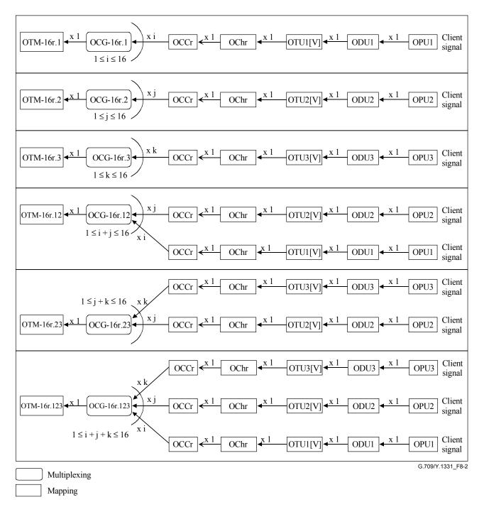
Figure 8-2 – OTM-16r.m multiplexing structure examples
