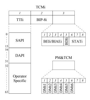
Figure 15-14 – ODUk tandem connection monitoring #i overhead
