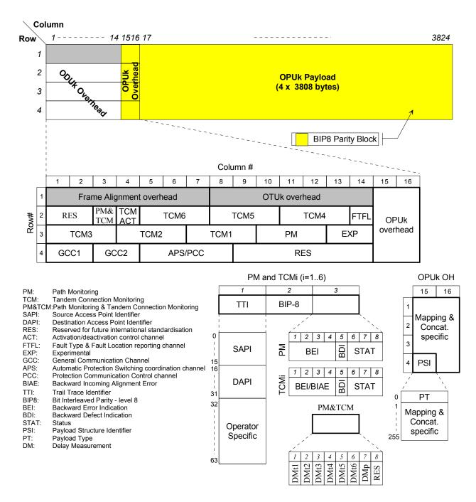
Figure 15-3 – ODUk frame structure, ODUk and OPUk overhead
