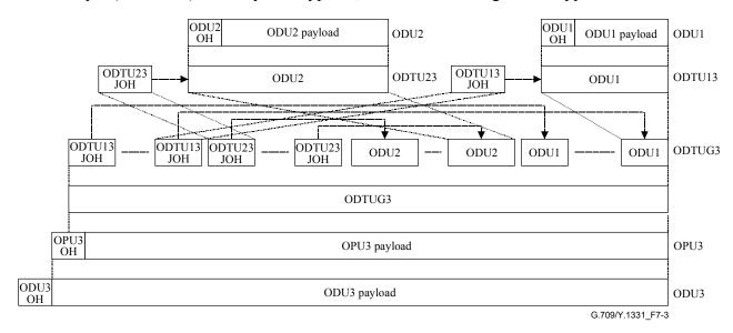
Figure 7-3 – ODU1 and ODU2 into ODU3 multiplexing method via ODTUG3 (PT=20)
