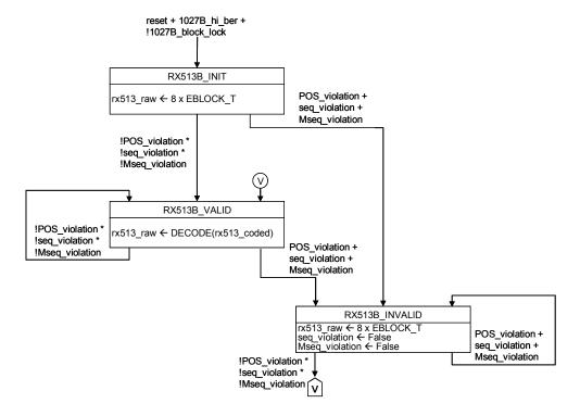
Figure VIII.2 – Receive state machine for the 512B/513B code blocks including lane alignment markers
