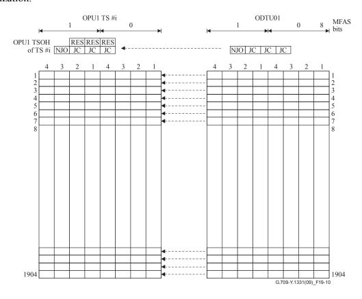
Figure 19-10 – Mapping of ODTU01 (excluding JOH) into OPU1 1.25G tributary slot
