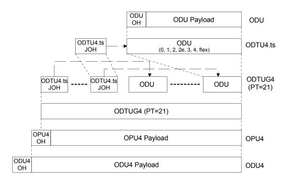
Figure 7-7 – ODU0, ODU1, ODU2, ODU2e, ODU3 and ODUflex into ODU4 multiplexing method via ODTUG4 (PT=21)
