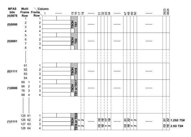
Figure 19-2 - OPU3 tributary slot allocation
