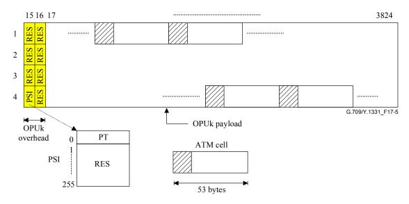
Figure 17-6 – OPUk frame structure and mapping of ATM cells into OPUk
