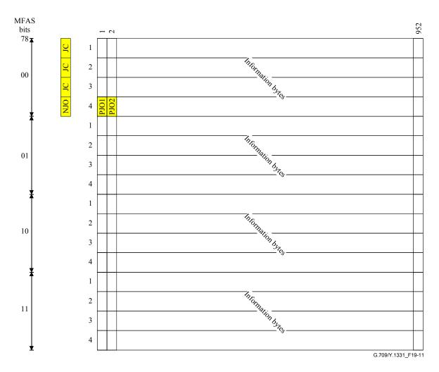
Figure 19-23A – ODTU12 frame format and mapping of ODU1 (case of mapping in 2.5G TS1)
