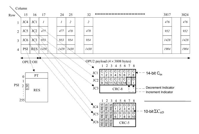
Figure 17-14 – OPU2 frame structure for the mapping of a CBR client signal
