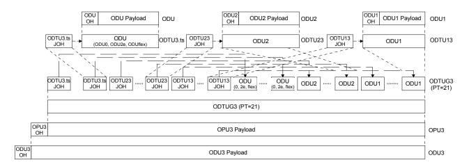
Figure 7-6 – ODU0, ODU1, ODU2, ODU2e and ODUflex into ODU3 multiplexing method via ODTUG3 (PT=21)
