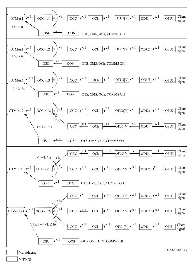
Figure 8-4 – OTM-n.m multiplexing structure examples
