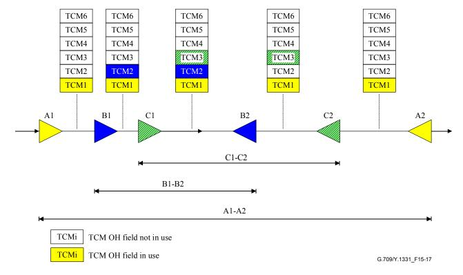
Figure 15-17 – Example of overlapping ODUk monitored connections
