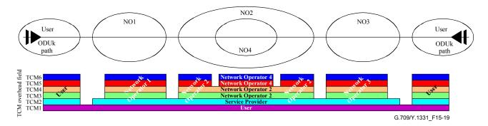
Figure 15-19 – Example of TCM overhead field assignment
