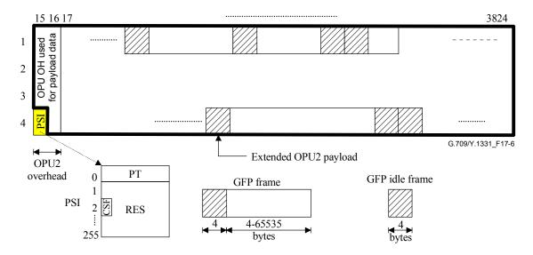
Figure 17-8 – OPU2 frame structure and mapping of GFP frames into Extended OPU2 payload area
