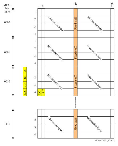
Figure 19-24A – ODTU13 frame format and mapping of ODU1 (case of mapping in 2.5G TS3)
