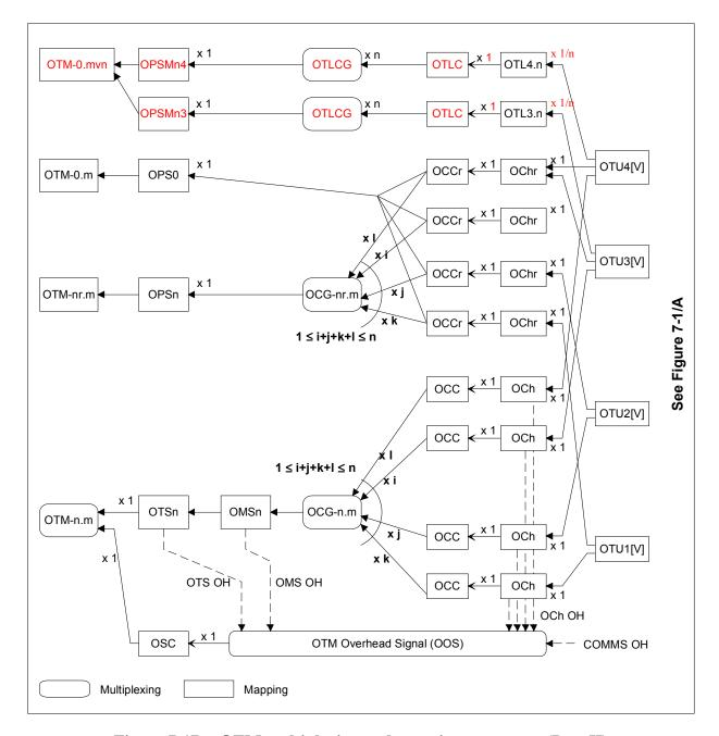
Figure 7-1B – OTM multiplexing and mapping structures (Part II)
