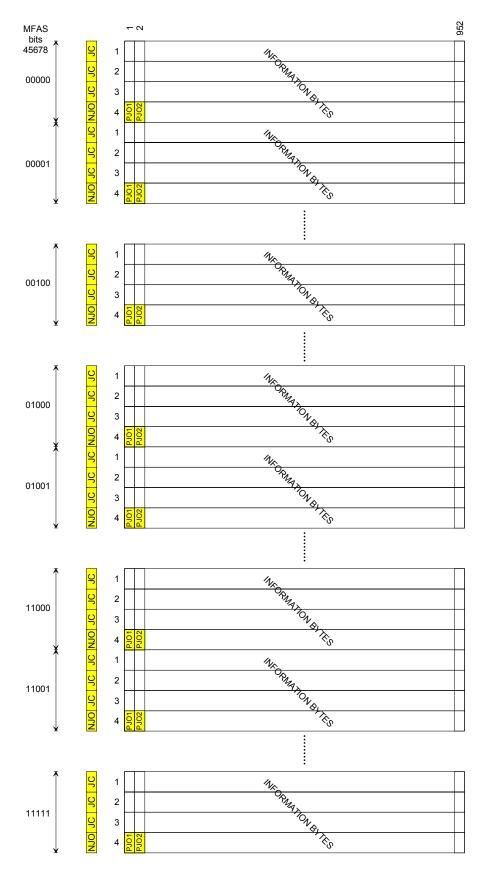
Figure 19-25B – ODTU23 frame format and mapping of ODU2 (case of mapping in 1.25G TS 1,2,5,9,10,25,26,32)
