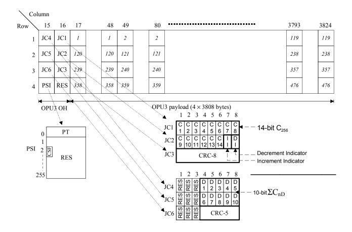
Figure 17-15 – OPU3 frame structure for the mapping of a CBR client signal
