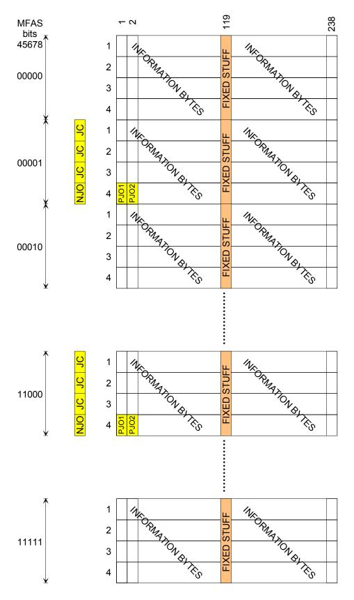
Figure 19-24B – ODTU13 frame format and mapping of ODU1 (case of mapping in 1.25G TS2 and TS25)
