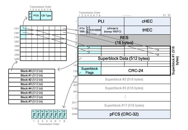
Figure 17-18 – GFP frame format for FC-1200
