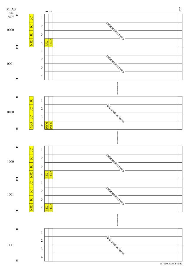
Figure 19-25A – ODTU23 frame format and mapping of ODU2 (case of mapping in 2.5G TS 1,5,9,10)
