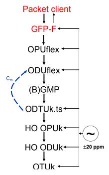
Figure 12-3 – ODUflex clock generation for GFP-F mapped packet client signals
