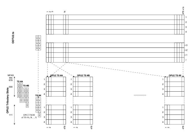
Figure 19-11 - Mapping of ODTU2.ts into 'ts' OPU2 1.25G tributary slots
