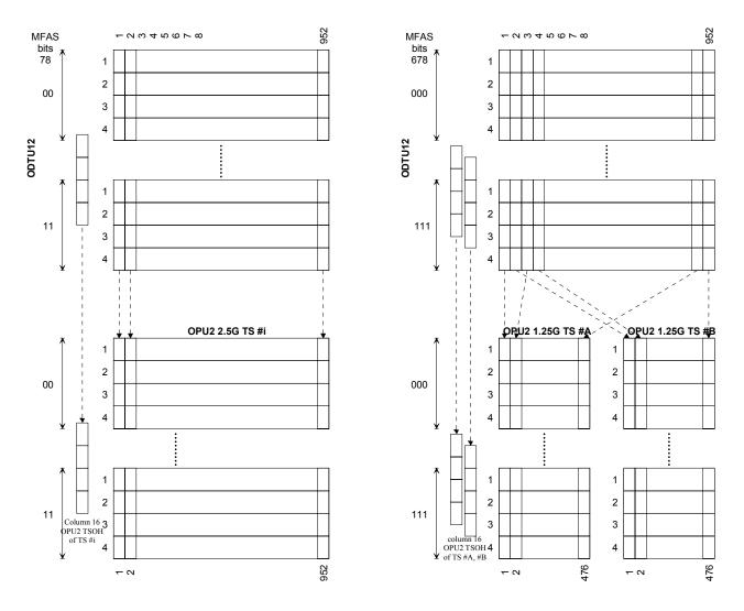
Figure 19-7 – Mapping of ODTU12 into one OPU2 2.5G tributary slot (left) and two OPU2 1.25G tributary slots (right)
