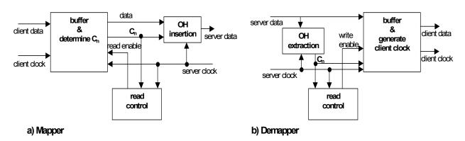
Figure D.1 – Generic functionality of a mapper/demapper circuit
