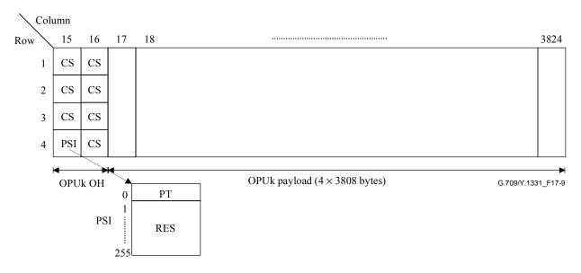
Figure 17-11 – OPUk frame structure for the mapping of a synchronous constant bit stream
