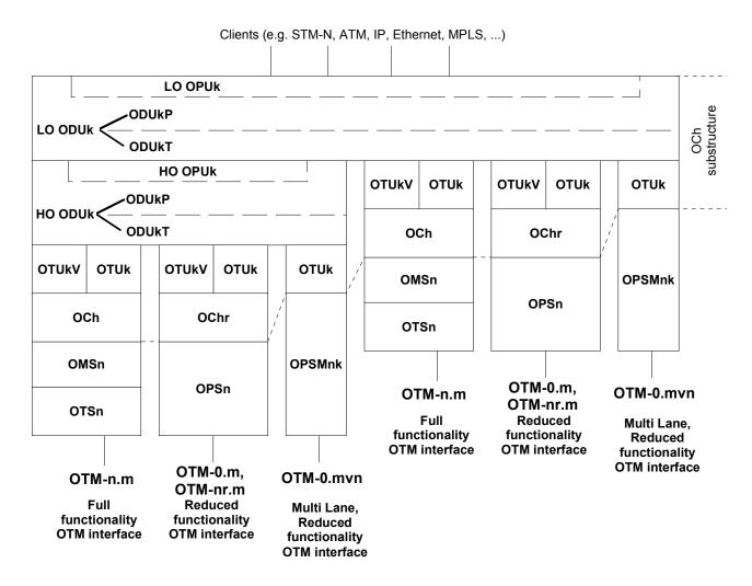
Figure 6-1 – Structure of the OTN interfaces
