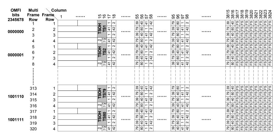
Figure 19-4A – OPU4 1.25G tributary slot allocation
