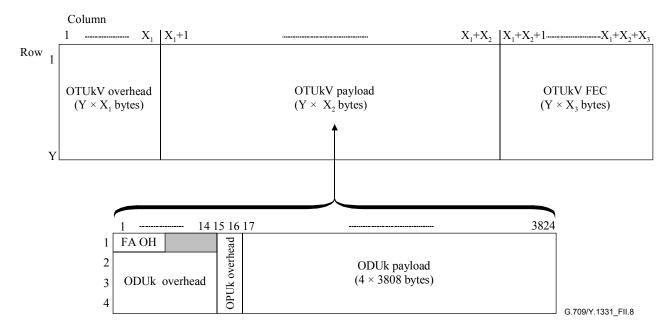
Figure II.8 – Asynchronous (or bit synchronous) mapping of ODUk into OTUkV
