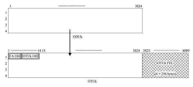
Figure 11-1 – OTUk frame structure
