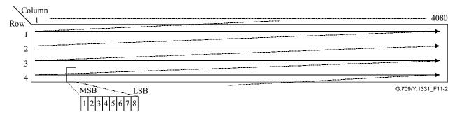
Figure 11-2 – Transmission order of the OTUk frame bits
