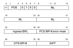
Figure VII.2 – Transcoded lane marker format
