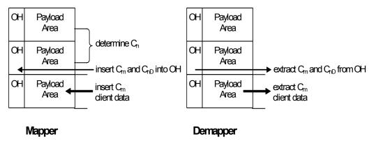
Figure D.5 – Processing flow for GMP in OTN
