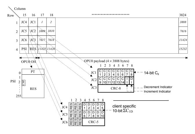
Figure 17-12 – OPU0 frame structure for the mapping of a sub-1.238 Gbit/s client signal
