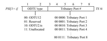
Figure 19-19B – OPU2 MSI coding – Payload type 21
