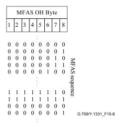
Figure 15-8 – Multiframe alignment signal overhead
