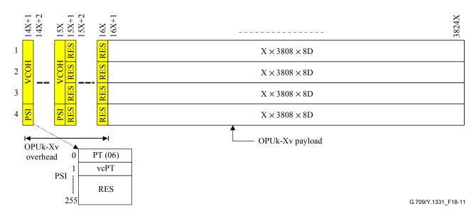
Figure 18-11 – OPUk-Xv frame structure and mapping of 2 147 483 647-bit pseudo-random test sequence into OPUk-Xv
