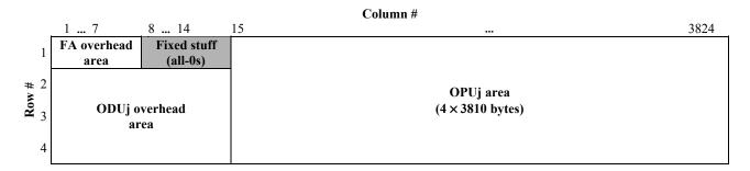
Figure 19-22 – Extended ODUj frame structure (FA OH included, OTUj OH area contains fixed Stuff)
