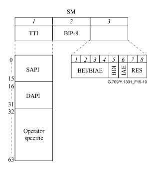
Figure 15-10 – OTUk section monitoring overhead
