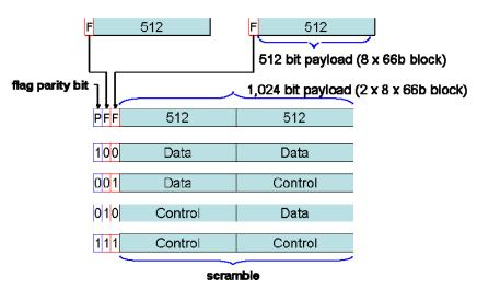
Figure VIII.1 – Flag parity bit on two 513B blocks (1027B code)
