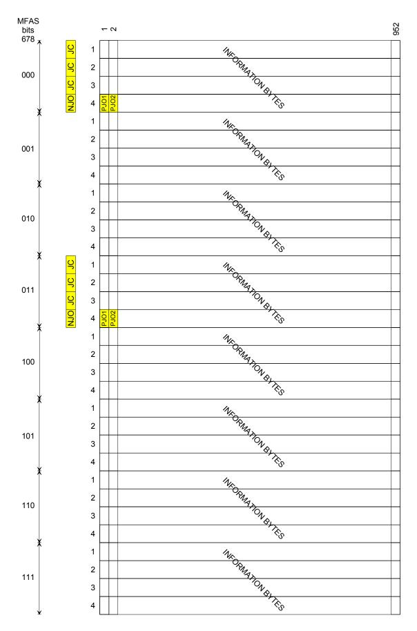
Figure 19-23B – ODTU12 frame format and mapping of ODU1 (case of mapping in 1.25G TS1 and TS4)
