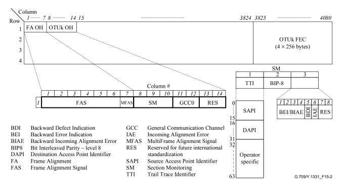
Figure 15-2 – OTUk frame structure, frame alignment and OTUk overhead
