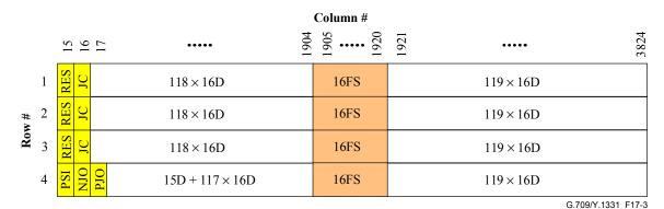
Figure 17-5 – Mapping of a CBR10G3 signal into OPU2e
