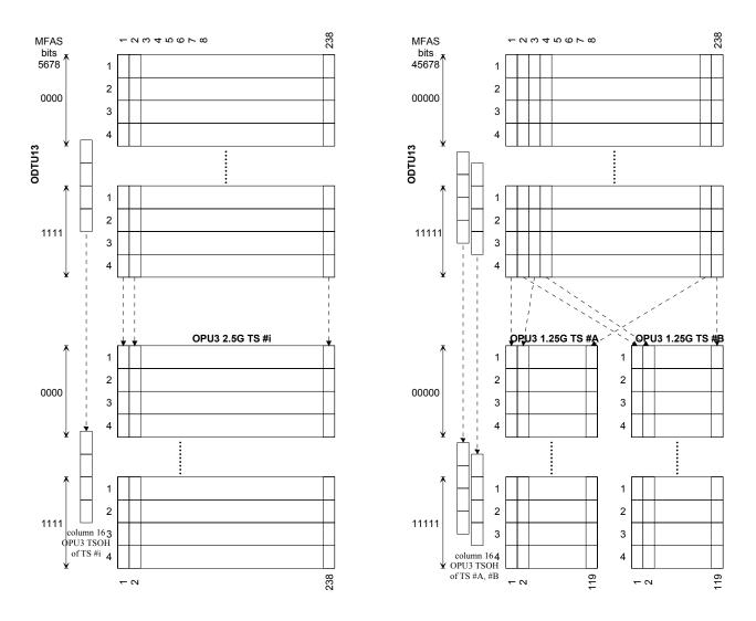
Figure 19-8 – Mapping of ODTU13 into one OPU3 2.5G tributary slot (left) and two OPU3 1.25G tributary slots (right)
