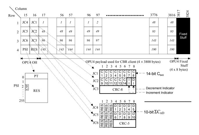
Figure 17-16 – OPU4 frame structure for the mapping of a CBR client signal
