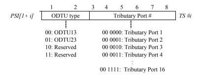
Figure 19-16B - OPU3 MSI coding - Payload type 20
