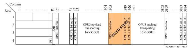
Figure IV.1 – Fixed stuff locations when mapping 16 × ODU1 into OPU3
