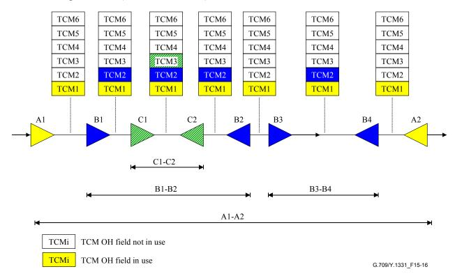
Figure 15-16 – Example of nested and cascaded ODUk monitored connections
