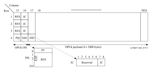
Figure 17-1 – OPUk frame structure for the mapping of a CBR2G5, CBR10G or CBR40G signal
