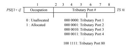
Figure 19-18B - OPU4 MSI coding - Payload type 21
