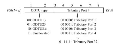
Figure 19-20B - OPU3 MSI coding - Payload type 21
