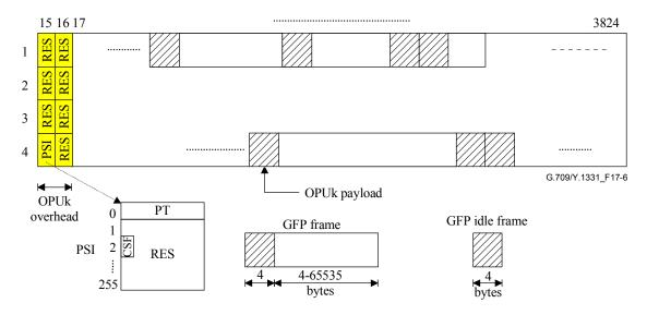
Figure 17-7 – OPUk frame structure and mapping of GFP frames into OPUk
