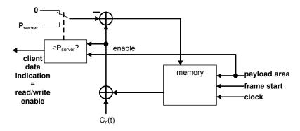
Figure D.4 – Sigma-Delta accumulator
