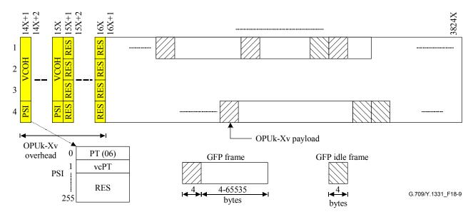
Figure 18-9 – OPUk-Xv frame structure and mapping of GFP frames into OPUk-Xv
