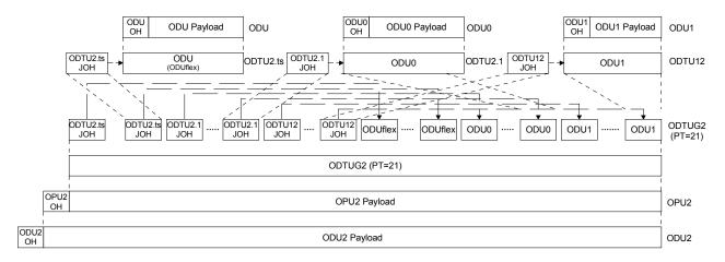
Figure 7-5 – ODU0, ODU1 and ODUflex into ODU2 multiplexing method via ODTUG2 (PT=21)
