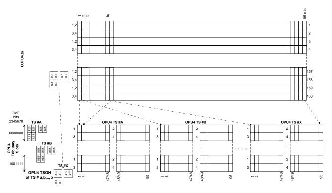
Figure 19-13 – Mapping of ODTU4.ts into 'ts' OPU4 1.25G tributary slots
