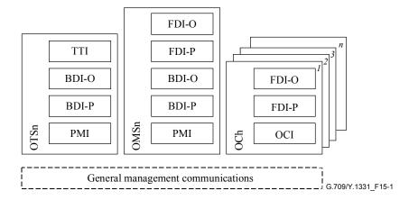
Figure 15-1 – OTSn, OMSn and OCh overhead as logical elements within the OOS
