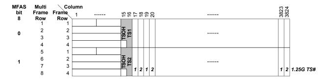
Figure 19-3 – OPU1 tributary slot allocation
