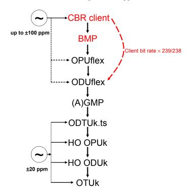
Figure 12-2 – ODUflex clock generation for CBR signals
