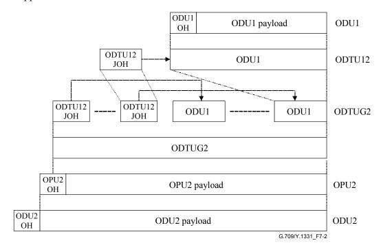
Figure 7-2 – ODU1 into ODU2 multiplexing method via ODTUG2 (PT=20)
