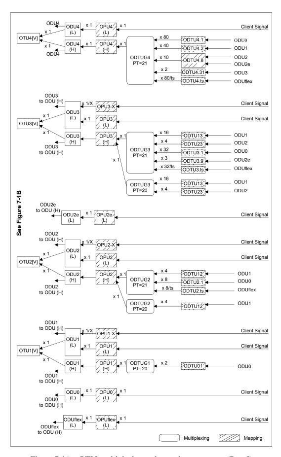
Figure 7-1A – OTM multiplexing and mapping structures (Part I)
