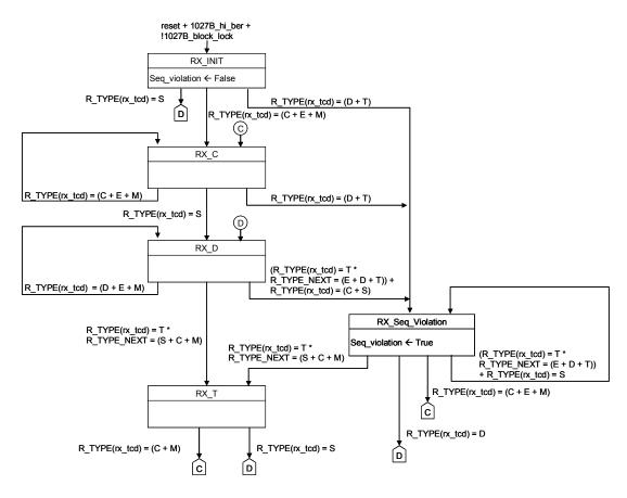
Figure VIII.3 – Trans-decode state machine for the 64B/66B code blocks including the lane alignment markers
