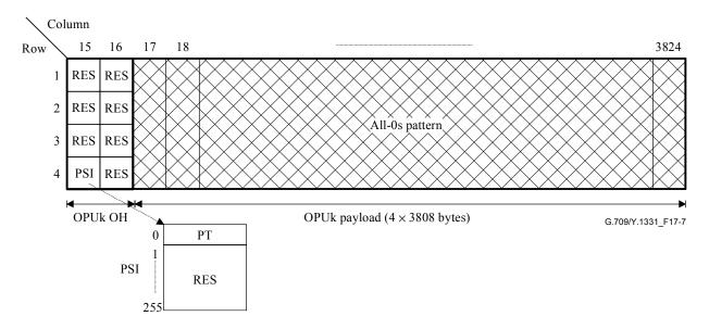
Figure 17-9 – OPUk frame structure and mapping of NULL client into OPUk
