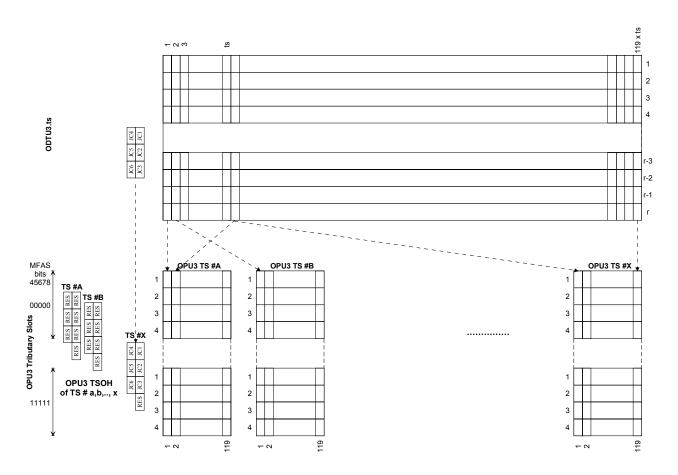
Figure 19-12 - Mapping of ODTU3.ts into 'ts' OPU3 1.25G tributary slots
