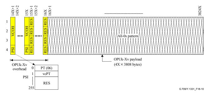
Figure 18-10 – OPUk-Xv frame structure and mapping of NULL client into OPUk-Xv
