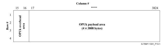
Figure 13-1 – OPUk frame structure
