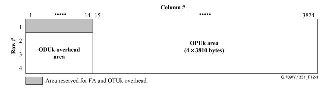
Figure 12-1 – ODUk frame structure
