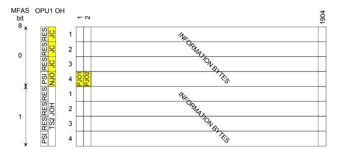
Figure 19-26 – Mapping of ODU0 in OPU1 TS1
