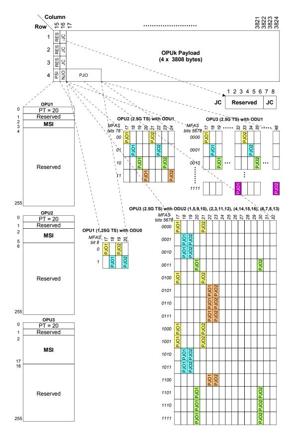
Figure 19-14A – OPUk (k=1,2,3) multiplex overhead associated with an ODTUjk only (payload type = 20)
