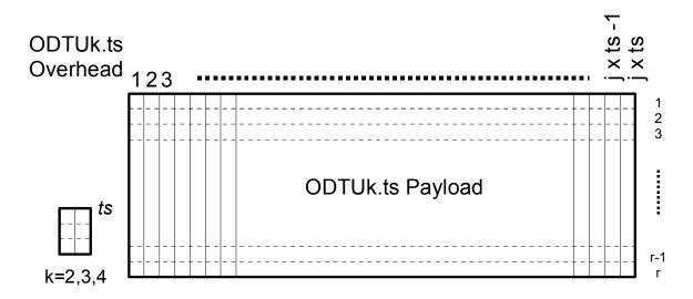
Figure 19-6 – ODTUk.ts frame formats
