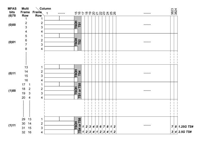
Figure 19-1 – OPU2 tributary slot allocation
