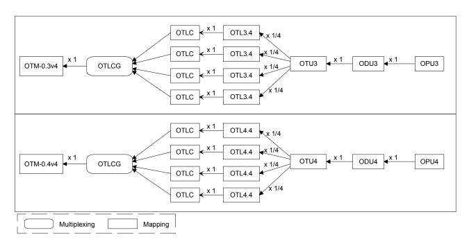
Figure 8-3 - OTM-0.3v4 and OTM-0.4v4 structure
