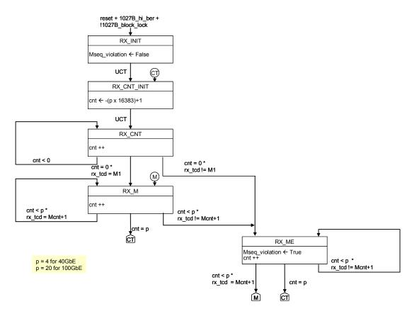
Figure VIII.4 – Receive state machine for the lane alignment markers
