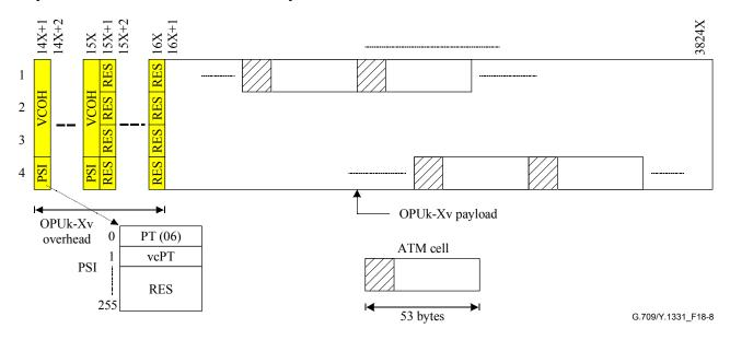
Figure 18-8 – OPUk-Xv frame structure and mapping of ATM cells into OPUk-Xv
