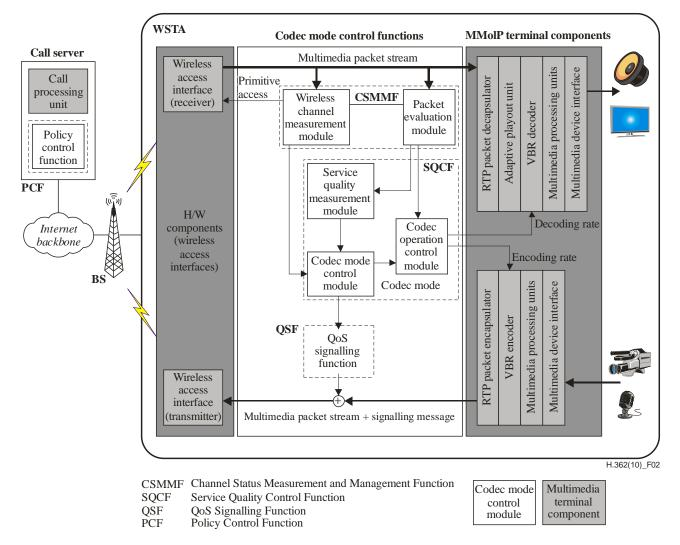
Figure 2 – Terminal architecture for codec mode control
