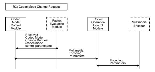
Figure 9 – Signalling flow to apply the received codec mode change request
