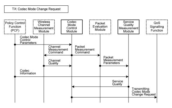
Figure 8 – Signalling flow to change the codec mode of the remote WSTA
