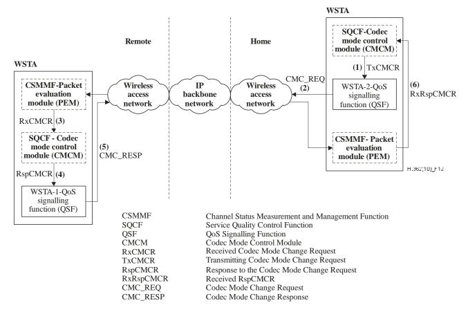
Figure 12 – QoS signalling function (QSF)
