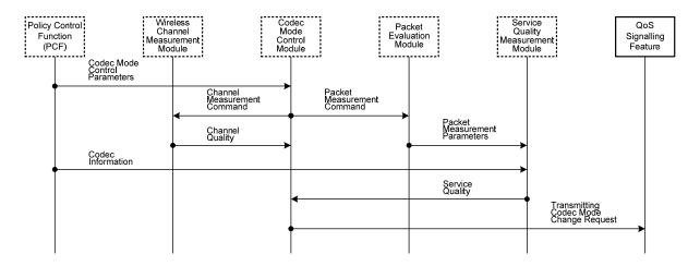
Figure 14 – Detailed message exchange sequences for the transmitted codec mode decision procedure
