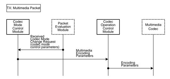
**Figure 11 – Signalling flow to apply the multimedia encoding parameters**
