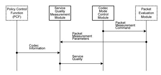
Figure 7 – Signalling flow to measure the service quality
