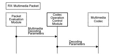
Figure 10 – Signalling flow to apply the multimedia decoding parameters
