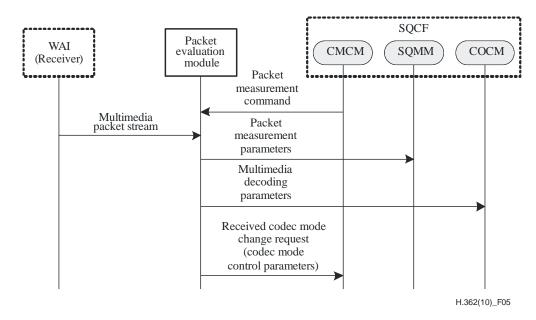
Figure 5 – Signalling flow for the packet evaluation module (PEM)
