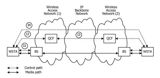
Figure 1 – Conceptual reference network architecture for adaptive QoS control using variable bit-rate codecs
