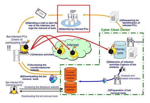
Figure 2 – Workflow of bots detection and response in CCC
