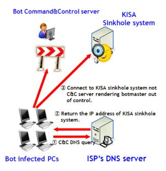
Figure 3 – DNS sinkhole operation
