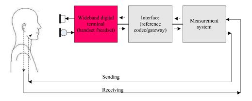
**Figure 1 – Test configuration**
