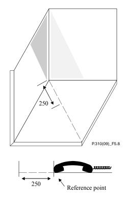
Figure 4 – Reference corner and reference position
