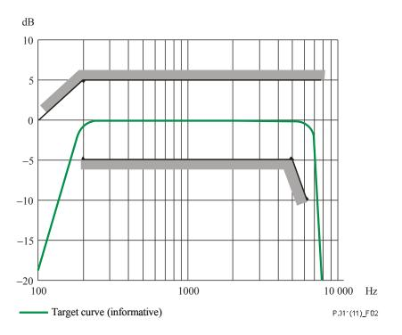
Figure 2 – Handset sending sensitivity/frequency mask
