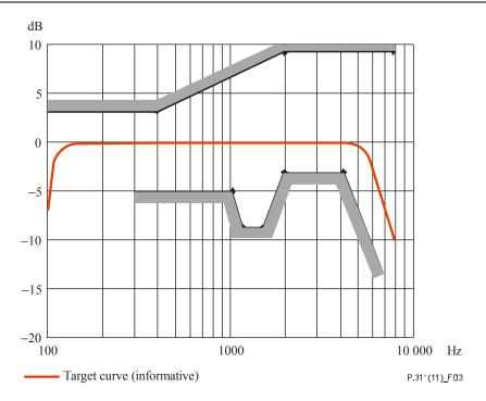
Figure 3 – Handset receiving sensitivity/frequency mask
