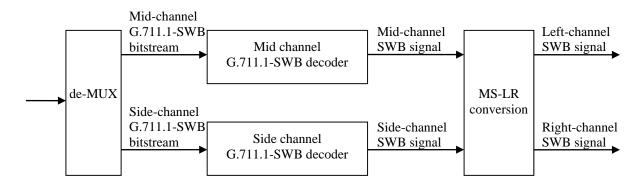
Figure IV.3 – Decoder block diagram of MS stereo using ITU-T G.711.1-SWB
