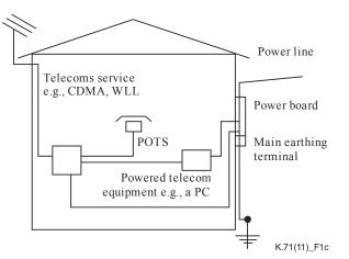
Figure 1c – Basic antenna-provided service
