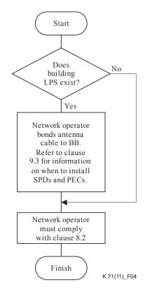
Figure 4 – Process for an antenna on a separate tower
