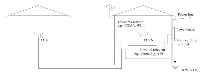
Figure 1d - Basic antenna-provided service with service extended to an out-building
