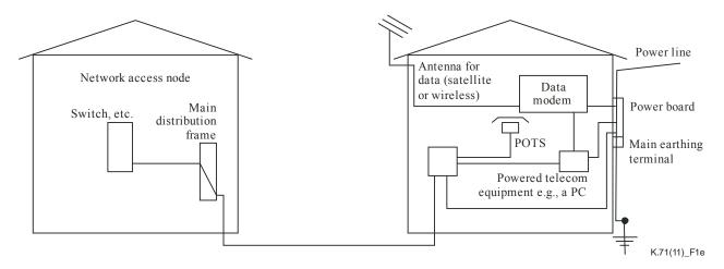
Figure 1e – Telecommunications service plus an antenna for Internet service
