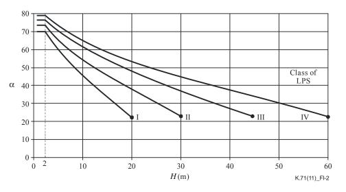
Figure I.1 – Volume protected by a vertical air-termination rod
