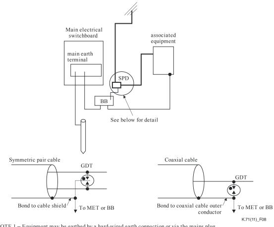
NOTE 1 – Equipment may be earthed by a hard-wired earth connection or via the mains plug. NOTE 2 – To be effective, the length of the bond wire from the cable screen and SPD to the MET must be < 1.5 m. NOTE 3 – If required, the cable shield or coaxial cable outer may be bonded to the MET or BB via a GDT. NOTE 4 – Refer to [ITU-T K.66] for further bonding information.
