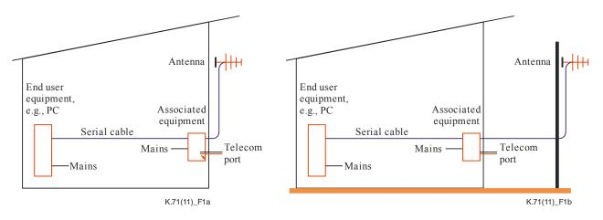
Figure 1a – Antenna attached to structure
