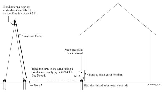
NOTE 1 - To be effective, the bond wire length from the SPD to the MET must be less than 1.5 m long.
