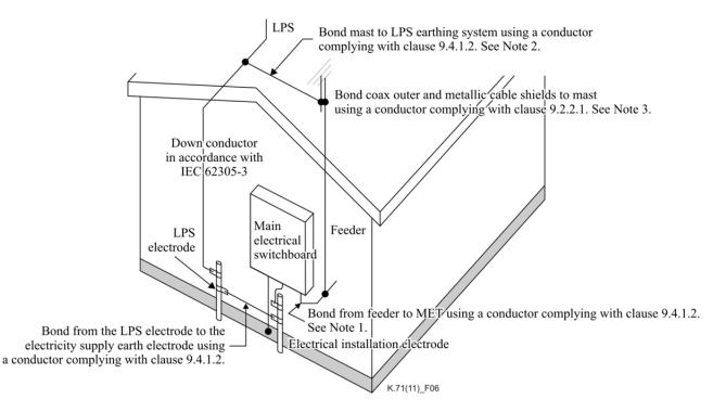
NOTE 1 – The bond to MET may be via a BB or a connection to the electrical installation electrode. NOTE 2 – If antenna is adequately isolated from the LPS, bonding is not required. See [IEC 62305-3] for the required clearances. NOTE 3 – In a normal installation a bond will already exist between the coax outer/metallic cable shield and the mast.
