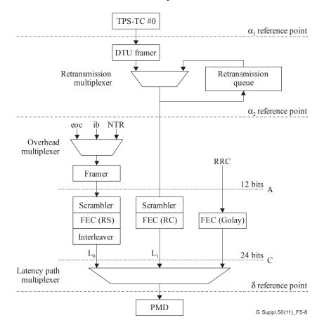
Figure 5-8 – Reference model when retransmission is enabled in both directions
