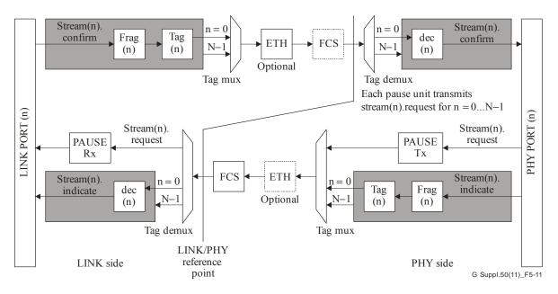
Figure 5-11 – Reference model for the LINK/PHY interface
