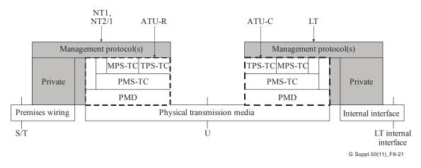
Figure 6-21 – Management plane protocol reference architecture for ITU-T G.99x Recommendations
