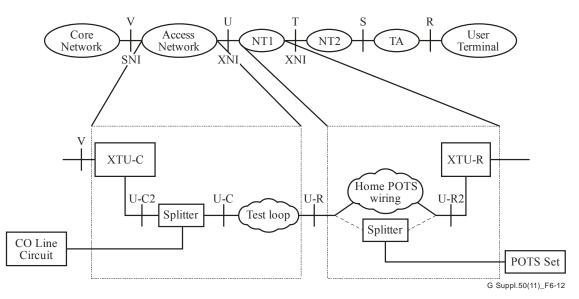
Figure 6-12 – ITU-T G.996.1 system reference model and its alignment with the generic reference configuration
