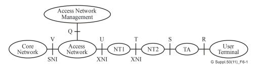
Figure 6-1 – A reference configuration for a generic ITU-T G.99x system
