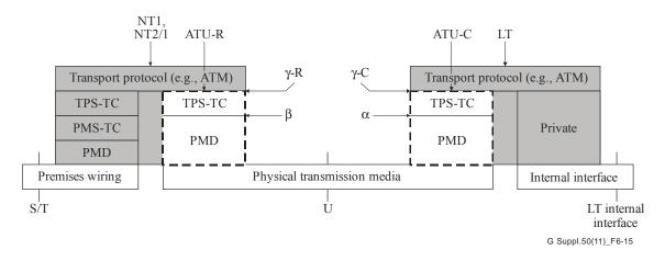
Figure 6-15 – User plane protocol reference architecture for ITU-T G.992.1 and ITU-T G.992.2
