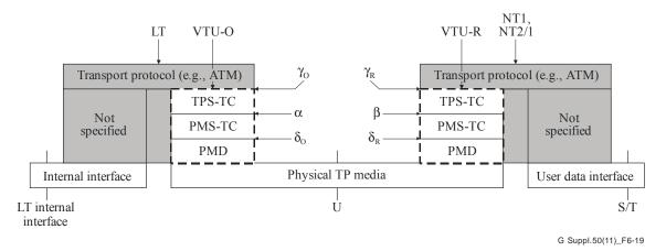
Figure 6-19 – User plane protocol reference model for ITU-T G.993.1 and ITU-T G.993.2
