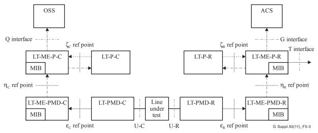
NOTE: arrows show flow of data elements only; flow of control elements are bi-directional (not shown).
