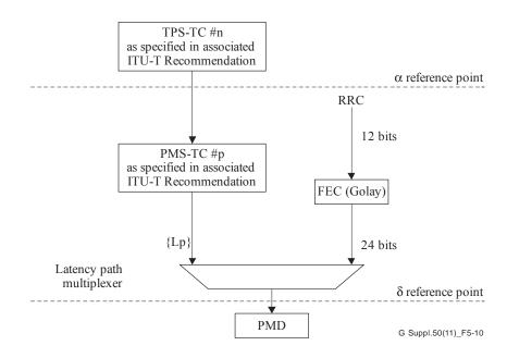
Figure 5-10 – Reference model in the return direction when retransmission is enabled in a single direction
