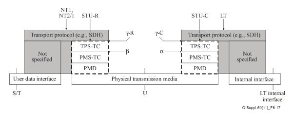
Figure 6-17 – User plane protocol reference architecture for ITU-T G.991.2
