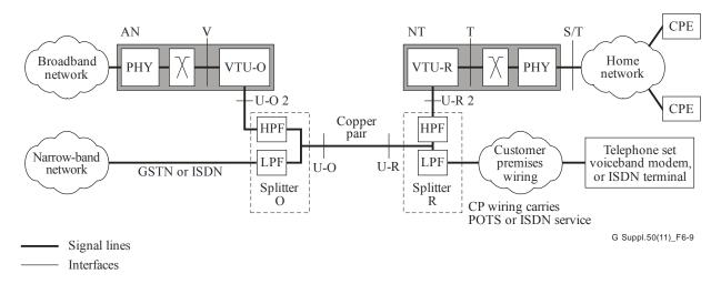
Figure 6-9 – Generic application reference model for remote deployment with splitter
