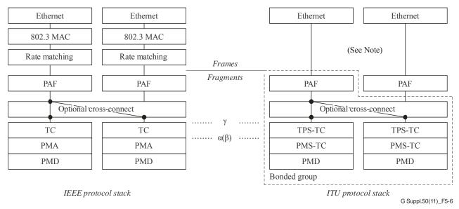
NOTE – A rate matching algorithm may be implemented somewhere above the PAFT. The IEEE rate matching algorithm is specifically designed for the Ethernet MAC.
