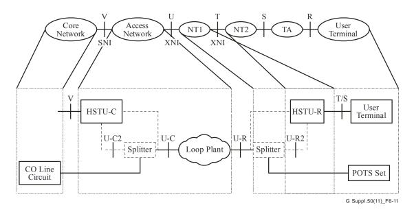
Figure 6-11 – ITU-T G.994.1 system reference model and its alignment with the generic reference configuration
