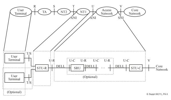
Figure 6-3 – ITU-T G.991.2 system reference model and its alignment with the generic reference configuration
