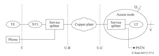
Figure 7-3 – ITU-T G.992.1 data service presentation at the T interface
