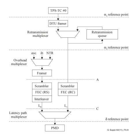
Figure 5-9 – Reference model in the forward direction when retransmission is enabled in a single direction
