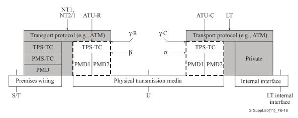
Figure 6-16 – User plane protocol reference architecture for ITU-T G.991.1
