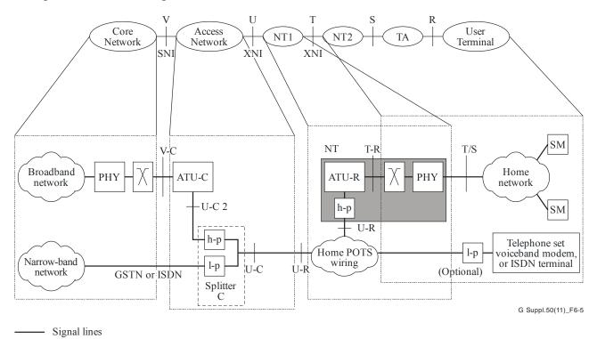
Figure 6-5 – ITU-T G.992.2 system reference model and its alignment with the generic reference configuration
