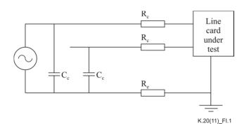
Coupling resistors,  $R_c$ , represent the line resistances; capacitances,  $C_c$ , represent the line capacitances to earth and  $R_e$  represents the earthing resistance of the overvoltage protectors at the subscriber end of the line.
