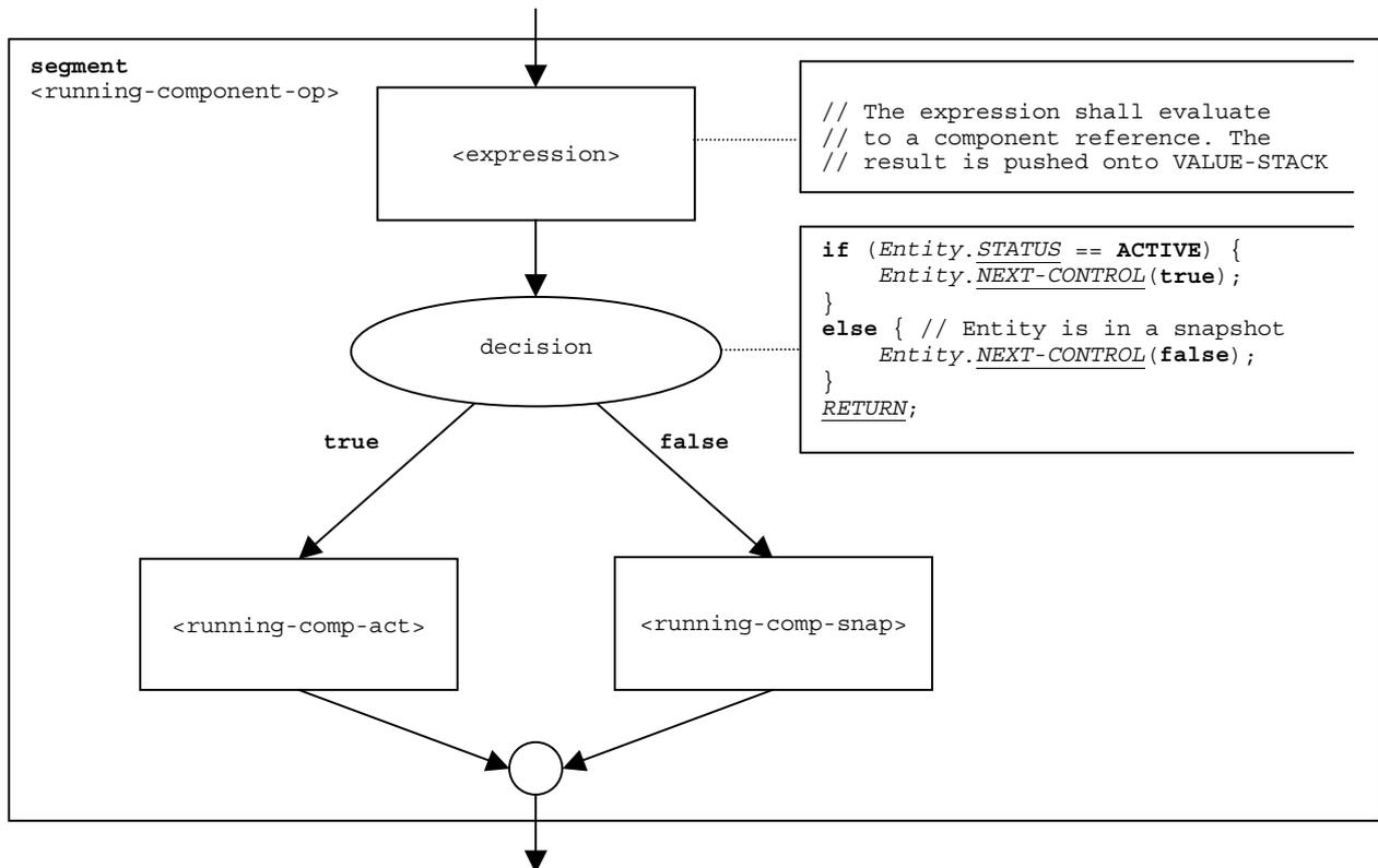
Figure 111 – Flow graph segment <running-component-op>
