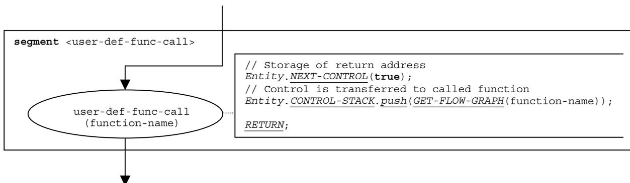
**Figure 84 – Flow graph segment  $\langle \text{user-def-func-call} \rangle$**
