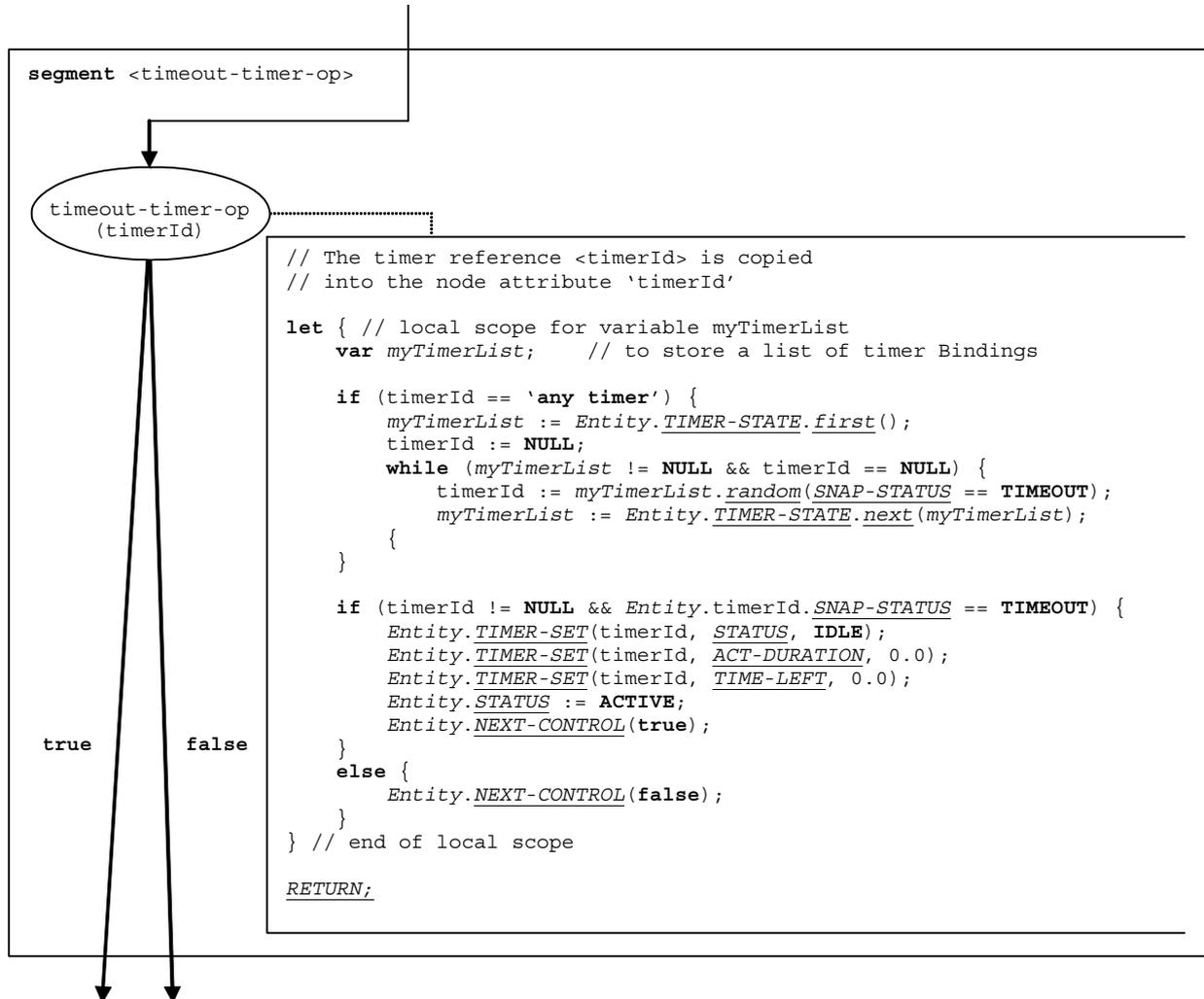
NOTE 1 – A `timeout` operation is embedded in an `alt` statement. Its evaluation is based on the actual snapshot, i.e., the decision is based on the `SNAP-STATUS` entry in the timer binding. If the timeout operation is successful, i.e., `SNAP-STATUS == TIMEOUT`, the timer is set into an `IDLE` state and the component state changes from `SNAPSHOT` to `ACTIVE`.
