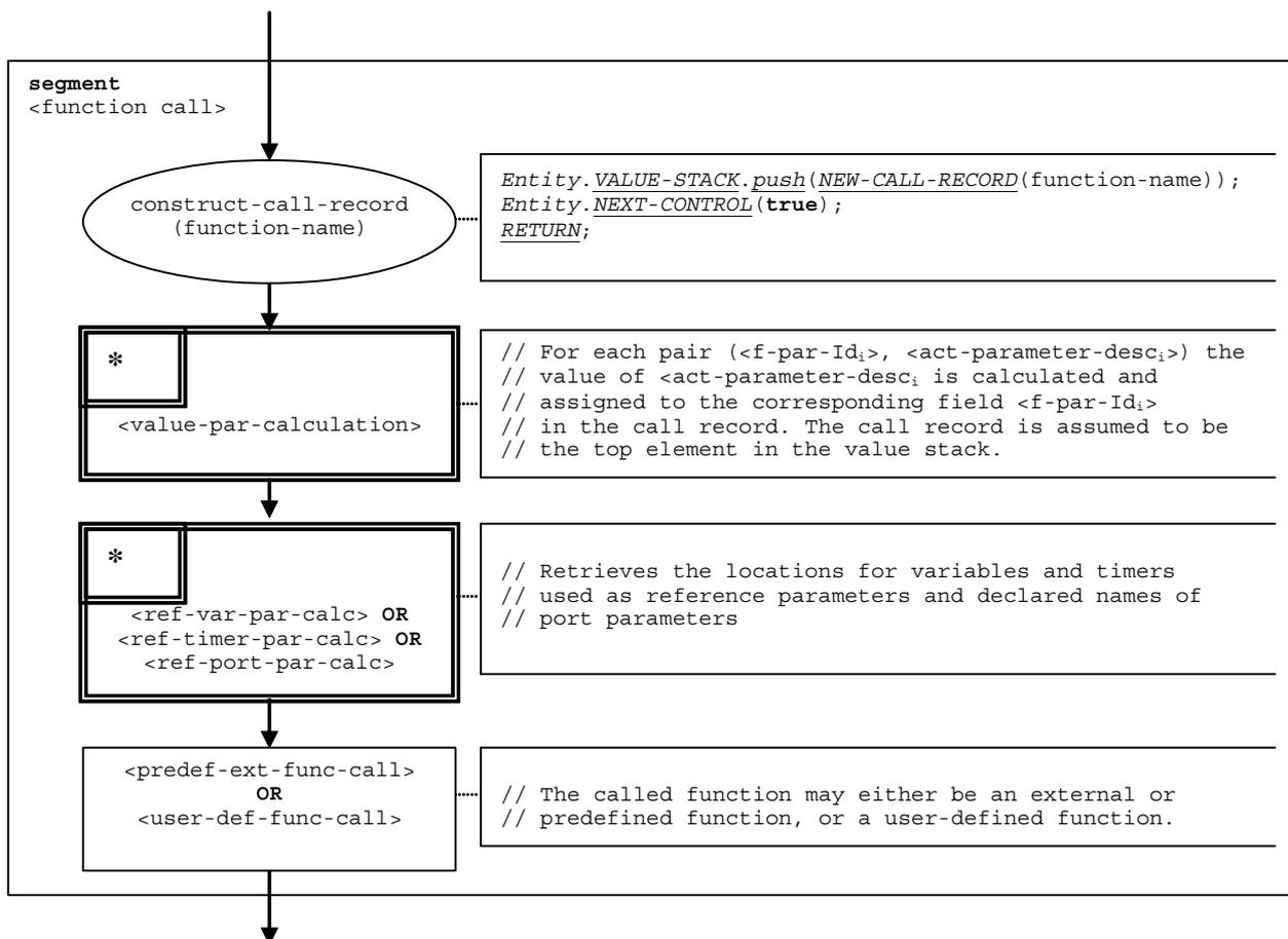
Figure 80 – Flow graph segment  $\langle \text{function-call} \rangle$
