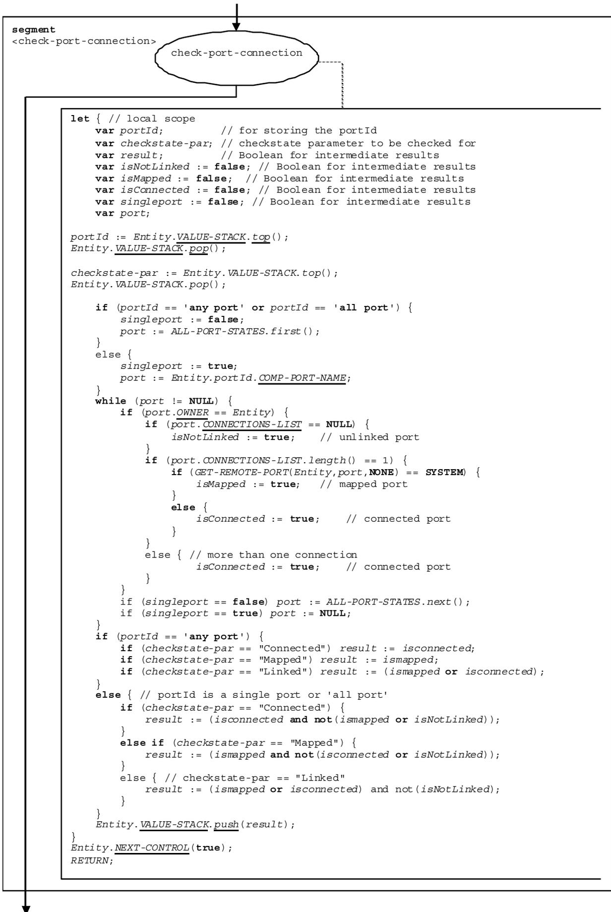
Figure 58c – Flow graph segment <check-port-connection>
