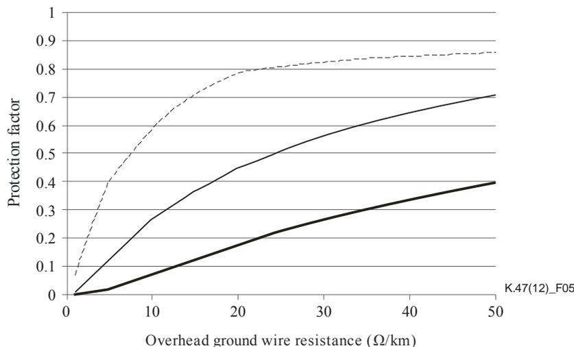
NOTE –  $U_b = 100$  kV;  $l_t = 50$  m; bold line:  $R_t = 10$  Ω; thin line:  $R_t = 30$  Ω; dashed line:  $R_t = 100$  Ω.
