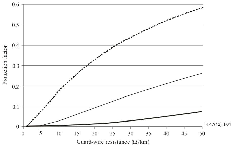
NOTE –  $U_b = 100$  kV; bold line:  $\rho = 100$   $\Omega\text{m}$ ; thin line:  $\rho = 300$   $\Omega\text{m}$ ; dashed line:  $\rho = 1000$   $\Omega\text{m}$ .
