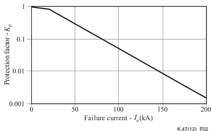
**Figure 2 – Protection factor ( $K_p$ ) as function of the failure current ( $I_a$ )**
