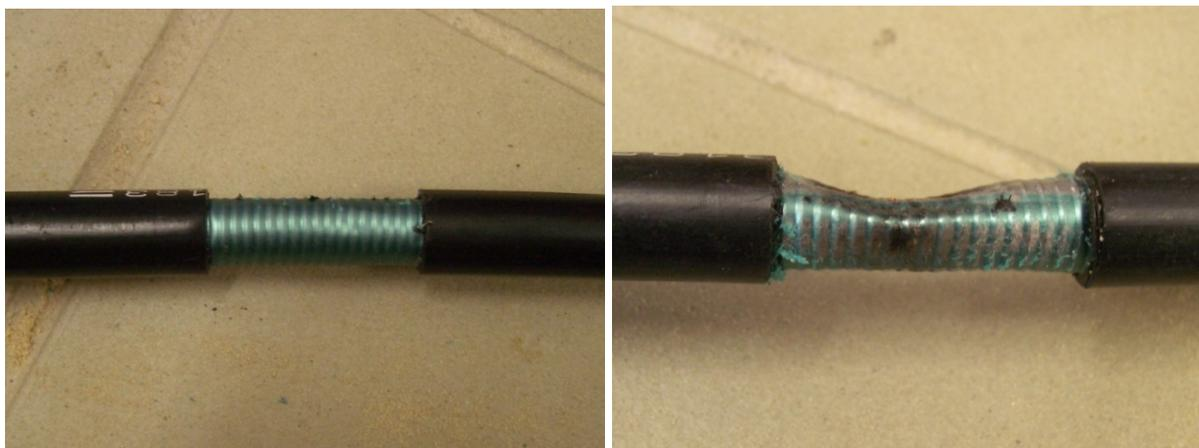
**Figure B.2 – Armoured optical fibre cable before and after the 55 kA sand-box test**
