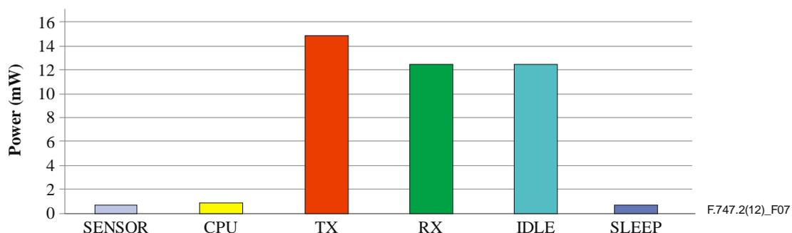
Figure 7 – Energy consumption for a typical sensor reported in [b-IEEE VTC]
