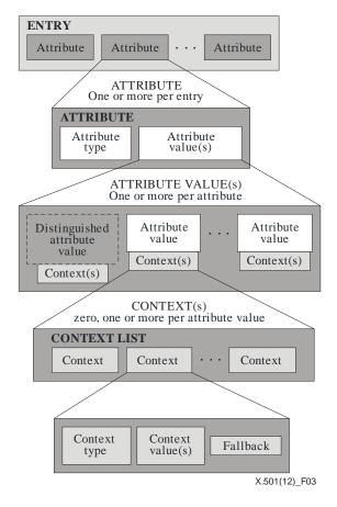
Figure 3 – Structure of an entry
