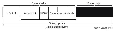
Figure K.1 – Response data structure on http-udp connection
