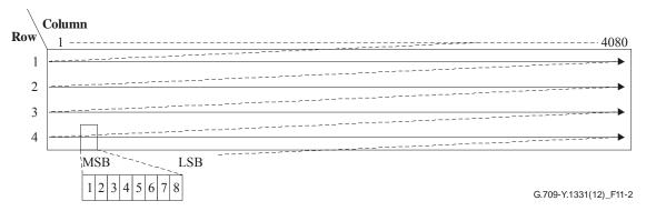
Figure G.2 – Transmission order of the OTU0LL frame bits
