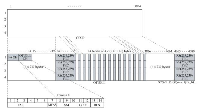
Figure G.1 – OTU0LL frame structure, overhead and ODU0 mapping
