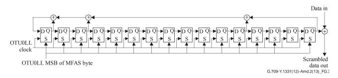
Figure G.3 – Frame synchronous scrambler
