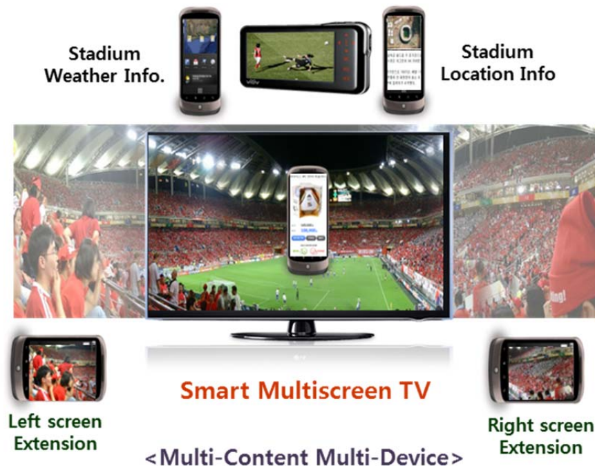
Figure 7-3 – Case III of the N-screen service: Collaboration among multiple devices
