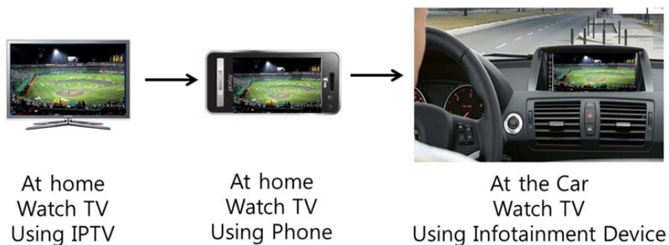
Figure 7-2 – Case II of the N-screen service: Handover or shift
